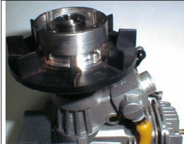
Attach the clutch to the fan hub using (2) M3x8 cap head screw.
