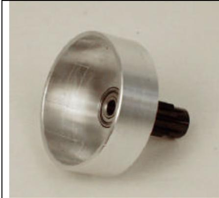
Score the clutch bell as shown. This provides better adhesion from the liner to the bell.
