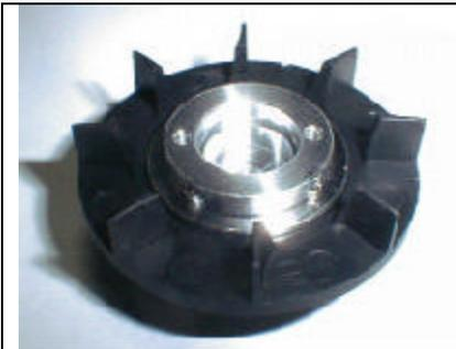
Attach the fan to the fan hub using (4) M3x6 flat head screws.
