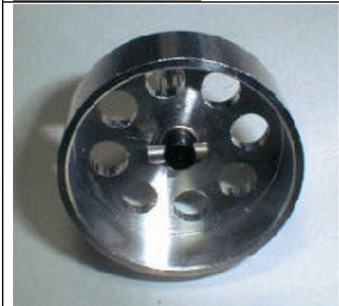
Slide the start shaft into the bell as shown to the left.
