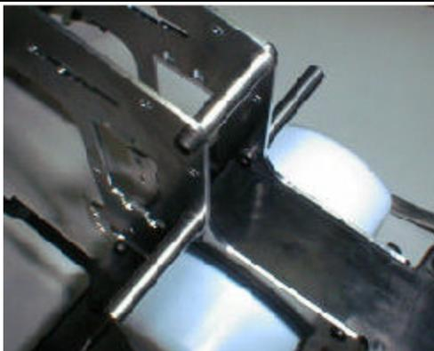
Install (1) 24mm cross member using (2) M3x6 cap head screws.
