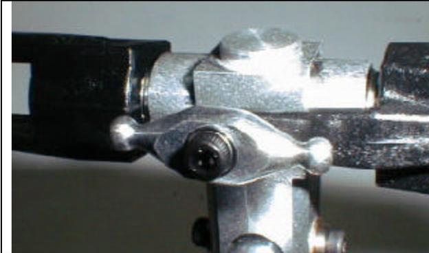
Attach each hiller arm to the blade grip using an M3x10 cap head screw. Put the bolt through the hiller arm and put a 3x5x1 spacer on the bolt next, and screw it into the blade grip.
