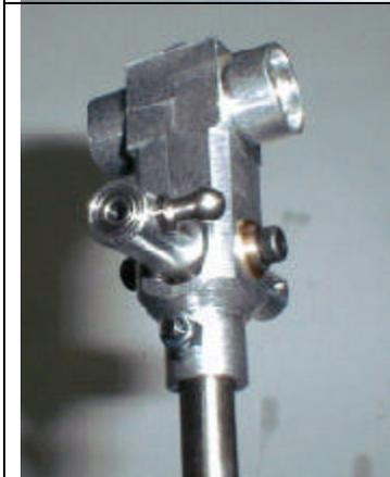
Locate (2) M3x6 pivot studs. Install the two pivot studs into the seesaw. They should be in holes opposite of each other. The other two holes tapped in the seesaw will be unused.
