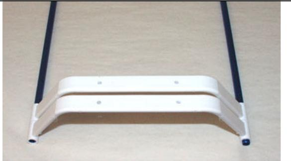
Attach the landing gear to the lower frame using (4) M3x14 cap head bolt. Secure the bolts using the (4) M3 locknuts.
