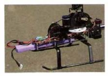
with a small file tip, I increased the length of the slots in the frames about 1mm farther forward to allow a proper gear mesh.
