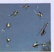
When I let the stick go back to center, the tail stopped immediately. After some moderate 3D flying, the average current draw was 32A, which should allow about 7 minutes of flight. Peak current was measured at 60 amps—right at the maximum limit of the TrueRC battery's rating.
