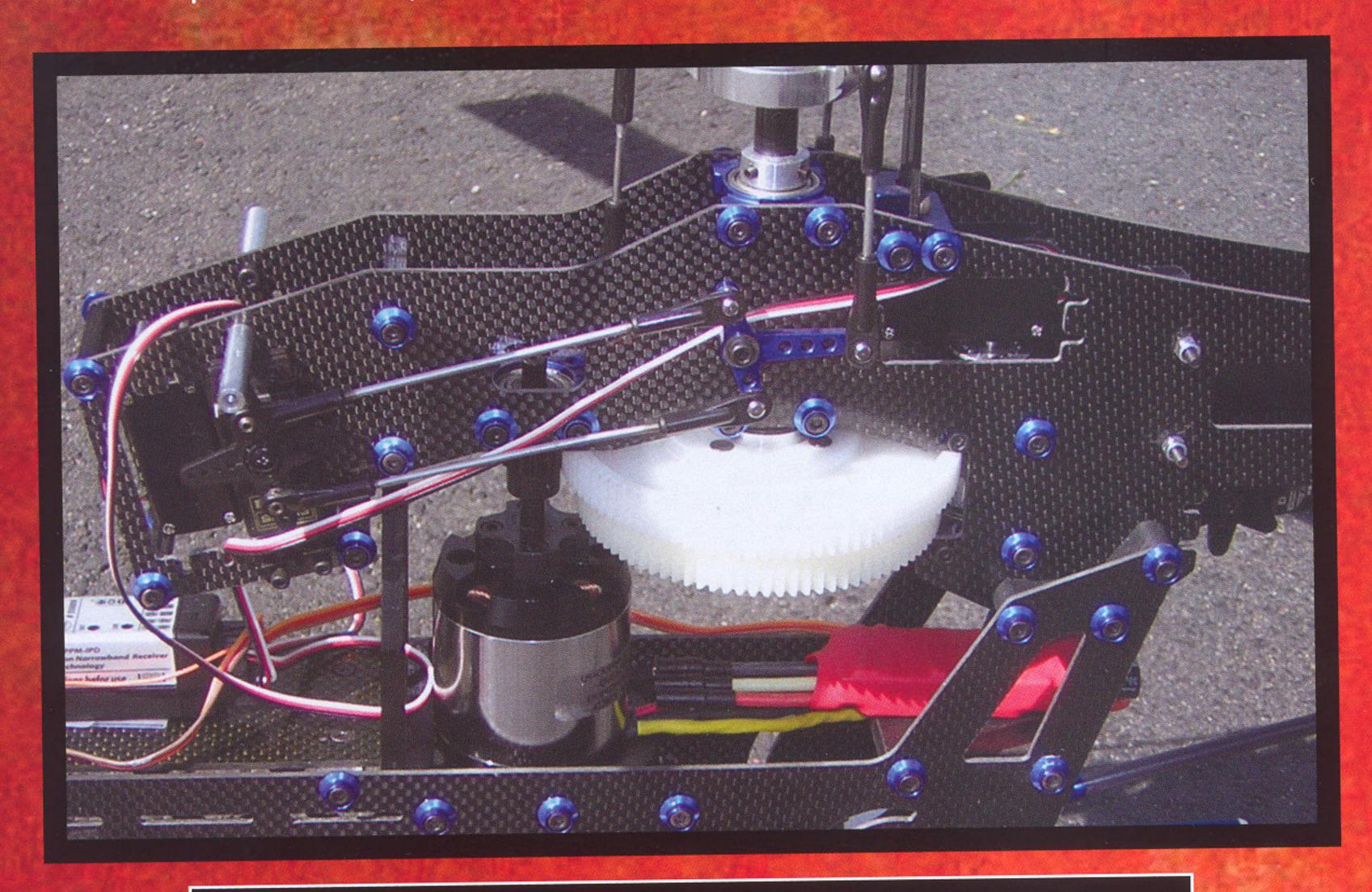
This model is powered by Quick World Wide's own Outrunner brushless motor and a 77-0 electronic speed controller.
