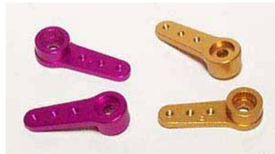
For all the Bat series helicopters you will need 3 full arms, short full arms, or wheels for the three collective servos. You will need either a half arm or a short half arm for the throttle and rudder.
