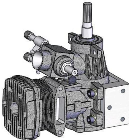
If you have the 70 or 90 helicopters you can follow these steps. They are basically the same as the 50 assembly, with some different hardware. Attach the motor mount using four M4x12 Cap Head Screws.
