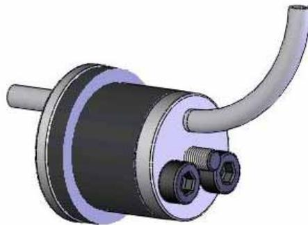
You will only need one line for fuel tank pressure so the other two holes in the stopper can be plugged off. This can be done with a few M3 bolts. When the stopper is tighten it will seal around the bolts.
