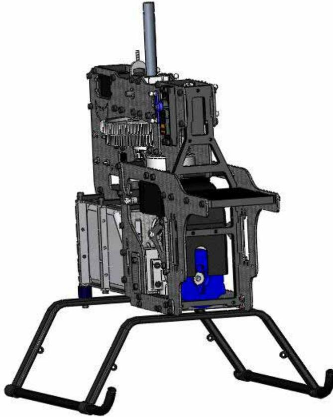
Attach the front landing gear mount to the landing gear mount using two M3x10 cap head screws. Epoxy in the skid tube ends.
