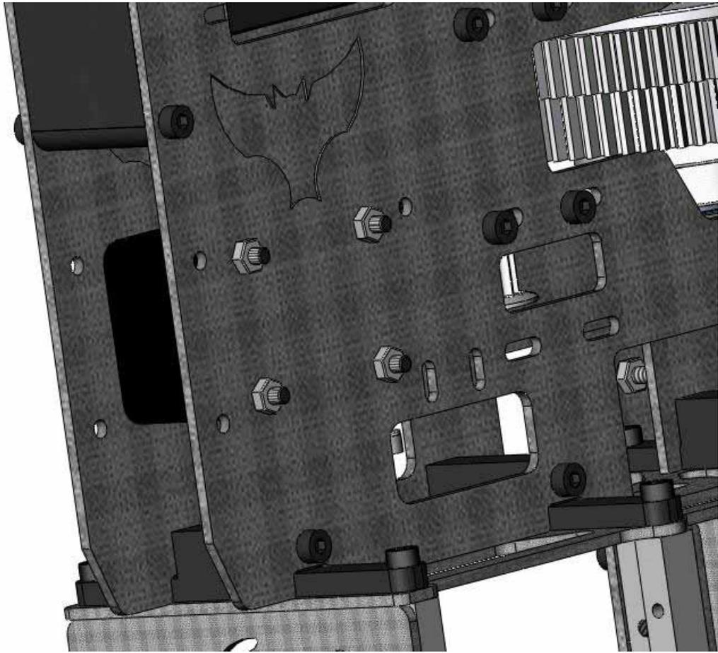
Now you can install the plastic boom holder blocks. Install the blocks with four M3x35 cap head screws and lock nuts.
