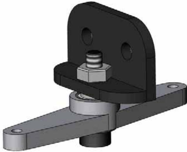
Locate your rudder bell crank mount and attach the Bell crank assembly with an M3 Locknut.
