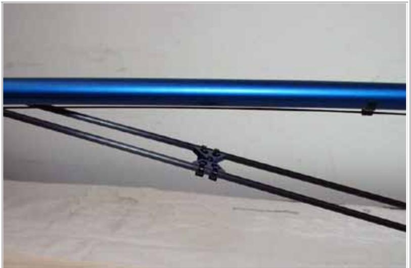
**Skid Stops** - The skid stops slide over top of the skids and cushion your landings a bit. They also prevent scratching if you hover over top of concrete or asphalt.
