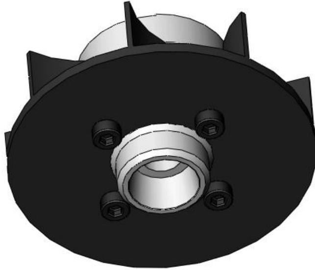
Attach the fan to the fan hub using four M3x8 cap head screws.
