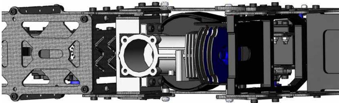
The next step is to install the motor assembly into the helicopter. There is a 3mm spacer on either side of the motor mount. You can CA or silicone these into place to make it a bit easier to get everything to line up when installing the motor.
