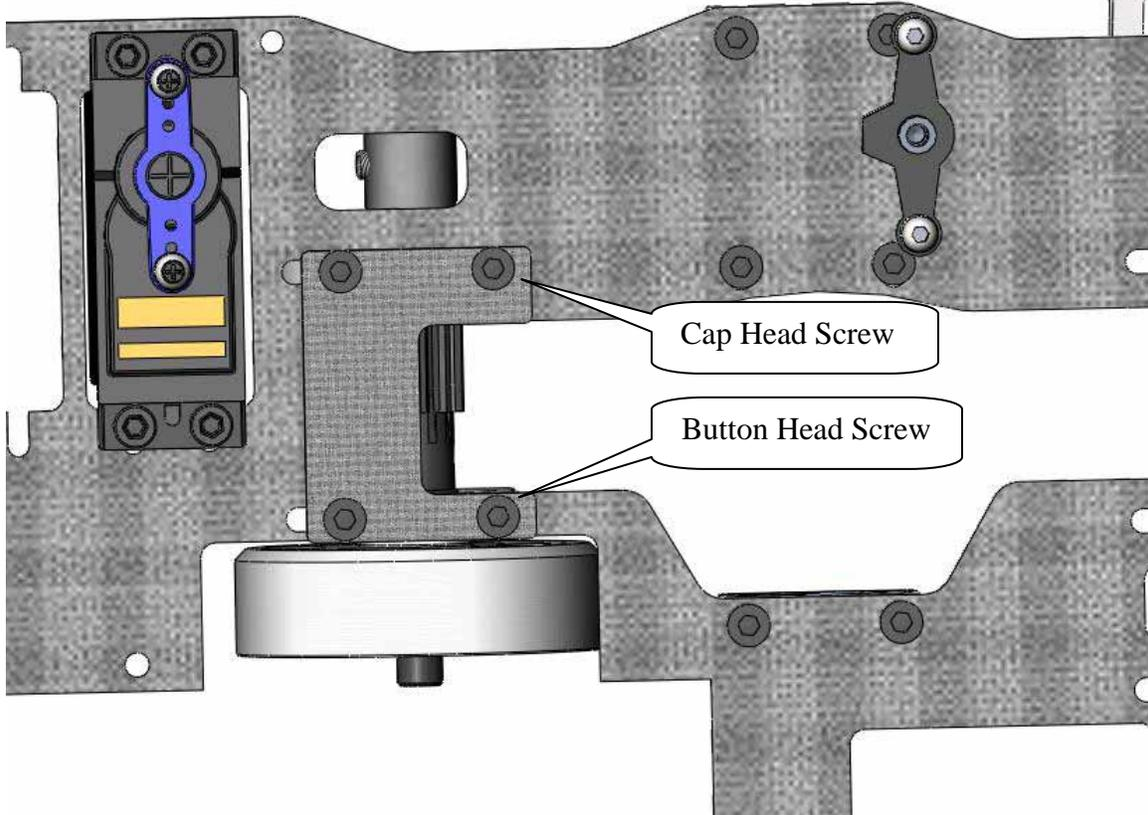
Now, attach your clutch bell assembly to the main frame. You will need (2) M3x10 SOCKET HEAD CAP SCREW, (2) M3x10 button head screws, and one of the doubler plates. Use two of the M3x10s in the upper holes and the two BUTTON HEAD CAP SCREWS in the lower holes. You can leave this sort of loose for now. It will need to be adjusted later when the main gear is installed for proper gear mesh.
