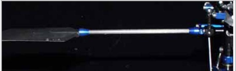
**Throttle Extension** - The throttle extension makes the setup of the throttle very easy. It clamps onto the throttle barrel of the carburetor and help produce linear throttle curves.
