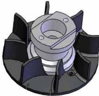
Locate your fan hub and fan. The fan fits over the fan hub from the top as it is pictured here.
