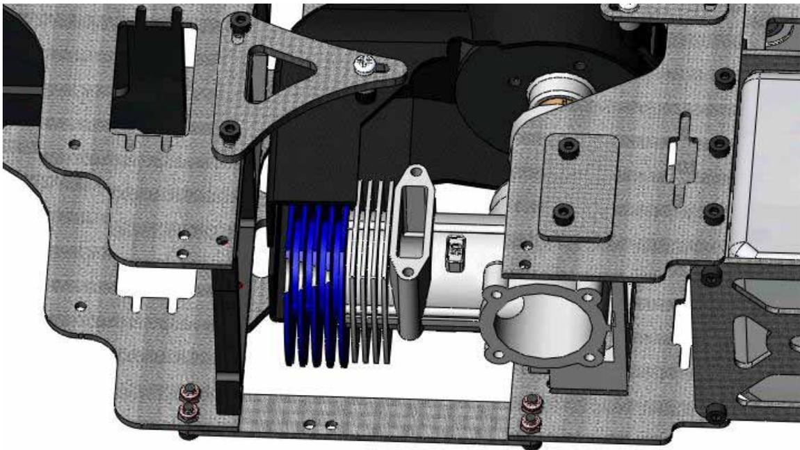
Attach the landing gear mounting plate to the engine frame with five M3x8 cap head screws and four lock nuts.
