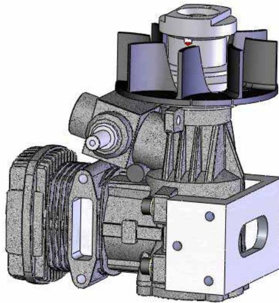
Slide your fan hub onto your crank shaft and secure it in place with the prop nut that came with the engine.
