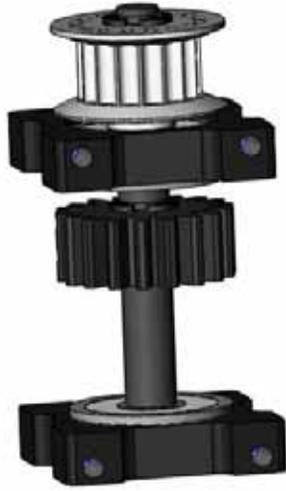
Now you can slide on the pulley gear and secure it with the M4 E-clip.
