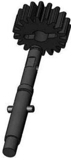
Slide counter gear lock pin into the counter gear shaft. Then slide the counter gear down the shaft and capture the pin in the groove
