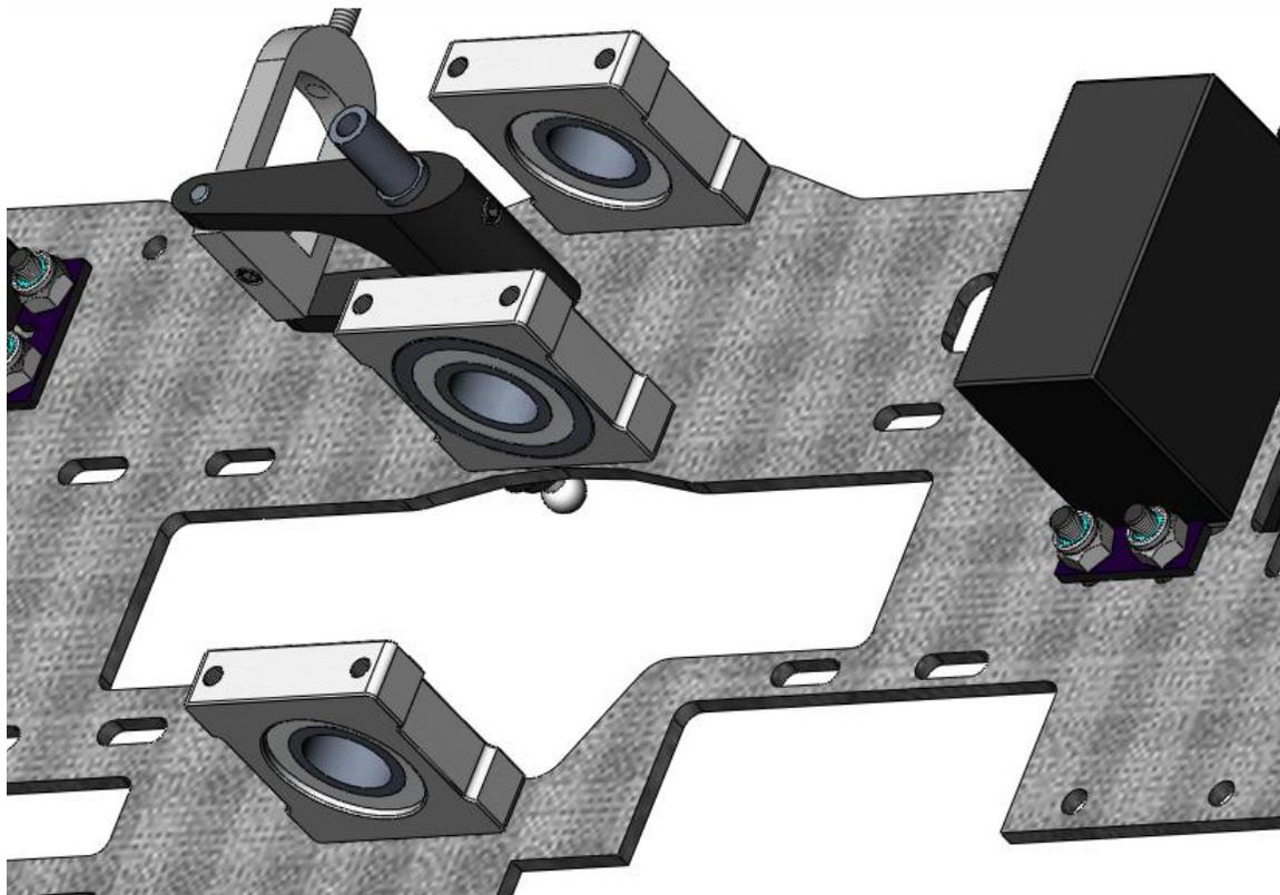
Attach the three main shaft bearing blocks to the upper frame. Be sure that the flanges for the two upper main shaft bearing blocks face each other. By flange, we mean the side of the bearing block
