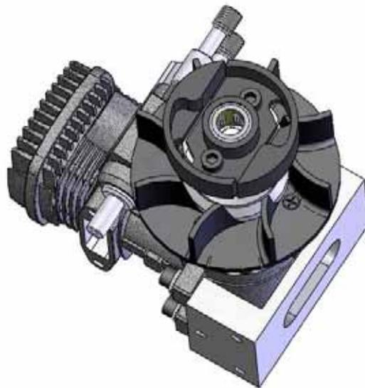
Next, attach the clutch shoe to the fan hub.
