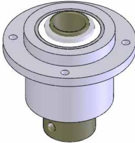
Locate your auto rotation sleeve and spacer. You will slide your auto rotation sleeve into your hub and slide the spacer on the top. You can leave the spacer off until you are ready to install the unit into the helicopter.
