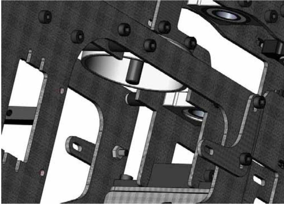
Next we will attach our rear fan shroud mounts. For the upper hole we will use an M3x25 cap head screw. Remove the M3x8 cap head screw in the lower main shaft bearing block. Install the new screw through the fan shroud mount, then through the engine frame, then through an 18mm spacer, and finally into the bearing block. You can leave this sort of loose for now, until the fan shroud is installed and adjusted. The lower screw is an M3x8 cap head screw and a lock nut.
