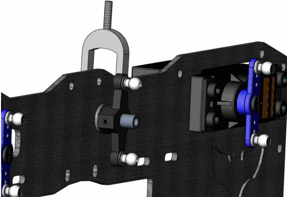
Install the elevator assembly into the bearing in the upper frame assembly and attach the outer elevator arm with an M3x5 set screw. Install two M3x4 pivot balls into the elevator arm.
