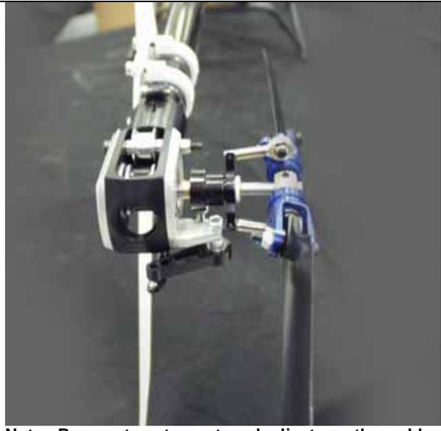
**Note:** Be sure to set your travel adjusts on the rudder to avoid the tail pitch slider from contacting the tail pitch lever mount. If your gyro does not have this function, put a little piece of fuel tubing on the shaft to make a rubber stopper.
