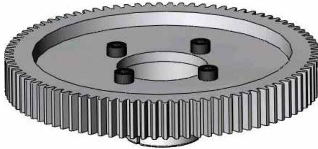
Attach the lower main gear to the lower main gear hub using (4) M3x12 cap head screws.
