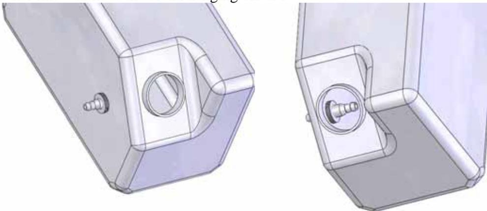
The alternate way of doing your fuel system is to add a fuel nozzle on the size of the tank.
