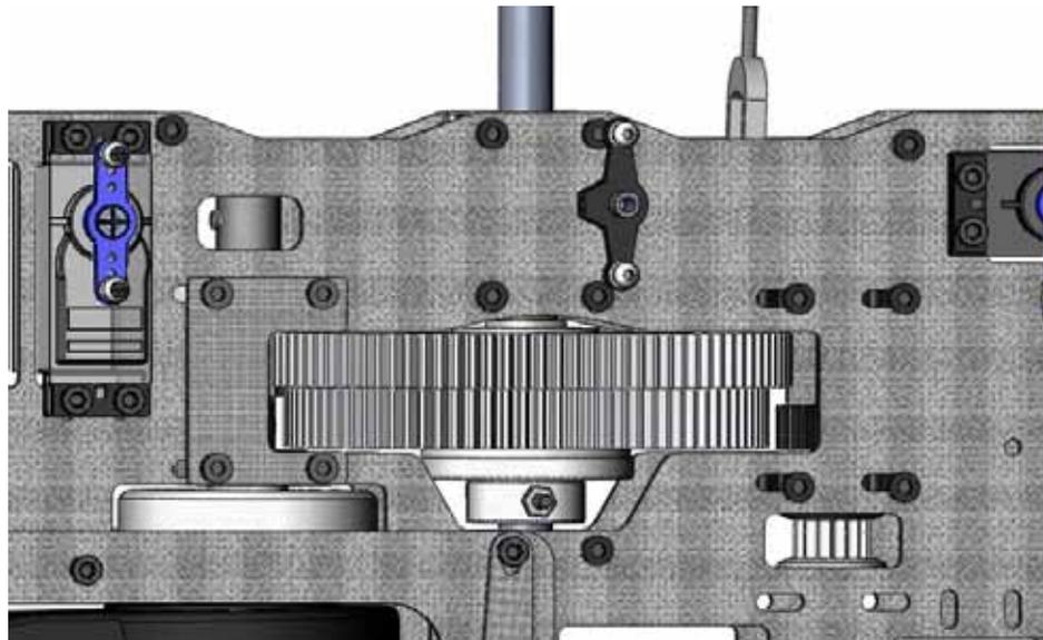
The lower main shaft bearing is vertically slotted so that you can adjust the height of the main gear to get the positioning perfect.
