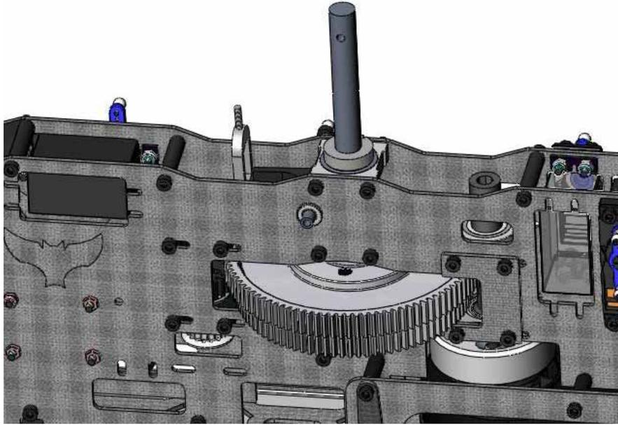
Slide the main shaft collar onto the main shaft. While pulling up on the main shaft to remove any play and tighten the collar with the supplied M2.5x8 cap head screw.
