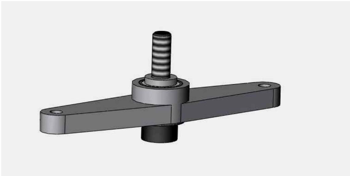
Insert an M3x14 cap head screw as shown. Slide a 3x5x3 spacer onto the screw,
