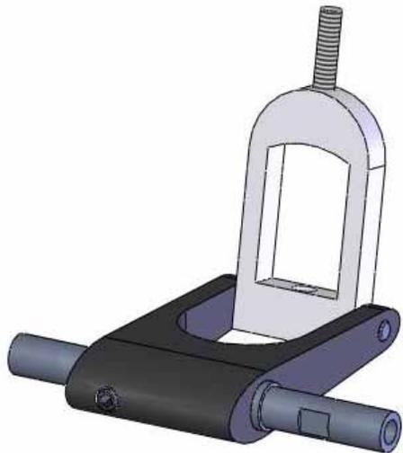
Attach the unit to the elevator control shaft using an M3x5 set screw. Be careful to install the shaft so the flat for the elevator bell crank comes out the same side you have your servo on. In our case we have is on the left side.
