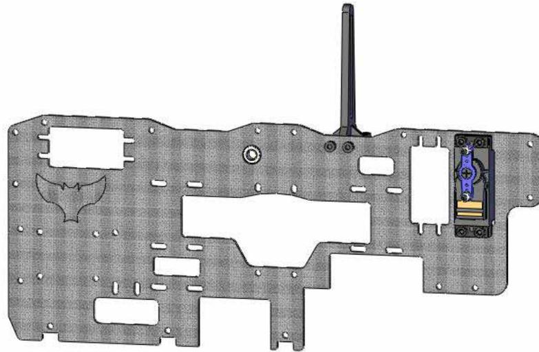
This step is only for the budget series helicopters. Install the Swashplate anti-rotation guide to the main frame using 2 M3x8 cap head bolts. You will install two on the opposite side when the other frame half is attached.
