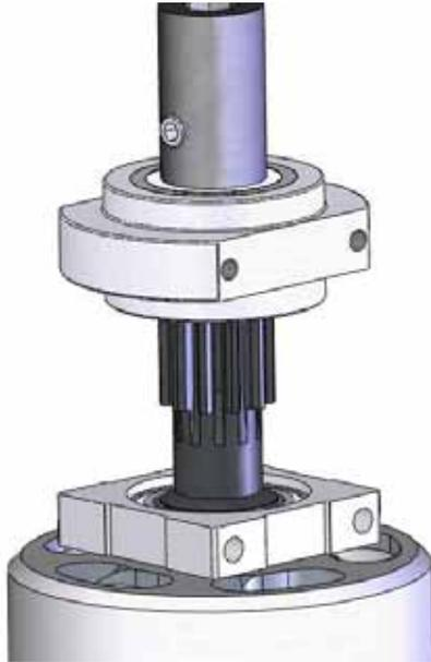
With the start shaft pushed all the way into the clutch bell attach the start coupler with an M4x4 set screw. When assembling this for the 70 or 90 clutch bells, you will use three 5x7x2 spacers between the clutch bell bearing block and the start coupler.
