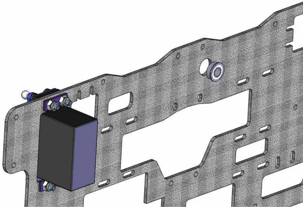
Note: The holes on the frames are designed for “push-fit” feature. Sometime you may have to use a round “rat tail file” before pushing the bearings in. The bearing flange mates against the inside of the frame. The flange is set on the inside of the frames. The elevator shaft will hold the bearing in place.
