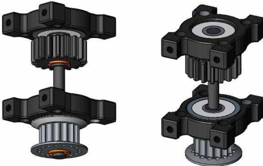
If you are building the budget series of bat helicopters, your counter gear assembly will look like this. It is assembled the same way as the regular bat counter gear assembly except that this one will work off the top gear for the budget bat auto hub.
