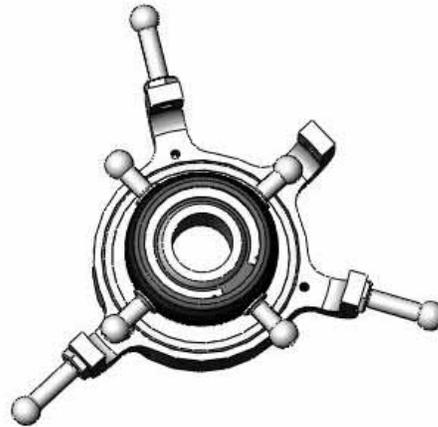
There are 3 M2 holes tapped in the lower ring of the Swashplate install the M2x4 Phillips head screws there. The lower outer ring of the Swashplate will get the M3x12 pivot balls, and the inner ring will get the M3x7 pivot balls. On the budget series bat you will add a straight pin to the 4<sup>th</sup> open position on the outer ring of the Swashplate.
