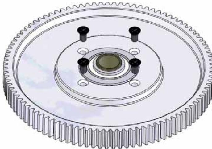
Attach the upper 97T main gear to the auto rotation hub using (4) M3x6 flat head screws. When you install the screws on both gears, tighten the screws in a cross wise fashion to get equal pressure on the gear and ensure that the gears sit flush onto their hubs.
