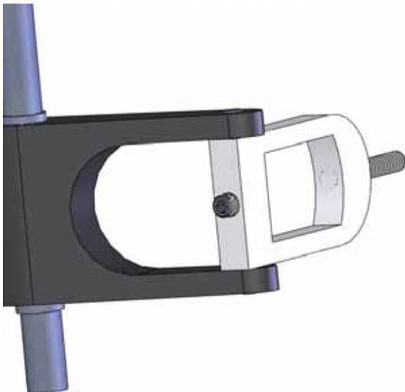
Install an M3x5 set screw into the bottom of the elevator control unit to secure the pin.
