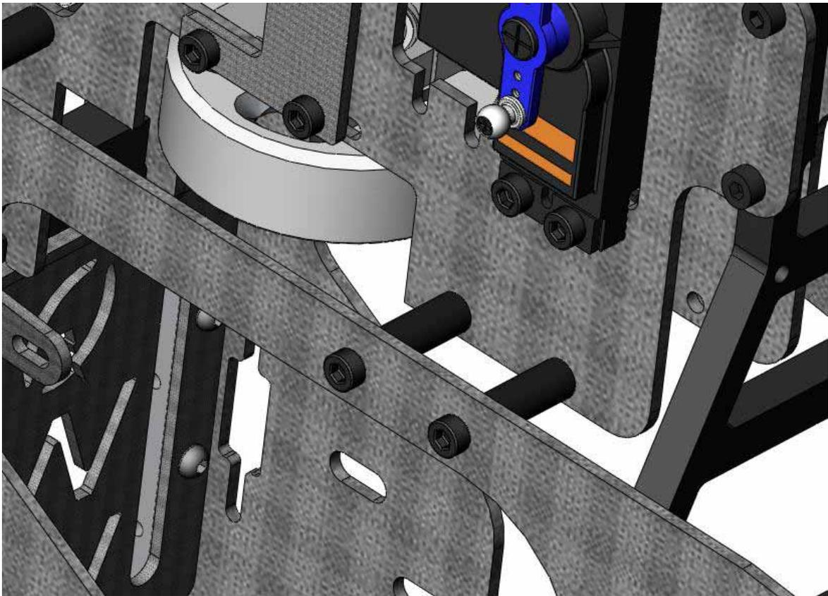
Now we can install the two frame cross members. First, gather four M3x25 cap head screws and four 18mm frame spacers. Slide the bolt through the frame slide an 18mm spacer onto the bolt and slide the bolt through the hole in the main frame assembly.
