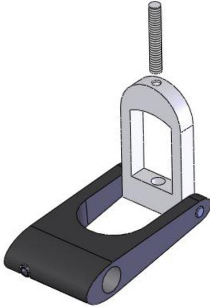
Install the M2.5 set Screw into the elevator control unit
