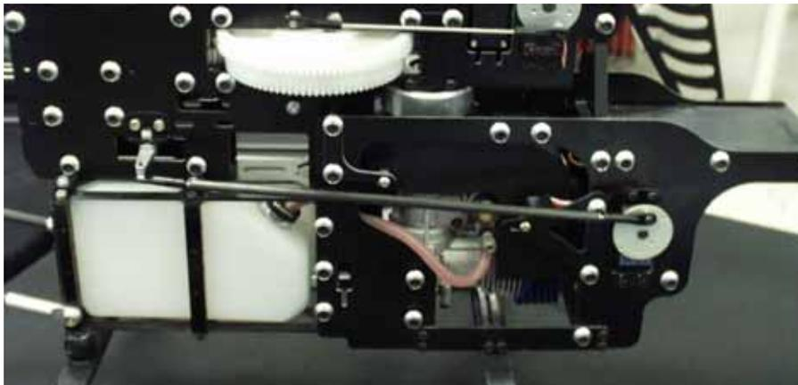
For the 50 sized helicopters you will need a carbon rod cut to 200mm. Glue in the ends, and thread on a long ball end on each end. The ending rod should be ~250mm from ball to ball. You simply want to have your servo at straight up and down at neutral and then have the bell crank in the rear perpendicular to the side frame.
