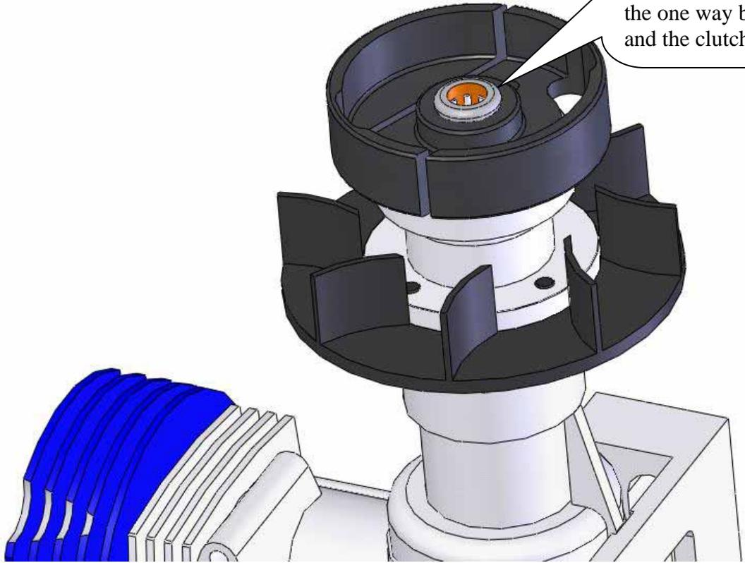
Attach the clutch shoe to the fan hub using two M3x8 cap head screws.
