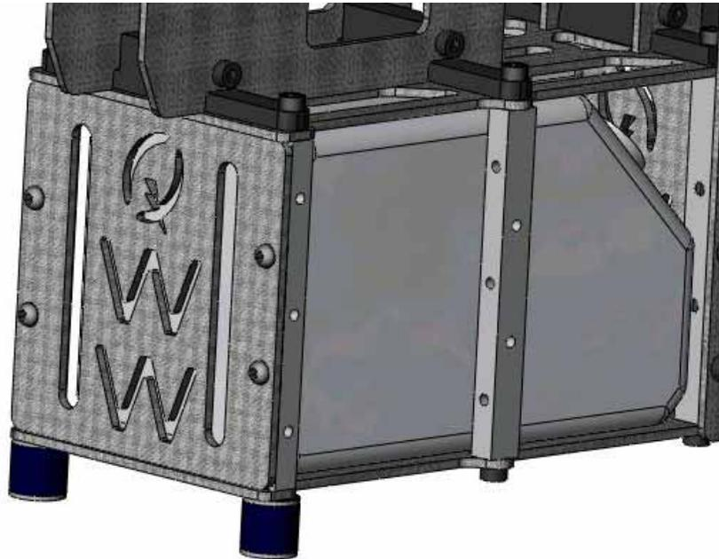
Attach two landing gear dampeners to the fuel tank assembly. Find two M3x12 set screws and install them into the landing gear dampeners using Loctite. Next, thread them into the rear fuel tank cross members.
