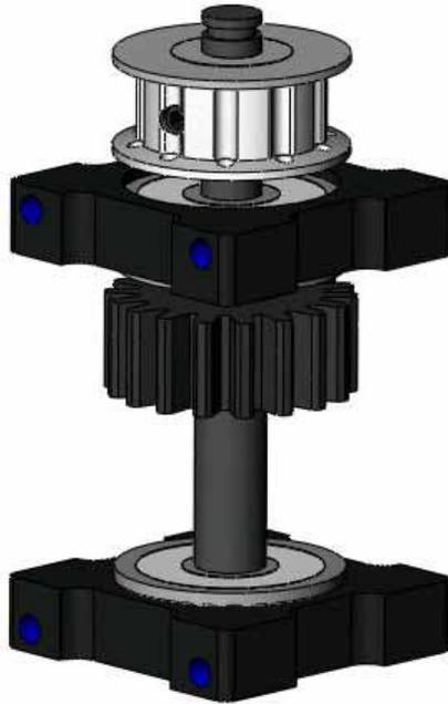
If you are building a 70 or 90 helicopter, you will have a pulley like this for the coarse belt. It is simply secured in place with an M3x5 set screw onto the flat on the shaft.
