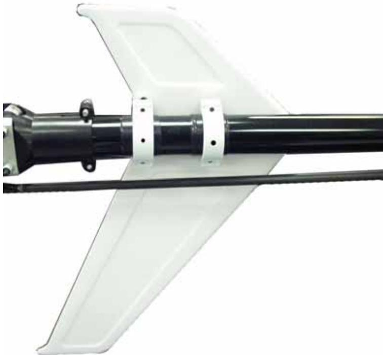
It is a good idea after you mount your fin onto the helicopter to add a small hole to each fin mount and insert a small self tapping screw to ensure the fin cannot twist and get into the tail rotor assembly.
