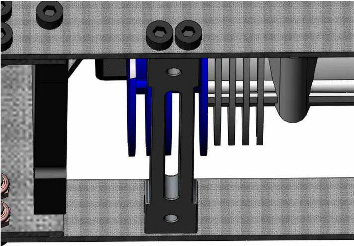
Attach the landing gear mount with four M3x8 cap head screws.
