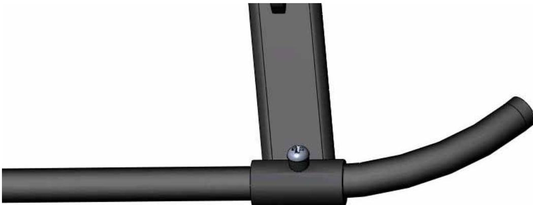
Secure the landing gear skids with (4) M2.5x6 self tapping screws.
