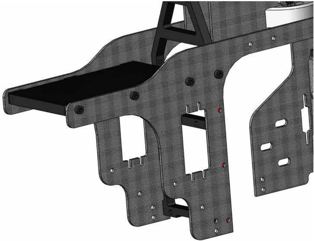
Now we will attach the radio tray. There are 3 M3x8 cap head screws needed for each side.
