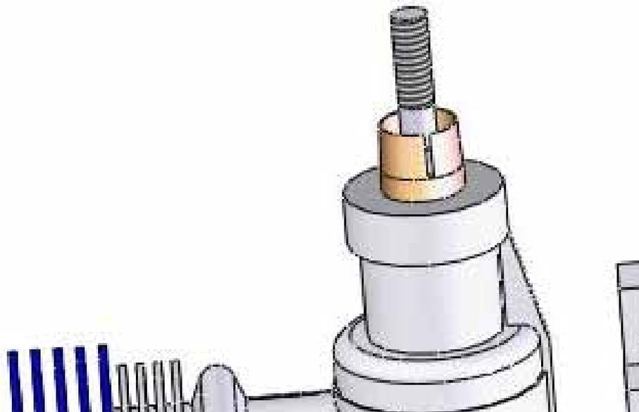
Next, install the engine collets. First is the one that just looks like a spacer/washer. Then the larger conical collet goes on.
