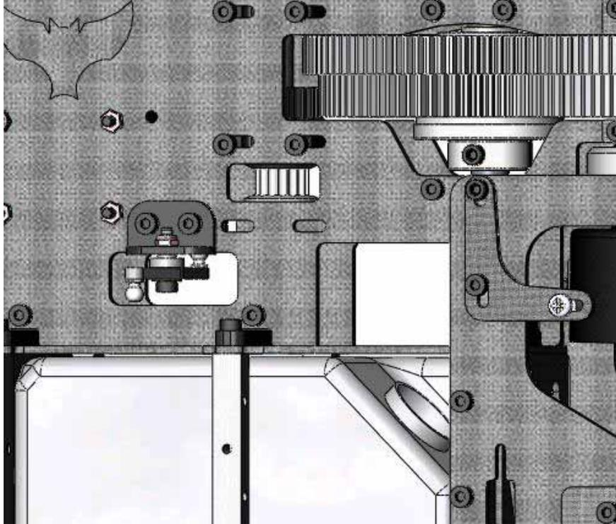
Next, attach the completed assembly to the helicopter with two M3x10 cap head screws and M3 lock nuts. The bat 50 uses the rudder bell crank on the right hand side as if you were sitting in the helicopter. The 70 and 90 Bats go onto the opposite side. This is due to how the fan shroud gets mounted in the helicopters.
