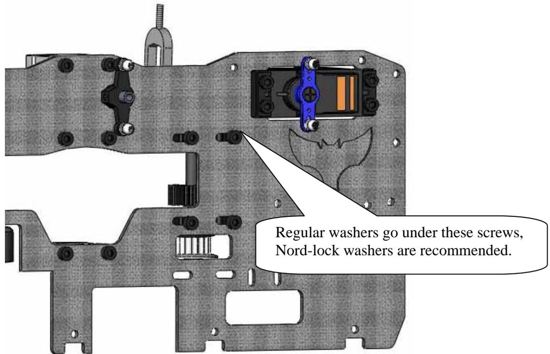
Now attach your counter gear assembly using (4) HHI3M08C (3 X 8mm SOCKET HEAD CAP SCREW) screws. Leave this slightly loose until you are ready to adjust gear mesh. Included are 4 M3 washers to use on the slots. It is recommended that you upgrade these to M3 Nord-lock washers to prevent any bearing block movement than can result in the main gear stripping out.
