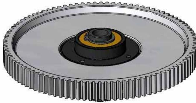
This is how it will end up looking from the top side. You will Slide the main shaft into the auto rotation hub in the same way as detailed earlier. Attach the autorotation hub to the main shaft using an M3x16 cap head screw and M3 Locknut.
