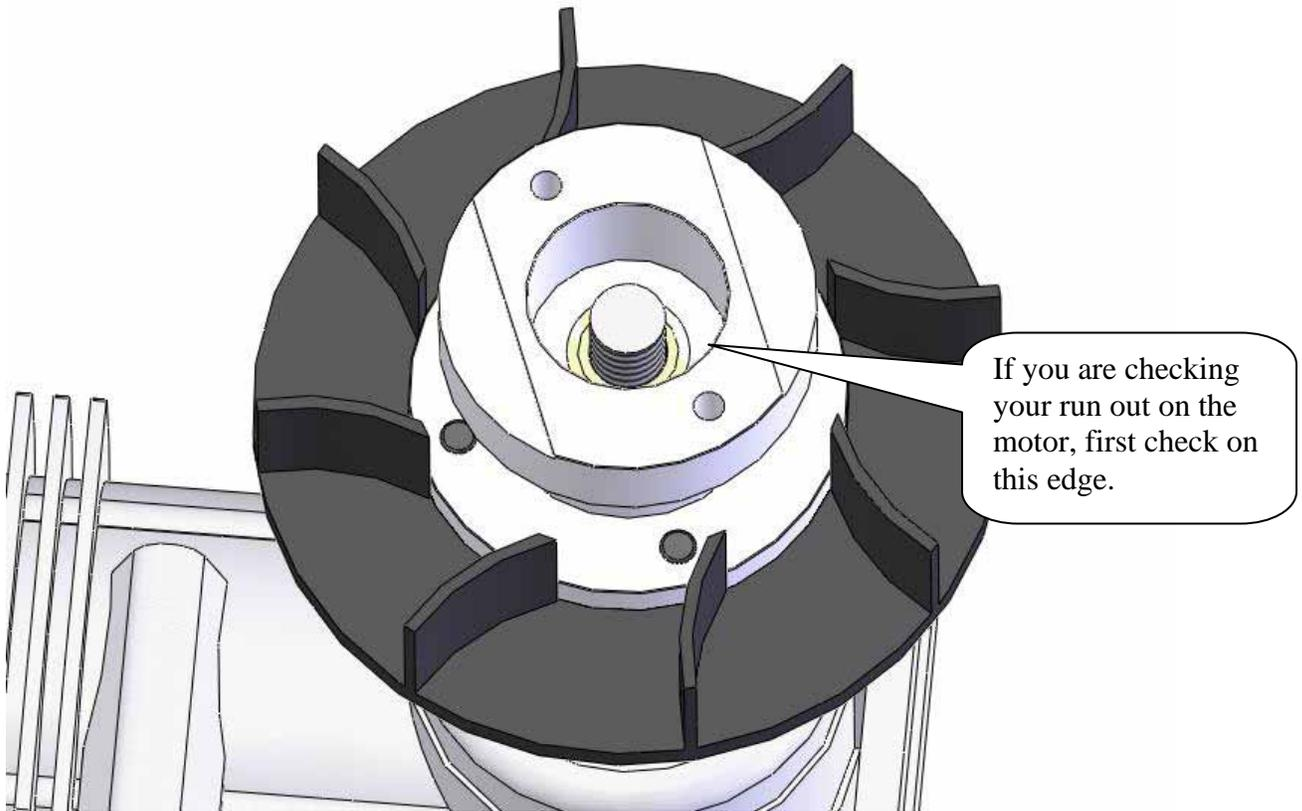
Slide the second smaller conical collet down onto the crank shaft. The tapered side goes down into the cavity. Secure the fan hub with the prop nut that is included with the motor. Note: It is important to use a Dial Indicator to check the run out of the Engine Assembly. Most of the vibration problems come from this. The run out should be no more than 0.004 inch (0.10 mm).
