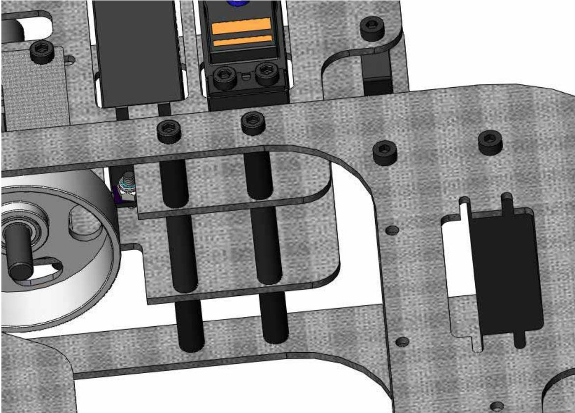
Locate two 26mm cross members. Remember to Loctite all screws and screw the outer spacers into the inserted 26mm cross members in the frame.
