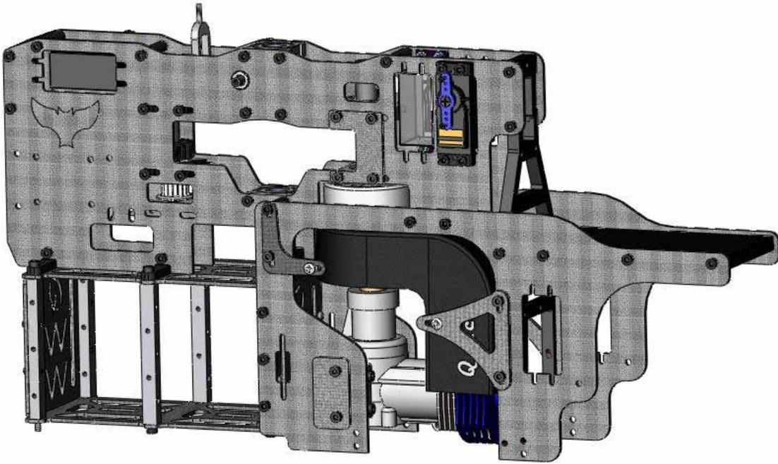
Secure the motor in the helicopter using four M3x12 cap head screws. There is a motor mount double plate provided for the outside of the frame as well.
