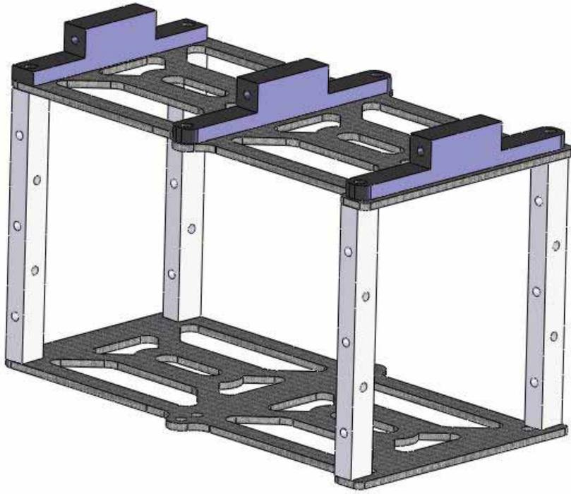
Assemble the fuel tank assembly as shown. You will have one shorter upper to lower mounting block and two longer ones. The longer ones go on the two rear sets of holes.
