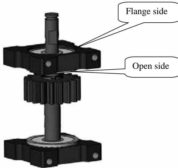
Next, install the two counter gear bearing blocks. Be sure that the flange face the top on the upper block and down on the lower block.
