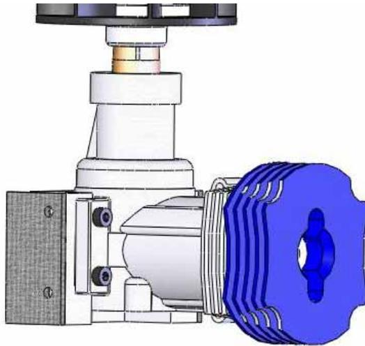
Attach the motor mount to the motor using four M3x10 cap head screws. Using Nord-lock washers are a nice accessory to use here. The motor mount is not symmetric. The end that has the further distance to the end from the screw hole will down as shown in the picture.
