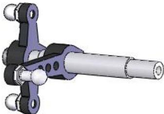
If you are building a budget series bat helicopter you will be using this style of elevator lever. You will assemble it onto the elevator shaft the same way as the other style with an M3x5 set screw. Install an M3x7 pivot ball stud into the arm.
