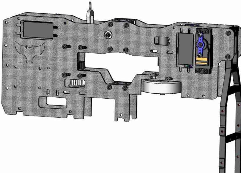
Now attach the two frame halves together. Use (4) M3x8 cap head screws to attach at the Counter gear assembly. Use (6) M3x8 cap head screws for attaching the main shaft bearing blocks. Locate your 2<sup>nd</sup> clutch bell bearing block doubler. Use (2) M3x10 socket head cap screws to attach the upper bearing block on the clutch bell assembly to the main frame. Use (2) M3x10 button head screws to attach the clutch bell assembly's lower bearing block.
