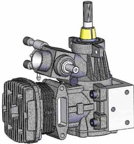
Slide the Collet onto the shaft.
