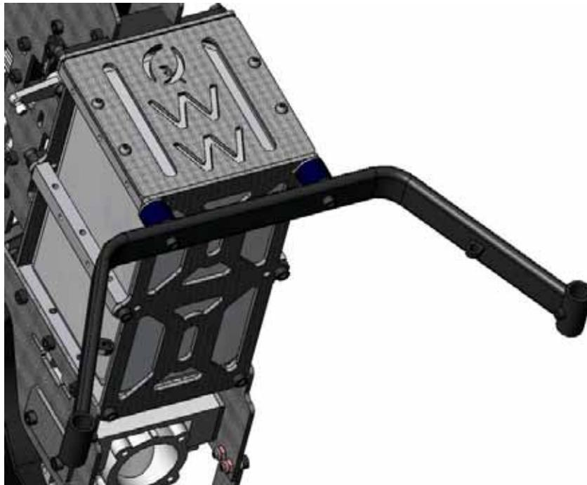
Attach the landing gear to the dampeners as shown. Use two M3x10 cap head screws. You will need to drill two M3 or 1/8" holes in the plastic to mount the landing gear. It is 70mm from hole to hole on the rear landing gear and 60 on the front one. **TIP:** One method for aligning the holes properly is to take a piece of masking tape and put it on the mount for the helicopter. Mark the holes with a magic marker or pen and then transfer the tape to the landing gear and drill the holes.
