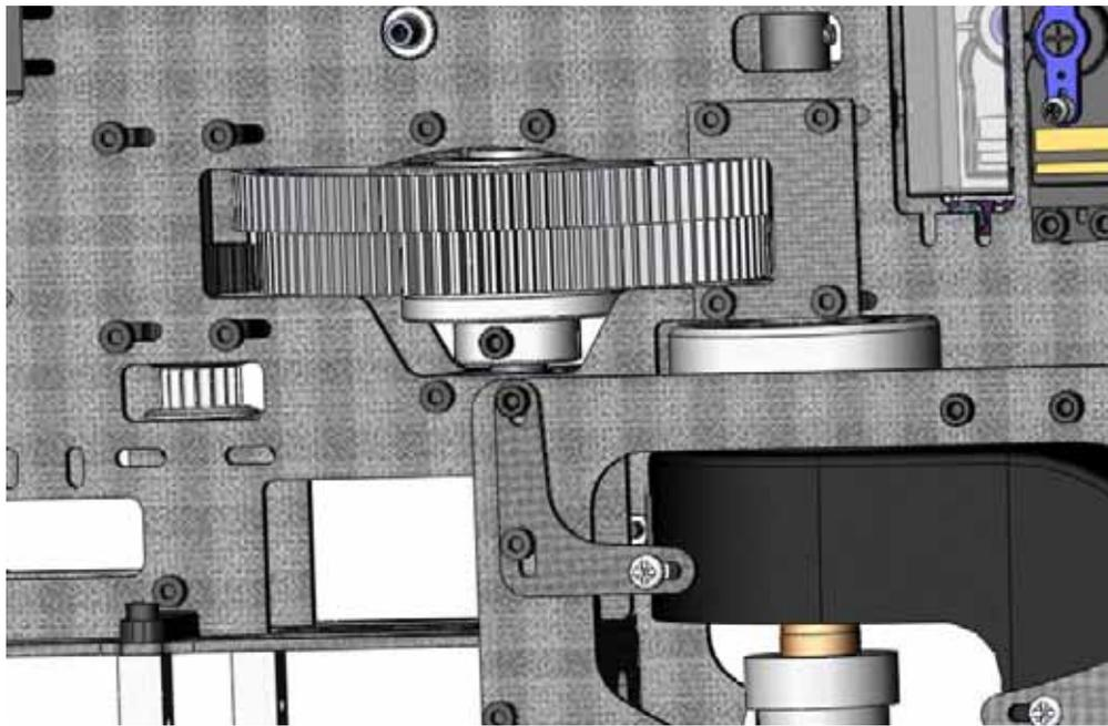
Next, you will slide your main shaft through the main gear hub assembly. The end with the longer distance to the hole goes in first. It will be the end going in first. Attach the main gear assembly using an M3x30 cap head screw and an M3 Locknut.
