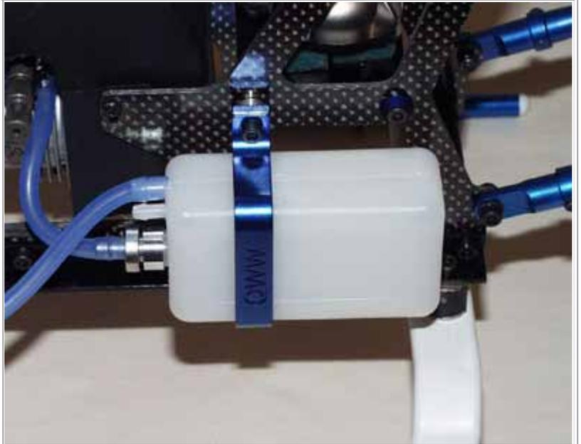
**Fuel Filter (QUI9002)**- A fuel filter is required because of the dirt and dust that can get into your fuel at the field.
