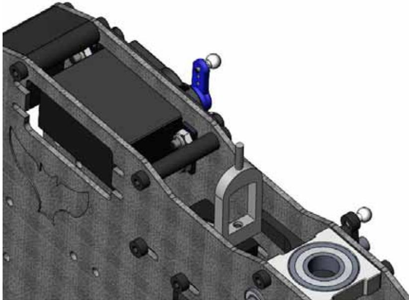
Install the upper frame cross member with two M3x8 cap head screws.
