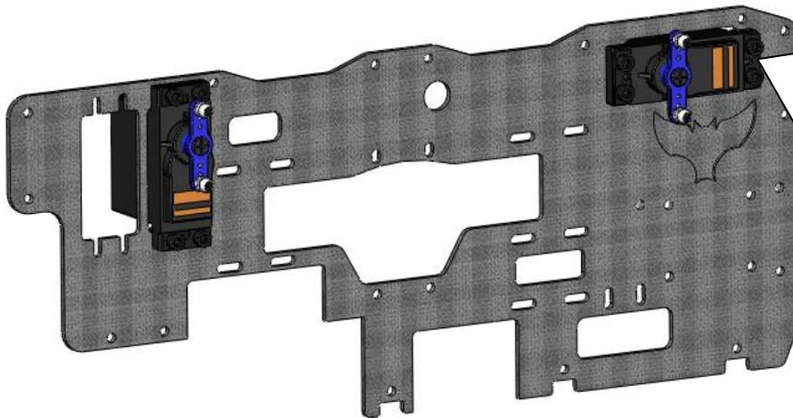
Depending on your servo type you may get better servo rod angles by mounting the servo on the inside of the frame. Shown here is with the servo on the outside. You want to have the rods as straight as possible.
