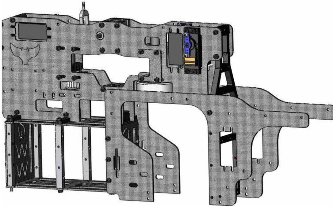
Now, attach the second engine frame piece. You will use four M3x8 screws just like the previous step.
