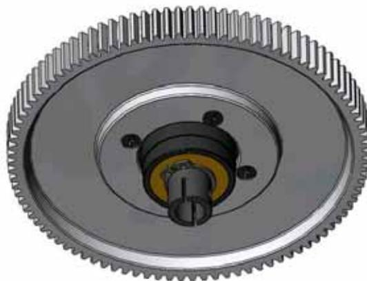
If you are building a budget bat you will have an autorotation assembly that will look like this. The gear slides up from the bottom and attached with (4) M3x6 Flat Head Screws.
