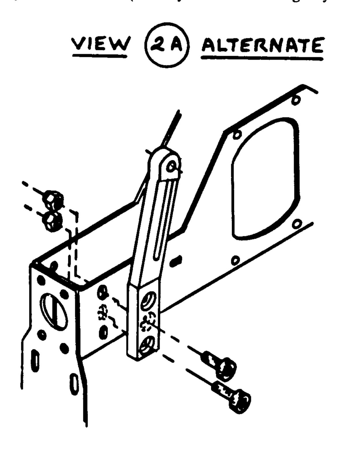
A. Select a 2mm Control Ball Spacer, #0697, and, using poly-zap cyano only, glue in place in the radius arm #0247. Slide a steel ball #0361 onto the #0042 (M2x10) slotted screw. Using slow cyano, thread the screw/ball assembly into the previously glue spacer #0697. Tighten completely.
