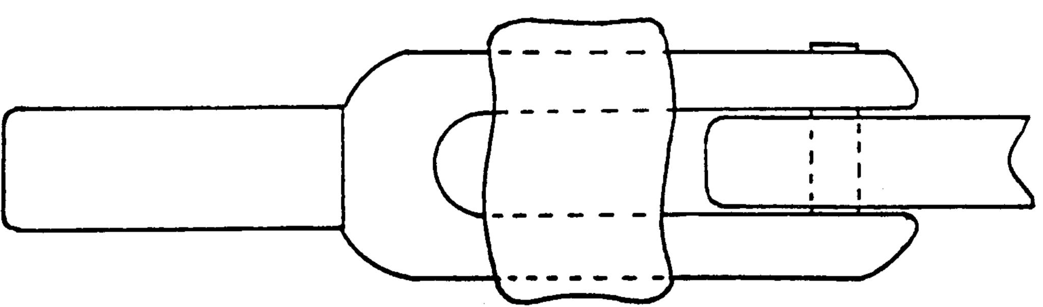
"Safety" all clevis links with 4.0mm. long fuel tubing.
