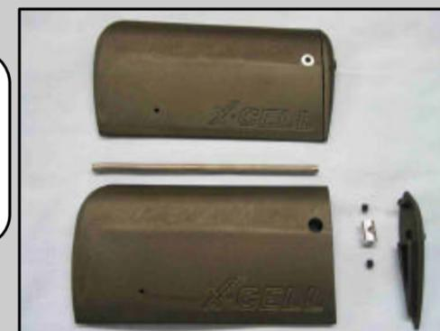
All New Pro-3 Fly bar Paddles. Easily assembled and allow for easy weight adjustment at any time. Thicker airfoil ensures smooth cyclic response. Weight ranges from 38 gms to 65 gms.
