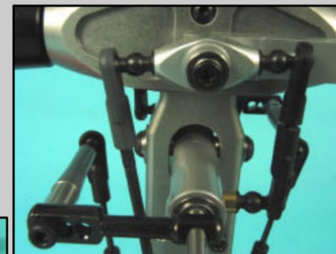
New design adjustable flybar control arms, allow 3 different flybar mix ratios. Also specially designed flybar tube and bell mixers allow you to choose just the right setup for your personal flying style.
