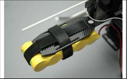
Install the battery on the top of the battery tray using the included Velcro (an optional position is on the bottom of the plate) as shown. Cut the material to length as necessary to wrap the battery both front to back and around the middle.
