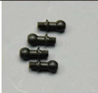
Select the two side bellcranks from your original model and remove the threaded balls. Select the four #0107 from Bag 2A. Apply a small amount of slow Cyanoacrylate glue to the threads on the ball and use a 1.5mm allen driver to insert the two threaded balls into each of the two bellcranks as shown in the photo.
