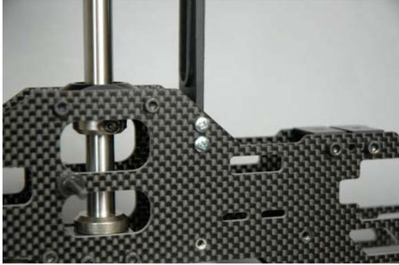
Finally, select the remaining two Phillips head mount screws for the anti-rotation guide from your original model.
