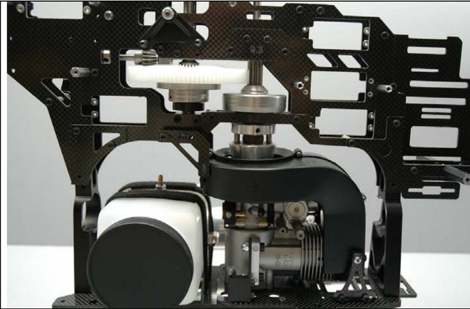
Position the upper and lower frames as shown. The bottom legs of the upper frame will slip over the tops of the frame support ladders previously installed on the lower plate.
