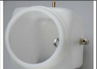
Connect the fuel clunk to a piece of flexible fuel line. The exact length of this line will depend on where you installed the fuel pickup in the tank, however it must be long enough for the fuel clunk to fit into the corners of the tank, but not be so long that the clunk can get stuck on the middle edge of the tank.
