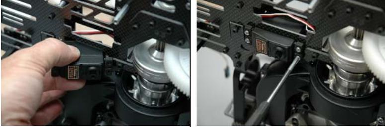
Insert the throttle servo into the frame position shown with the servo splined shaft towards the back of the model. Using the throttle servo mount bolts from your original model, apply a small amount of Loctite to the threads and tighten the servo into place. Follow your servo manufacturers instructions as to how tight these bolts should be
