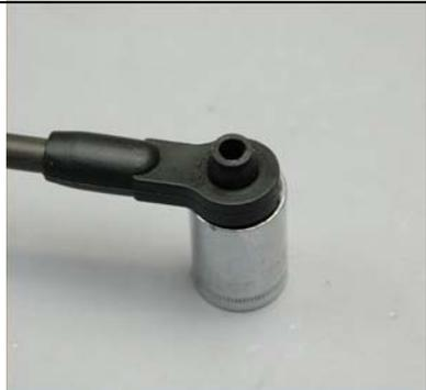
Insert a short M3 socket head bolt into the ball on one end of the support.
