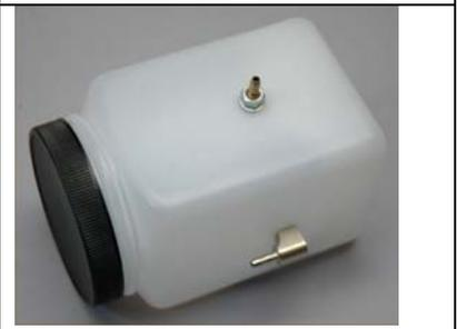
Apply the RTV around the outside lip of the fuel tank opening, and use your finger to even the adhesive and also to remove excess. Be careful to remove any adhesive that may be on the inside of the fuel tank or can get on the inside. (Loose cured RTV can get into the fuel system and plug the fuel pump or carburetor orifices).
