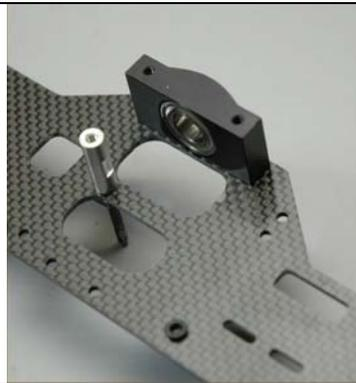
Insert the bolts from the outside of the left frame into the two holes at the top of the frame as shown
