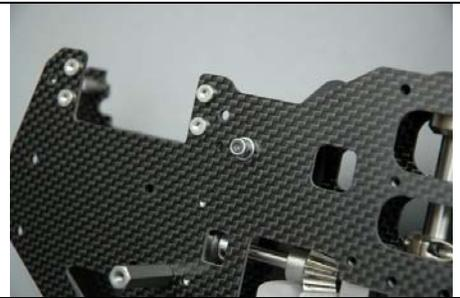
Select the #126-62 front doubler plate and lay it as shown on the outside of the right frame. Select two #0061 M3 x 8mm socket head bolts and one #0060-1 M3 x 6mm socket head bolt and insert as follows:
