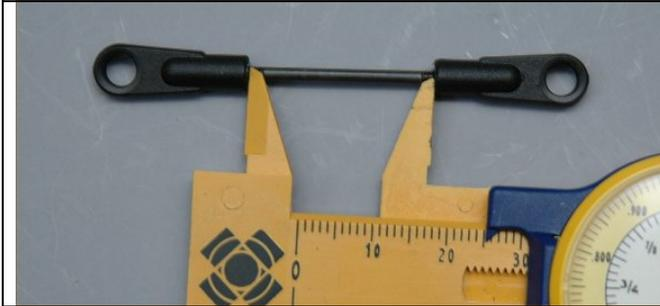
Thread the links onto both ends of the rods and tighten until the starting point for the gap between the ball links, measured at the base of the two links is 25.2mm.
