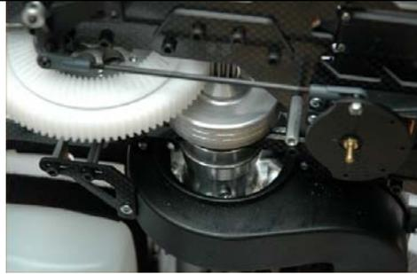
Install the pitch servo wheel from your original model on the elevator servo as shown with the servo cutout towards the rear. Install the threaded servo studs from your original model (use Loctite if your servo has a metal output shaft). The servo wheel must be perpendicular to the servo at the center of travel and the ball on the servo wheel/arm must be on the inside.
