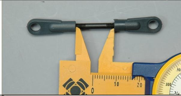
Assemble the elevator control rod by selecting the #121-4 M3 x 30 threaded rod and two #0133-1 grey ball links. Assemble the ball links as shown and tighten both. The typical gap between the base of the two links is 17 mm however depending on your servo you may have to slightly adjust it so that the elevator bellcrank is at 90 degrees and the elevator servo wheel is perfectly vertical.
