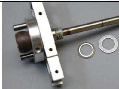
Now you can remove the extreme clutch block. You may need to heat the clutch driver to break the Loctite before removing the block
