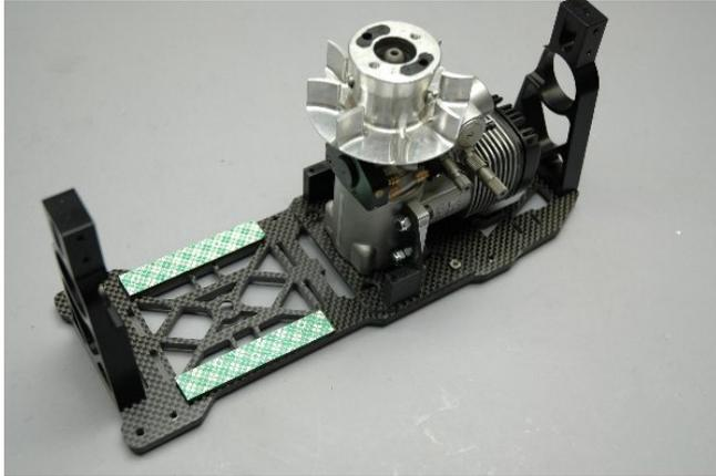
First tighten each of the four M3 bolts that attach the aluminum side engine mount blocks. When complete, remove them one at a time, apply blue Loctite and then reinstall and tighten them.
