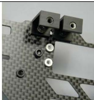
Select a #126-69 22mm spacer and a #0060-1 M3 x 6mm socket head bolt.
