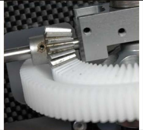
Now just slightly loosen the pinion gear socket screw that you marked so that the gear can be repositioned. Move the pinion rearwards until a smooth feel is achieved when the gears are rotated with minimal backlash in the gears. Again lightly tighten the marked set screw on the pinion gear.
