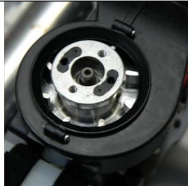
It is now time to mate the upper and lower frames. This will include pushing the clutch driver alignment ball and pins into the engine fan and dampers.
