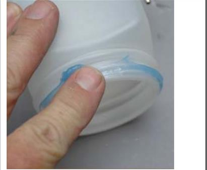
If you are using a pressurized fuel system (YS or OS with Kline pump) fuel cap must be sealed using blue or red RTV (clear may be affected by glow fuel).
