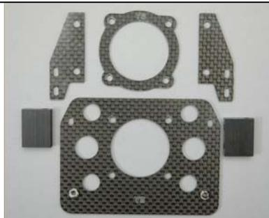
These are the parts that make up the engine mount assembly
