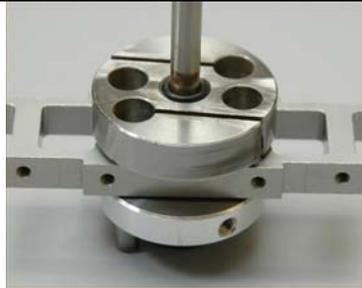
At this point you can reassemble the clutch onto the driver. Before threading the clutch on, place a small amount of blue Loctite on the driver threads. One side of the clutch has a small groove around the center of the clutch above the threads. This groove is installed on the top, or away from the bearing block
