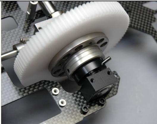
Assemble the constant drive assembly in the original order it was removed from your model. Place the assembly in the frame cutout between the middle and lower mainshaft bearing blocks as shown and align it with the mainshaft.
