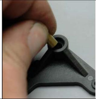
Select the two #106-02 flanged bearings. Push one of the bearing into the bearing cavity on one side of the bellcrank. The flange seats against the outside of the bearing cavity. Insert the #124-22 .305" brass spacer (the longest of the three spacers) into the bellcrank opening. Now take the final bearing and push it into the remaining bearing cavity.
