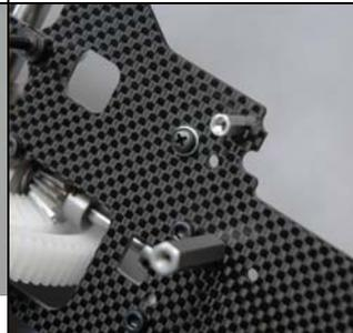
Now slip the completed bellcrank over the #0099 phillips head bolt installed earlier in the configuration shown in the photo.
