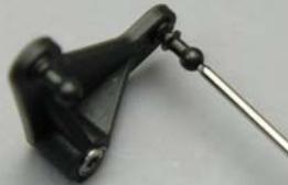
Carefully tighten so that the threaded balls seat onto the bellcrank. Do not overtighten.
