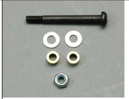
See the photo for the parts needed to install the elevator bellcrank onto the left frame and the installation sequence.
