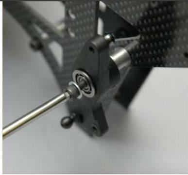
Using the M3 x 6mm bolt and washer from your original model, apply a small amount of blue Loctite to the bolt threads and insert the bolt into the bellcrank stud. Tighten firmly.
