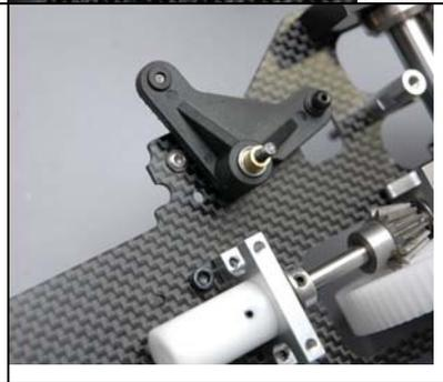
Finally slip the .187" brass spacer over the protruding bolt and seat it up against the bellcrank bearing.
