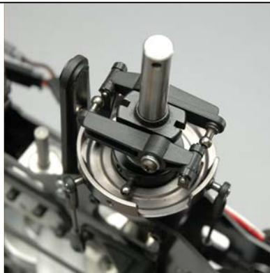
Select the washout assembly previously removed from your original model and slip it over the mainshaft.
