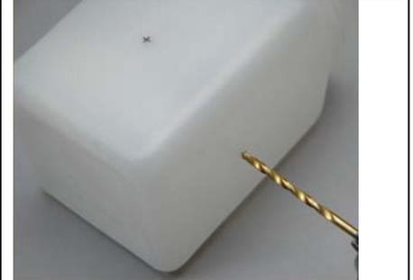
Remove the tank lid. First use a 1/8" bit and drill both holes. Then change to a 3/16" drill and re-drill the holes. By using two different drill bit sizes it prevents the plastic from being torn by drilling the hole too big in one step. Remove any tank shavings from inside the tank
