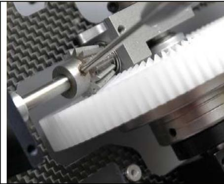
Now rotate the pinion gear again and remove the socket set screw that is against the t/r shaft flat. Apply a small amount of blue Thread lock to the threads on this socket screw and reinstall it. Tighten against the flat on the t/r shaft. Now rotate the pinion a final time and fully tighten the remaining socket set screw
