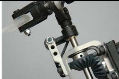
Now thread the remaining grey ball link onto the exposed control rod at the back of the push rod.
