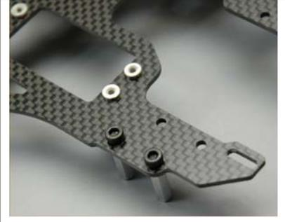
Insert the two bolts from the inside of the left frame through the two holes at the bottom of the gear drive cutout. Apply a small amount of blue Thread lock to the threads and thread the fan shroud spacers onto the bolts on the outside of the frame. Fully tighten using appropriate tools. These are the mounts for the fan shroud plate.
