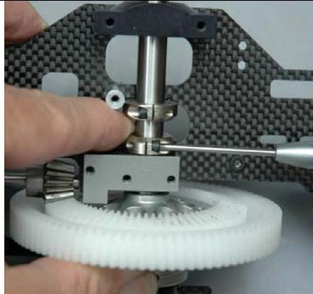
Using a 1.5mm allen driver, snug the socket screw marked in an earlier step as being on the flat of the t/r shaft.
