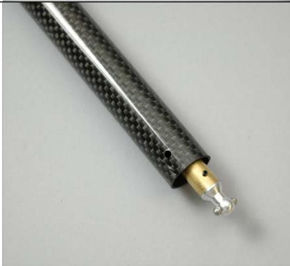
Push the tube drive into the tail boom from this end. It's not critical which end of the tube drive is inserted into the tail boom first.
