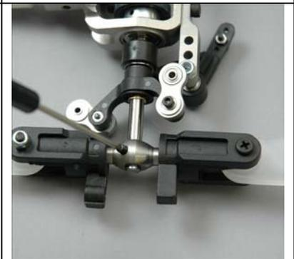
Hold the t/r hub and output shaft in this position and tighten the previously inserted dog point set screw on the other side of the t/r hub until it begins to engage in the t/r shaft.
