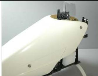
Install the four grommets into the canopy mount holes previously drilled into the canopy. These are best installed by pushing one side of the grommet channel into the hole and then using a flat bladed instrument to push the rest of the grommet in. Be careful not to tear or cut the grommet.
