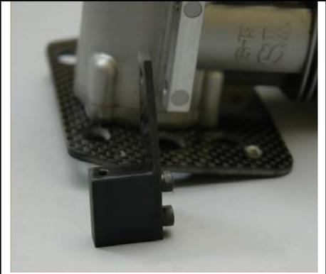
Assemble the two engine side mounts as shown. Assemble the flat engine mount plates to the aluminum mount blocks using 2 each M3 x 6mm bolts in each block. No washers are used. At this time only lightly tighten them. Do not fully tighten them yet or apply Thread lock. The plates and blocks are not marked left or right but must be assembled as shown.
