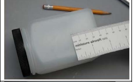
The tank is 2-7/8" (73mm) side to side. The center of the tank is 36.5mm or 1-7/16". Center the marks you just made so that they are centered side to side and mark them for drilling.
