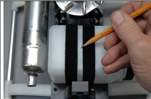
After positioning the fuel tank, use a pencil mark a spot on the top of the tank exactly between the two Velcro strips. Getting the exact side to side location correct is more important than getting the front to back position correct. Later you will install the fuel vent fitting here so you want to make sure it can clear the Velcro.
