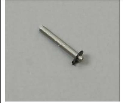
The first clip needs to be pushed over the pin to the approximate position shown. An easy way to do this is to drill a small hole in a block of wood (#30 drill), place the clip/pin over the hole and lightly tap the pin through the clip into the hole. If you tap it in too far, the clip can be adjusted using a pair of pliers.
