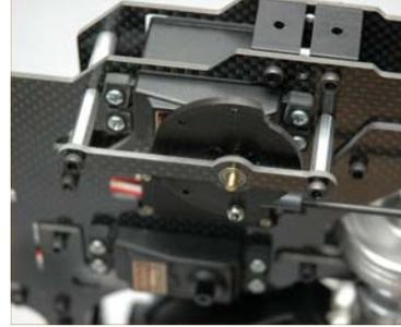
Snap the control rod onto the ball on the servo wheel and onto the control bellcrank on the left side of the frame.
