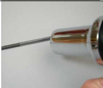
Measure 14-½" from the back of the pushrod and using a pencil, mark a line on the pushrod. Slip the Teflon tube over the pushrod from the back of the tube and slide it forward until you can see the pencil mark through the center of the tube.
