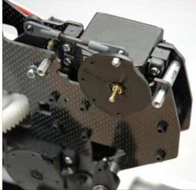
Install the elevator servo wheel on the elevator servo as shown with the servo cutout towards the rear. Install the threaded servo stud (use Thread lock if your servo has a metal output shaft). The servo wheel must be perpendicular to the servo at the center of travel and the ball on the servo wheel/arm must be on the inside.
