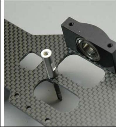
Insert the bolts from the outside of the left frame into the two holes at the top of the frame as shown
