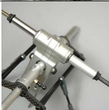
If you used the additional shims on the opposite side of the head axle, install the same shims on this side of the axle. Finally using circlip pliers, slip a #0848-2 retainer about 1/2" over the end of the now protruding head axle.
