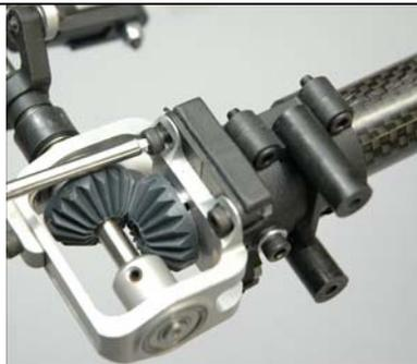
Place the left hand clamp over the rear of the tail boom, opposite of the installed right hand clamp. Using a 2.5mm allen driver to tighten the four 10mm bolts into the hex nuts on the left hand clamp and tighten firmly
