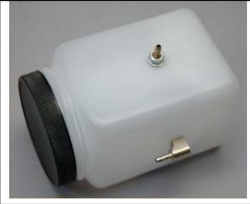
Test this by installing the fuel line/clunk and manually reposition the tank in all conceivable positions and visibly observe the clunk. Adjust the length until it touches the most areas of the tank without getting stuck. When you're satisfied with the position, push the fuel line over the fuel pickup installed in the front of the tank. Firmly thread on the cap of the tank, it is now complete.
