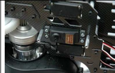
Route throttle, aileron, and pitch servo wires through the frames toward the front radio area. It is suggested that you use a piece of Velcro to wrap these wires together to prevent them from rubbing on the frames or other components.
