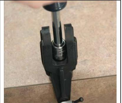
Select the one that fits loosely on the axle and drop it into the cavity on the inside of the blade grip such that the groove in the bearing is visible or facing towards the outside of the grip.
