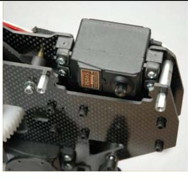
Another close-up view of the servo motor mounted in the rear servo cutout of the model's frame. The servo is secured with bolts. |
