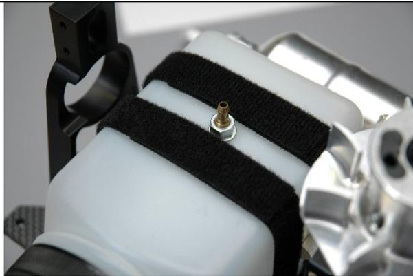
Tighten the two Velcro strips to firmly attach the tank to the bottom plate.
