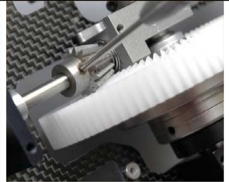
Now position the pinion gear where it just slightly extends past the inside of the crown gear. See the photo for the proper position.
