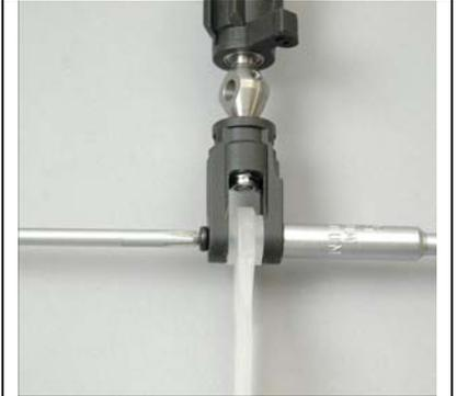
The t/r assembly turns at a very high speed and must be balanced before installation to ensure smooth operation. In order to balance the assembly, you will need a balancer of some sort like the one shown.
