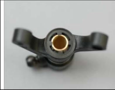
Now take the remaining clip and install it over the pitch slider. For best results, rotate it 45° from the first clip so that the retaining fingers don't align with the fingers on the first clip. This will ensure that this assembly does not come loose.
