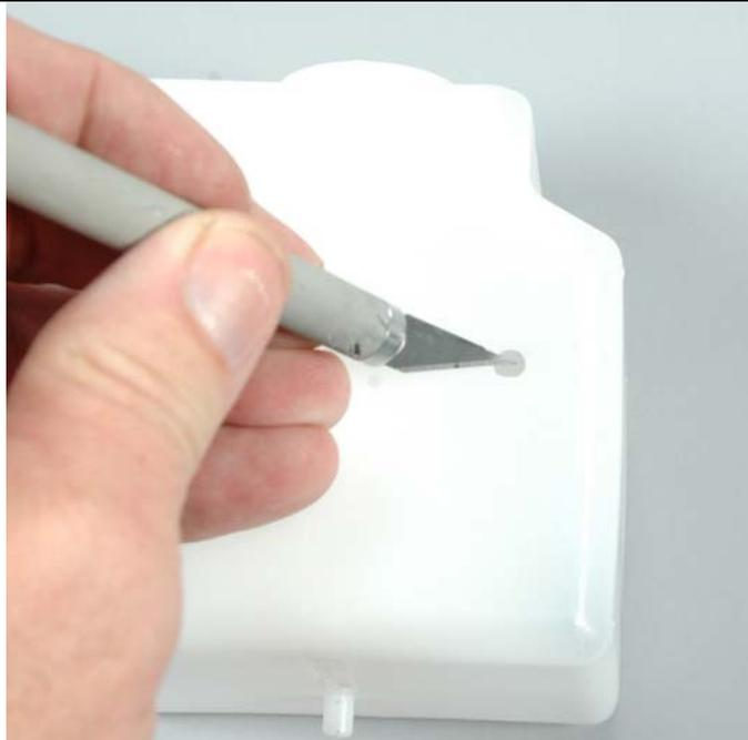
Remove any flashing from the drilled holes using a razor knife. Be careful to not enlarge the holes
