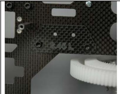
Select the left upper clutch plate and two #0060-1 M3 x 6mm socket head bolts. Position the plate on the left frame as shown and using a small amount of blue Thread lock on the threads, thread the bolts into the PEM mounting nuts in the frame half. Tighten both bolts firmly. Make sure you install the marked left plate on the correct side.
