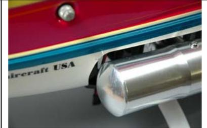
Hand fit the exhaust system to determine what if any cut-outs need to be made to the canopy. Mark the canopy and use a cutoff wheel or drum sander and a rotary tool to make any cutouts needed. Make sure there is at least 5mm clearance between any part of the canopy and the exhaust system.
