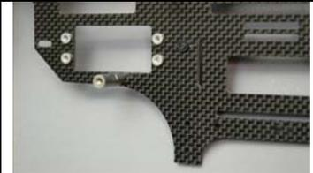
Attach the doubler plate to the outside of the front bottom part of the left frame with one #0060-1 M3 x 6mm socket head bolt in the top of the doubler threaded into the PEM nut. Apply a small amount of blue thread lock to the bolt threads, but don't fully tighten yet. Now install one #0061 M3 x 8mm socket head bolt in the front of the doubler. Apply a small amount of blue Thread lock to the threads of the exposed bolt and thread on a #115-20 frame spacer. Now tighten both bolts snugly.
