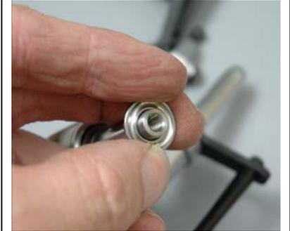
Now select a #0324 washer as shown and drop it into the inside blade grip cavity on top of the previously inserted bearing.
