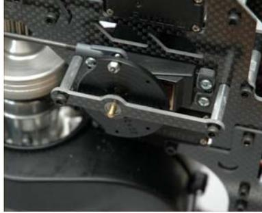
Snap the control rod onto the ball on the servo wheel and onto the control bellcrank on the right frame.
