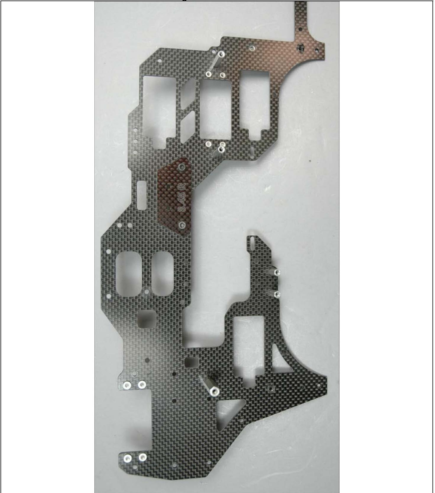
Assembled View of the Inside of the Right Frame Half
