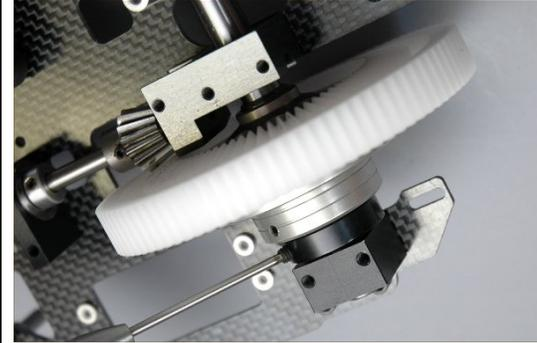
Hold the bottom of the constant drive and turn the main shaft until the holes align in the shaft, constant drive and constant drive retaining collar. Select the #0840-6 retaining dowel pin and push it through the constant drive retaining collar and through the shaft. If the pin won't go fully in, remove it and turn the main shaft 180 degrees and push the pin in. Since this was already installed on this shaft, any issues with this fit would have already been resolved.
