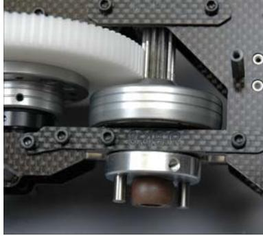
Install two #0061 bolts in the front and back open holes in the lower ratio plate and just snug them tight. Now install a #0060-1 6mm bolt in the remaining hole and just snug it tight.
