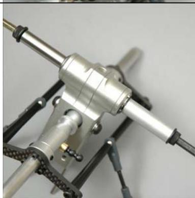
If you used the additional shims on the opposite side of the head axle, install the same shims on this side of the axle. Finally using circlip pliers, slip a #0848-2 retainer about  $\frac{1}{2}$ " over the end of the now protruding head axle.
