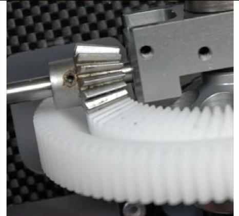
Using two fingers push the constant drive assembly/crown gear firmly up against the pinion gear while holding the lower retaining collar up against the middle mainshaft bearing. Tighten the lower retaining collar. Do not overtighten these bolts as the collar can crack. The correct way to tighten these bolts is to tighten until the socket head contacts the retaining collar and then tighten an additional  $\frac{1}{4}$  turn.
