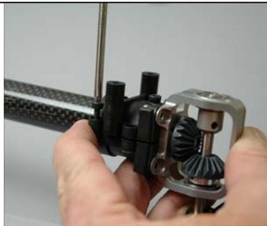
Insert four M3 x 10 bolts into the t/r mount clamp half bolt bosses as shown. Thread them in until the bolts are flush with the bottom face of the clamp.
