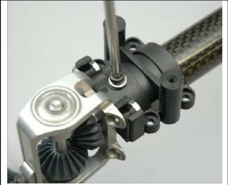
Using a 2.5mm allen driver, press down on the M3 bolt on the side of the clamp as you thread it into the t/r transmission. Be careful to make sure you don't cross thread or strip the threads. Tighten lightly only
