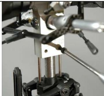
Finally, select the two #0067 M3 x 14 socket bolts, apply a small amount of blue thread lock and thread them into the clamp holes at the base of the rotor head. Tighten these bolts snug and then tighten an additional 1/8 turn to clamp the rotor head.
