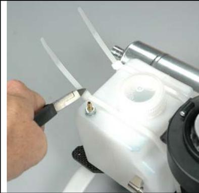
Push the ends of the straps into the strap grips to capture the tank as shown. Pull each strap snug against the tank. You may need to reposition each strap slightly to make sure that the grip stays on the rear angled area of the fuel tank. Continue to snug the straps down until there is no slack in the strap under the frame, however do NOT over tighten these. Its possible to deform the tank if these are pulled too tightly.
