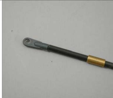
Select the 42mm control rod and one grey ball link. Thread the rod into the link until it bottoms out. Use #80 grit sandpaper to roughen up all of the exposed push rod (you should remove most of the black color).
