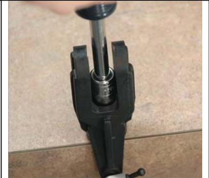
Place this back of this grip on a flat surface as shown. Now take the largest socket that will fit inside the grip and press on the rear thrust bearing race until you hear the bearing pop into place in the blade grip. If your "rock" the socket around, this can be easily accomplished.
