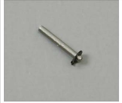
The first clip needs to be pushed over the pin to the approximate position shown. An easy way to do this is to drill a small hole in a block of wood (#30 drill), place the clip/pin over the hole and lightly tap the pin through the clip into the hole. If you tap it in too far, the clip can be adjusted using a pair of pliers.
