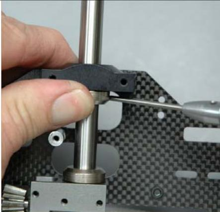
Now using two fingers, push the upper retaining collar up against the bottom of the upper mainshaft bearing. Repeat the tightening process previously outlined for the lower mainshaft retainer collar
