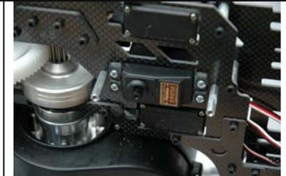
Route throttle, aileron, and pitch servo wires through the frames toward the front radio area. It is suggested that you use a piece of Velcro to wrap these wires together to prevent them from rubbing on the frames or other components.
