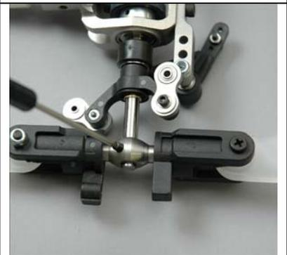
Hold the t/r hub and output shaft in this position and tighten the previously inserted dog point set screw on the other side of the t/r hub until it begins to engage in the t/r shaft.
