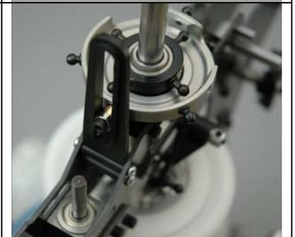
The swashplate should slide easily down the swashplate. Using a finger, slightly bend the plastic anti-rotation guide outward just enough to slip the bearing into it. When you release the guide, it will capture the anti-rotation bearing which prevents the outer swashplate from turning.
