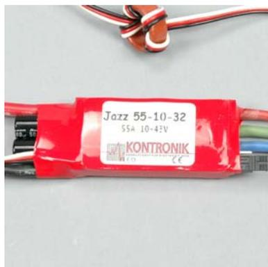
This allows for a more consistent head speed throughout the flight by using less of the available "speed" of the system initially and then using all of it later in the flight as the battery discharges.
