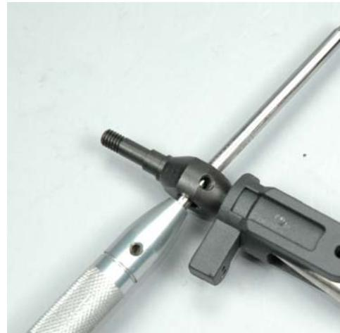
**Building Notes:** tighten the retaining nut carefully until it is snug. Now loosen it slightly until the blade grip moves freely.
