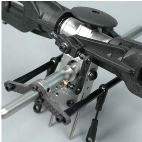
**Building Notes** – snap one end of the assembled link onto the double ball on the bell mixer and the other onto the double ball on the flybar carrier. Repeat for the other side
