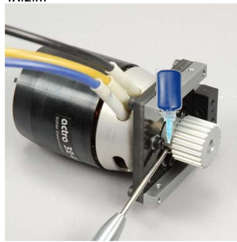
**Building Notes:** Align one set screw with the flat on the motor shaft. If there is no flat on the motor shaft use a grinding tool to cut one.
