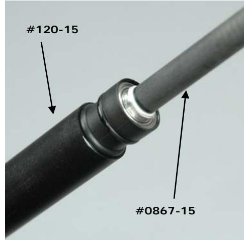
**Building Notes** – before inserting the tube drive into the tail boom as shown, spray inside the boom with a spray glass cleaner (like Windex®). This will make the tube drive easier to insert
