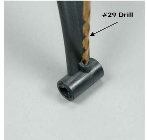
**Building Notes:** Locate the molded bosses on each of the landing gear struts. Find the center of drill through the boss with a #41 drill. The re-drill with the larger #29 drill. Drill all four bosses in this way
