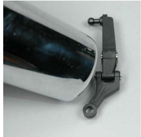
**Building Notes:** Heat Plastic with heat gun until hot and then move the link back and forth until it loosens up. Don't Overheat.
