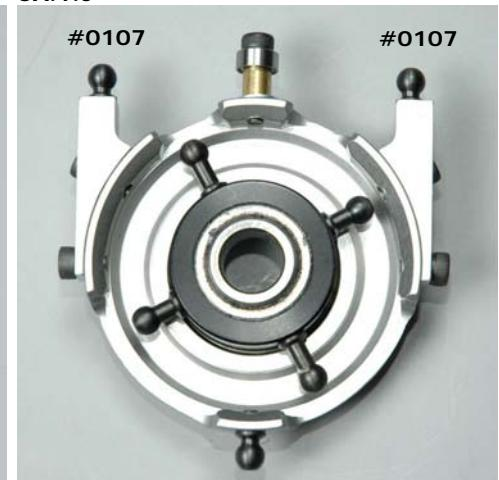
**Building Notes:** Thread set screws into the bearing tension holes on the bottom of the swashplate. Do not overtighten.
