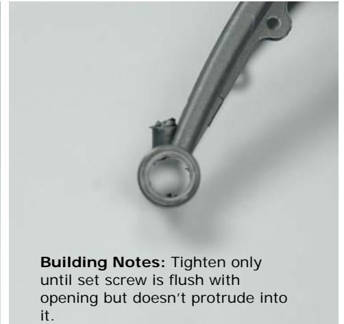
**Building Notes:** Tighten only until set screw is flush with opening but doesn't protrude into it.
