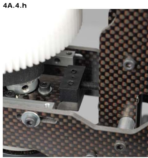
**Building Notes:** Depending on the drive ratio, you may need the shorter or longer bolt to set the belt tension. Insert the bolt/plate assembly through the back frame channel and thread into the motor adjustment block as shown
