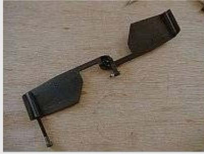
Large screws are used as weights and to keep a long pivot pin from flying out.
