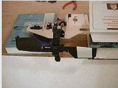
The manual outlines proper balancing. Black and white balance tape is included to match the color of the blades and paddles. I purposely used contrasting colors for photo purposes and to make in-flight orientation easier.
