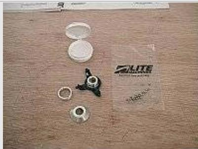
These are the swash plate parts prior to assembly. The white container holds lubricating grease.
