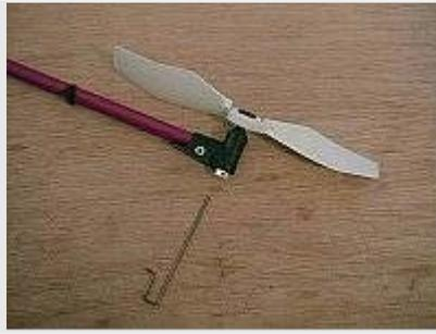
The tail pitch rod goes through the center of the tail shaft.
