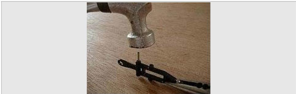
A light tap with a hammer positions the pivot pins in place.
