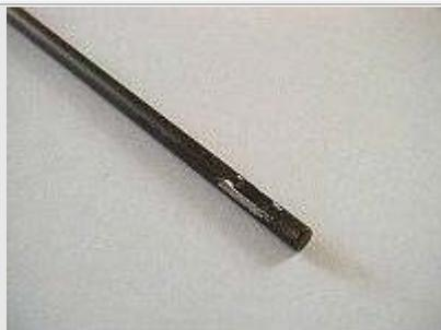
The main shaft needed to be sanded down a little in order to slide through the bearing mounts.
