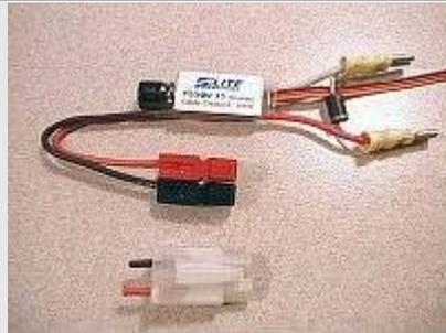
The only real change I made was to remove the white Molex type connector from the speed controller in favor of the Sermos type commonly used by electric fliers.
