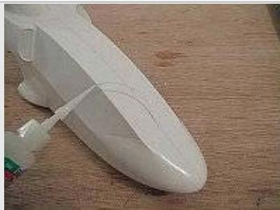
Thin CA was used to glue canopy halves together. Follow the instructions carefully as not all of the parts are completely glued.
