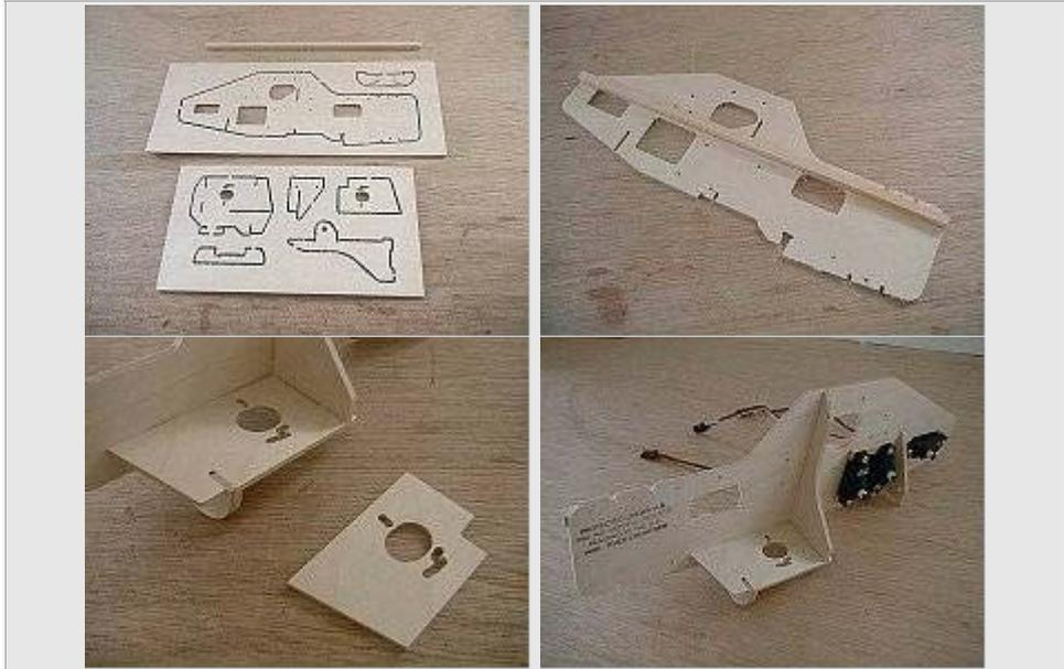
The crutch is a simple 3-D puzzle that is glued together. Note the adjustable motor mount and that the servos are mounted very early in the constructions stages.
