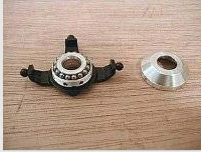
The nearly completed swashplate is ready for final top piece to be screwed on.
