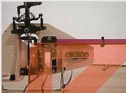
A drafting triangle is used to align the tail boom.
