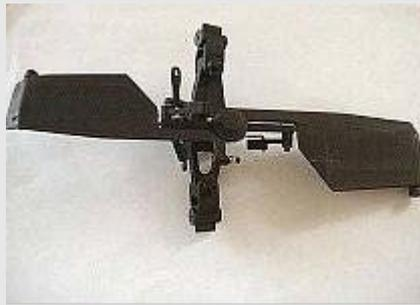
The finished head is ready to be balanced. The blade grips come in 4 and 6 degree preset blade pitch.
