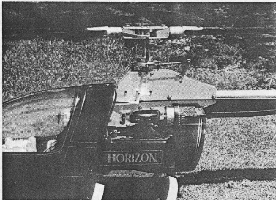
Our reviewer installed a separate collective servo; Horizon features a hinged servo tray for collective and tail rotor mixing. Also has a flex tail rotor drive.
