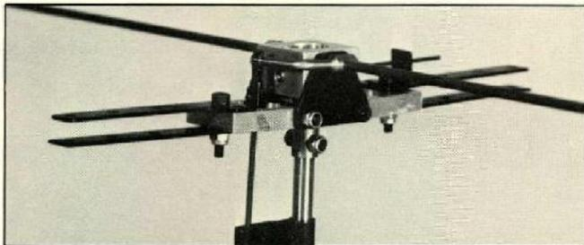
Cricket's simple but effective fixed pitch rotor head. Comes assembled--ready to fit flybar and blades.
