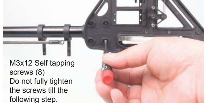
1) Align the mounting posts from the front transmission gearbox with the mounting posts at the rear of the main frame. The horizontal fin on the tail boom facing should face up so the rudder pushrod and tail boom support struts hang below the tail boom.
