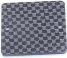
(Optional Item) CNE555 Carbon Gyro Mounting Plate can be used to mount the gyro at the rear of the helicopter. It is extremely important that the gyro is attached using only the supplied two sided tape onto a clean flat surface. Keep all wires and components away from the gyro housing. Do not use straps or elastics to secure the gyro.
