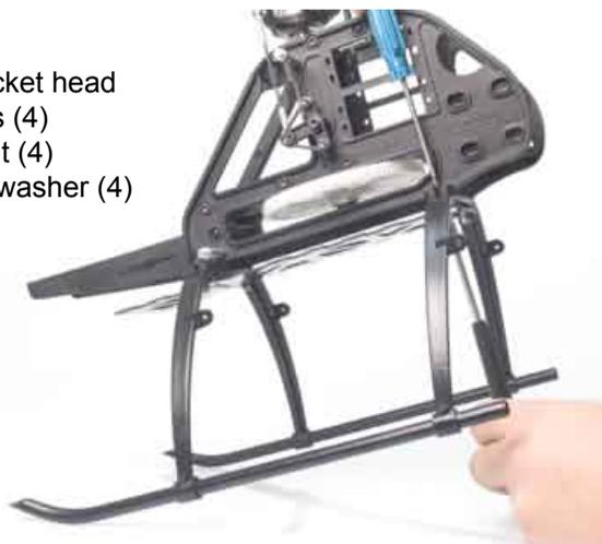
(1.3) Align the mounting points on the main frame with the holes in the landing struts and the battery tray.
