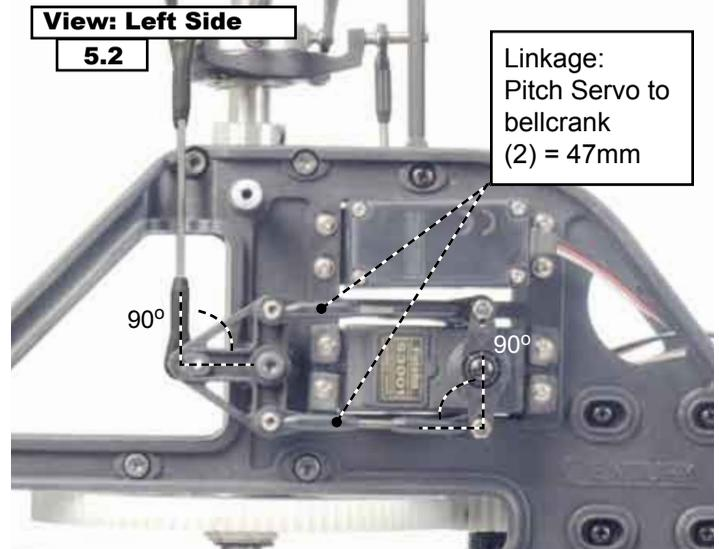
(5.2) The pitch servo will mount with a full servo arm on the lower opening of the left side of the main frame. Use the 4 servo screws and 2 servo mounting tabs to mount the pitch servo with the servo arm further toward the rear of the frame (pictured above).
