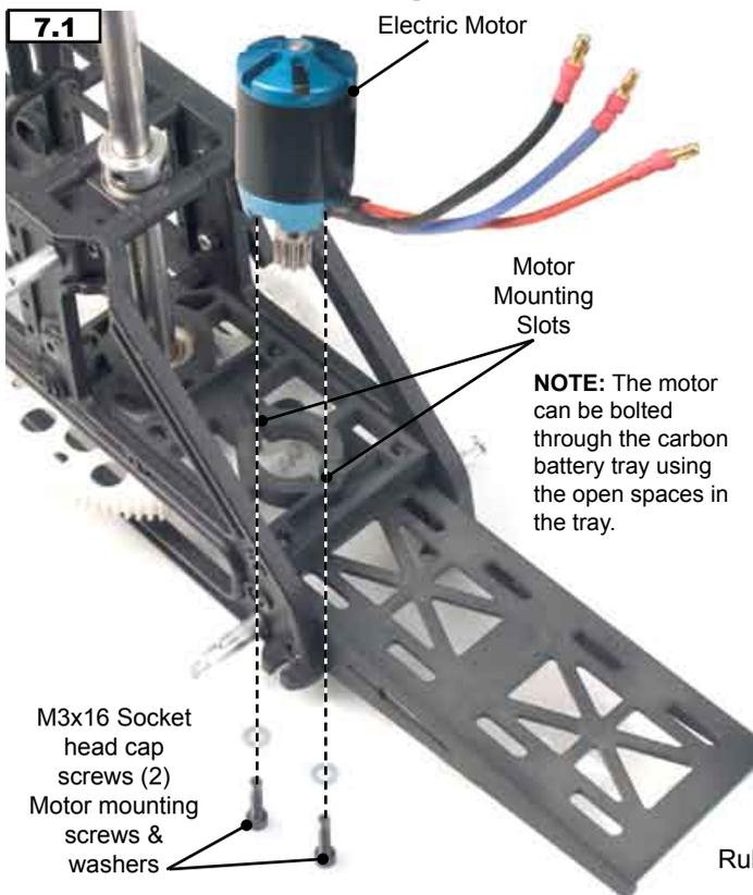
(7.1) The key to installing the motor is the gear mesh. The elongated slots for mounting the motor allow space to adjust the mesh between the motor pinion gear and the main gear. Install the motor to the motor mounting plate and secure with hardware provided by the manufacturer of the motor.
