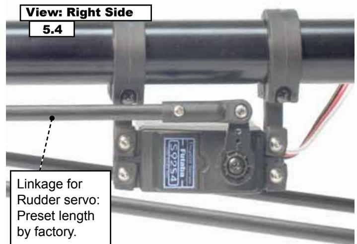
(5.4) The rudder servo will mount with a half servo arm on the servo bracket on the tail boom. Use the 4 Servo screws and 2 servo mounting tabs to mount the servo with the servo output facing the forward right side of the helicopter (pictured above).
