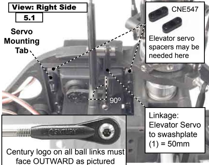
(5.1) The elevator servo will mount with a half servo arm on the upper opening of the left side of the main frame. Use the 4 servo screws and 2 servo mounting tabs to mount the elevator servo with the servo arm output facing toward the rear inside of the frame (pictured above).
