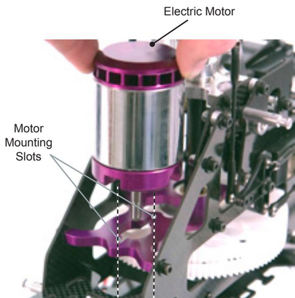
**NOTE:** The motor can be bolted through the carbon battery tray using the open spaces in the tray and Main Gear
