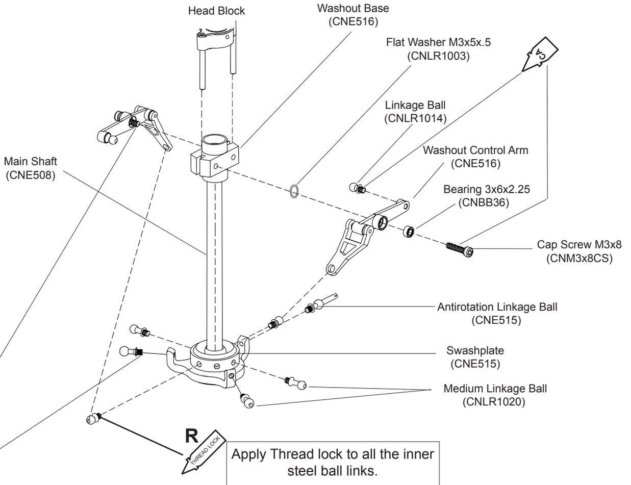
\*Hint: Undo the cap screws and linkage balls to the assembled parts. Apply CA on metal to plastic assembly. Apply blue thread lock on metal to metal assembly. Do not over tighten when screwing the attached assembly to its subassembly.
