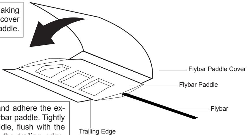
Hint: Cover the bottom end of the flybar paddle and adhere the excess covering material to the trailing edge of the flybar paddle. Tightly pull the top side of the cover over the flybar paddle, flush with the trailing edge and cut the excess material along the trailing edge.
