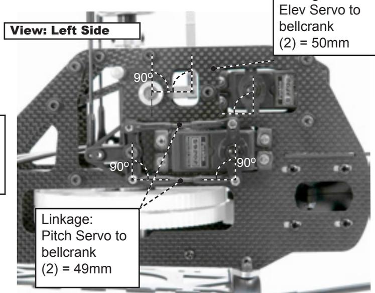
The pitch servo will mount with a full servo arm on the lower opening of the left side of the main frame. The distance between the steel balls (center of ball) on the servo arm should be 12.5mm. Use the 4 servo screws and 2 servo mounting tabs to mount the pitch servo with the servo arm further toward the rear of the frame (pictured above).
