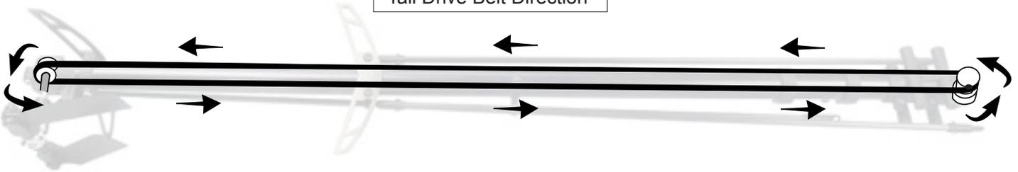
While facing the tail, the tail blades should spin counter clockwise.
