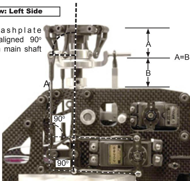
After installing the three cyclic pushrods, the swashplate should sit level.
