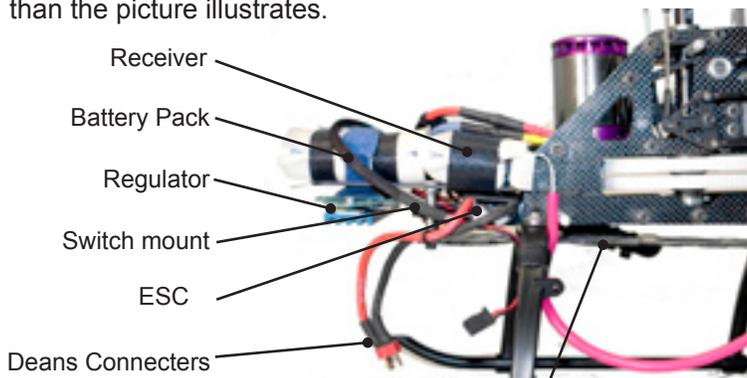
**HINT:** Installing industrial strength velcro will help secure the batteries during aerobatics.
