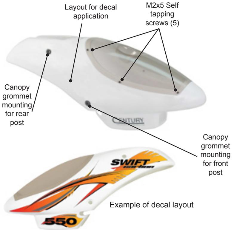
The canopy may require cutting to make space for certain batteries or other extras. We recommend the use of a dremel. A face mask and goggles should be used when cutting fiberglass.
