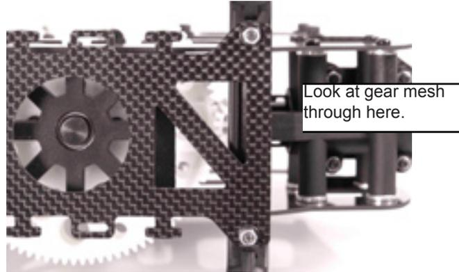
1) Align the mounting posts from the front transmission gearbox with the mounting posts at the rear of the main frame. The horizontal fin on the tail boom facing should face up so the rudder pushrod and tail boom support struts hang below the tail boom.
