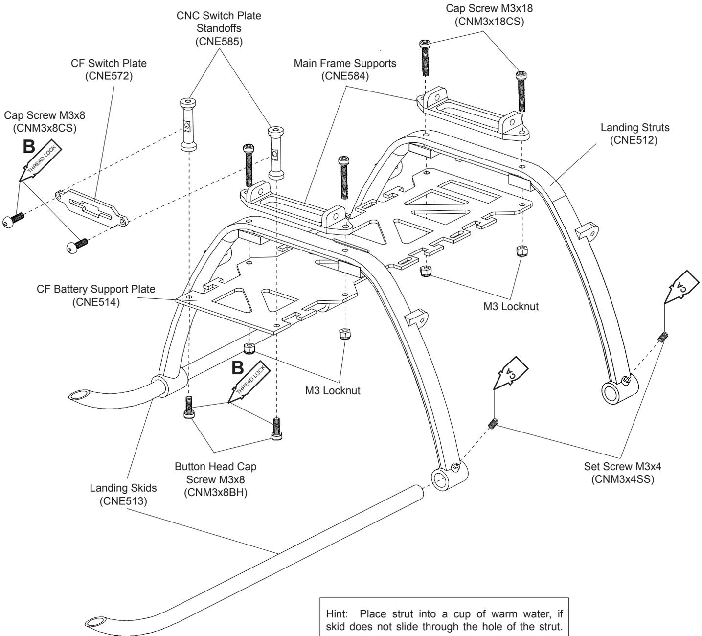
Hint: Place strut into a cup of warm water, if skid does not slide through the hole of the strut.
