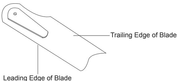
For aerobatic/stunt flight, the Swift Carbon 550 flies best using symmetrical rotor blades. For your convenience you can also use semi-symmetrical for smooth aerobatics and scale flying.
