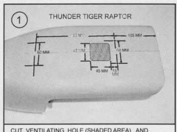
CUT VENTILATING HOLE (SHADED AREA) AND MECHANISM MOUNTING HOLES (3.5 MM) AS SHOWN.
