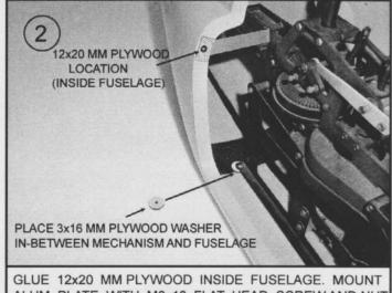
ALUM. PLATE WITH M3x10 FLAT HEAD SCREWAND NUT.
