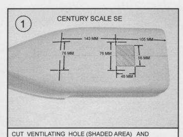
MECHANISM MOUNTING HOLES (3.5 MM) AS SHOWN.
