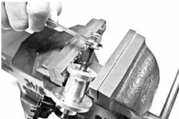
Because you have no use for the propeller hub, you can use a wrench or vice to grab onto the hub while trying to undo the stud. Grabbing onto this aluminum hub may damage the hub but it's of no use in this build. Once this stud is loosened, you can remove the propeller hub.
