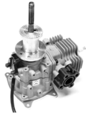
First undo the nut and remove the propeller washer. Screw down the original nut onto the stud followed by the locknut.
