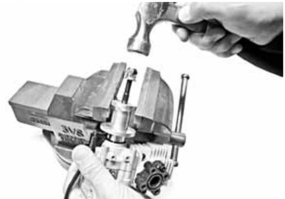
Remove the stud and hand tighten it a few threads into the crank. With the propeller hub still in the vice, gently tap on the head of the stud with a hammer while supporting the engine with your other hand. This will loosen the hub from the crank shaft.
