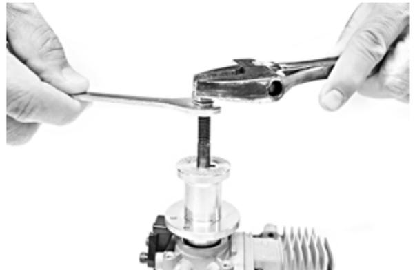
Tighten down on the top lock nut while applying opposite force (unscrewing) to the second nut using the Zenoah supplied wrench. This will allow you to lock the nuts together.
