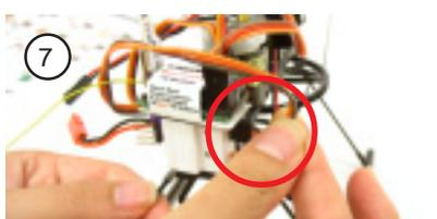
7. Plug mixer rudder lead into gyro (signal wires must face each other).
