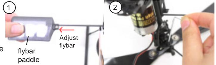
2. Tighten the two set screws in the flybar control arms to secure the flybar using the supplied allen key. Flybar paddles must be parallel to each other and the ground when the swashplate is level. Make sure the bolt head in each paddle faces upwards.
