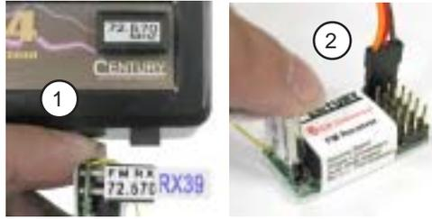
2. Note that all electronics plug into the receiver with the wires as pictured (orange wire faces receiver label). Follow the diagram for each electronic connection. Once the electronics system is connected and the transmitter is turned on, follow this step-by-step process to check your equipment.
