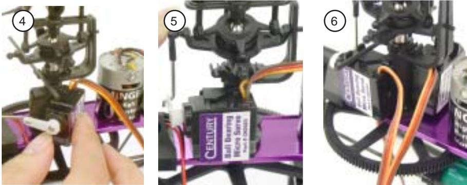
4. Once the mounting position of the servo is determined carefully mount the servo to the mast tower. If the servo has a label on the same side that will mount with double sided tape, peel off the label and clean the surface using rubbing alcohol.
