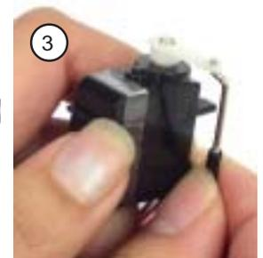
3. Some servo arms require widening the hole in the arm in order for them to accept the Hummingbird's pushrods using a #55 drill bit [1.34mm or 0.052"].
