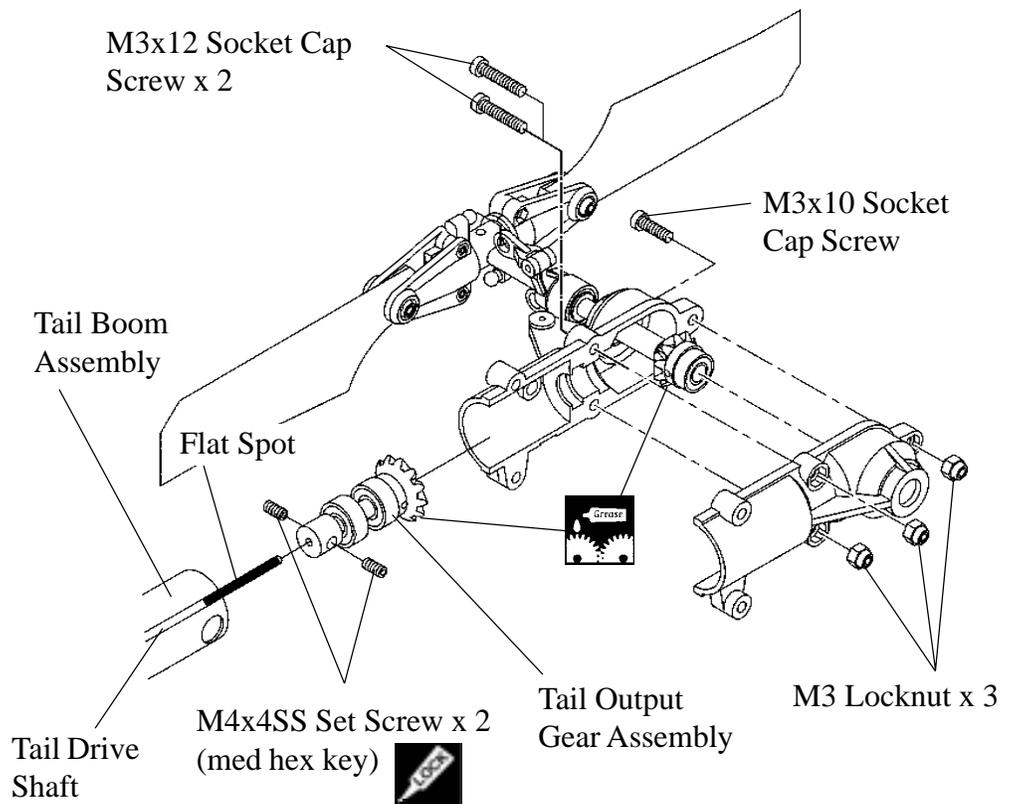
**Tip** Apply red locktite to the drive shaft end **only** and insert into the gearbox input shaft. Do not use on set screws, only bond the wire shaft to the input shaft. Tighten the set screws equally to make sure the wire and input shaft spin on the same center, especially when making field adjustments through the hole in the gearbox ( any clicking from the tail box indicates this problem.)
