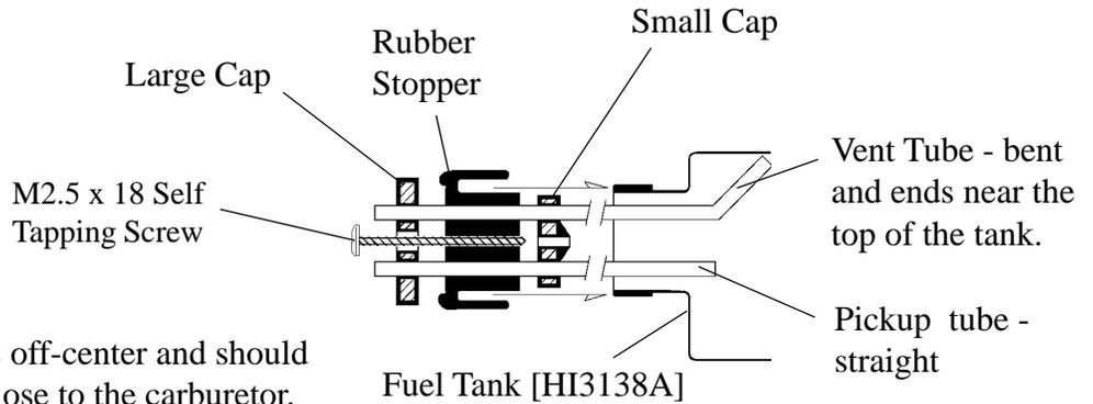
Note: The fuel tank opening is off-center and should be installed upwards to align close to the carburetor.
