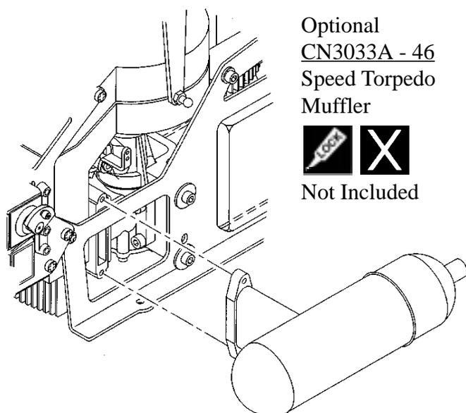
Attach the muffler to the engine with the screws provided with the muffler using threadlock. Attach the pressure tap to the top of the muffler and the M4x6 Phillips Machine screw to the bottom hole in the muffler, remember to use threadlock on these parts.
