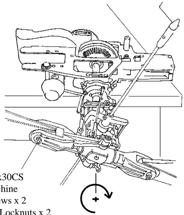
When attaching the main blades, the direction of rotation is clockwise, when looking on top of the helicopter.
