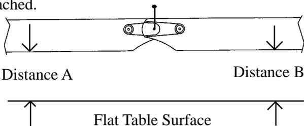
Bolt the blades together and support by the ends of the bolt off a flat surface. If one blade tips to one side add small pieces of tracking tape until both blades hang an equal distance from the table (Distance A = B). Attach the Main Blades to the helicopter using two 4x30mm Socket Head Cap Screws and M4 Locknuts.
