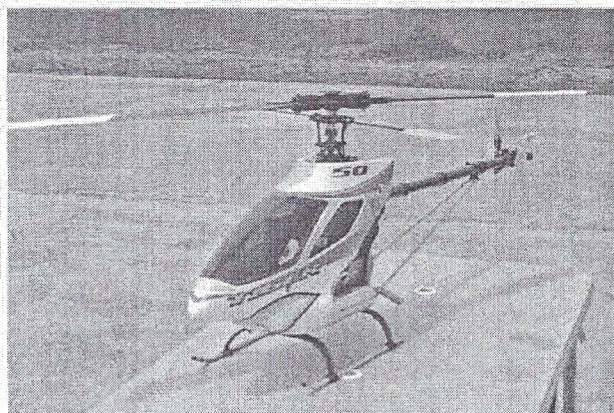
The Tiger's ready to roar ("Ready to Roar" ... Ash ... ouch! ED)you through some aerobatic maneuvers. Note the absence of the horizontal tail and the shorter flybar with thin KSJ paddles.
