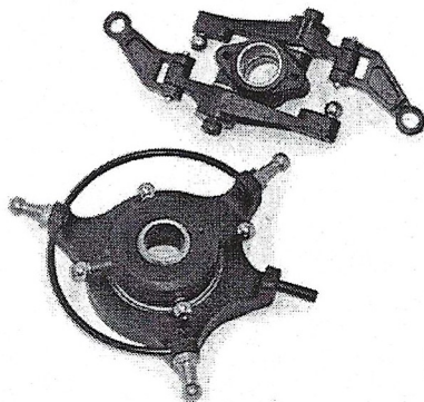
Note different ball link lengths on swash. Also note metal sleeve inside wash-out base. Nice touch.
