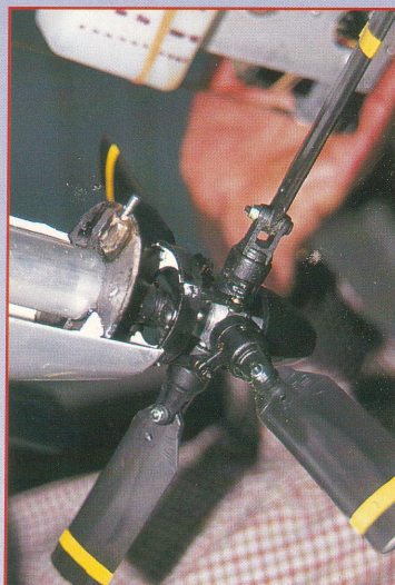
Pitch control for the four bladed propellers
