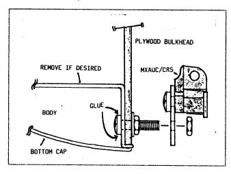
16 screws in the plywood 'U' facing forward and tighten a lock nut onto a washer.
