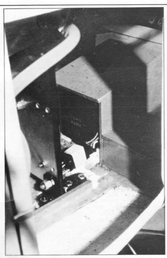
If doing it again, J.D. would move gyro further forward and make an air intake in the floor hereabouts. Note also stiffening added to side in case of grabbing by starting belt.
