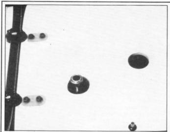
Not mentioned in test. J.D. moved front leg further forward using existing parts. Glass-fibre sheet spreads load for front chassis mounting bolts. They're all replaced by cap heads during rapid removal phase!
