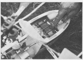
Above left: the complete tail rotor assembly. The tail skid has been extended a few inches to prevent the tail rotors chewing grass. Above: the radio installation showing four servos of Swan R/C system side-by-side in fuselage pod.
