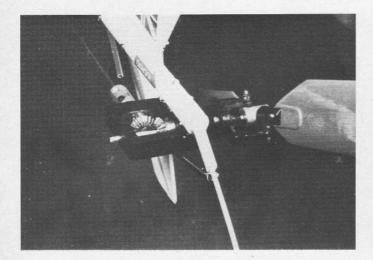
fitted is the heat sink on the engine cylinder head and after a thorough check over on the tightness of all nuts, angles of blades, freedom of movement of all controls, etc, we are ready to run the engine and adjust the throttle for an even tickover and smooth open up to full power.
