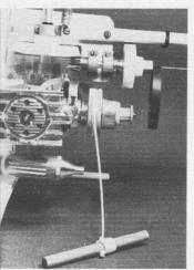
Far left: the main drive assembly mostly complete. Note the Kavan carb on the Veco 19 motor. Left: the motor is pull started and the drive belt slipped over the pulley when the engine is running. The correct tensioning of the belt is therefore essential.
