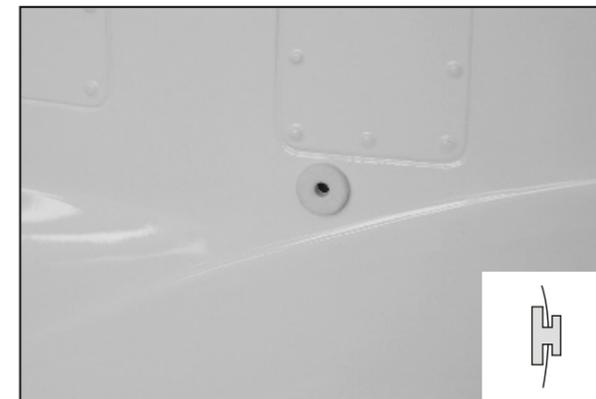
11. Drill the hole on the molded dot. Next enlarge the hole at about 8mm in diameter. Insert the Silicon Grommet on the hole. The smaller side faces outside.
