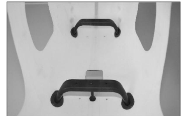
4. Remove the landing skid assembly from Heli. Remove the brace from the aluminum strut. Do not remove the strut and skid pipe as they are already adjusted and secured. Place the brace in place and install the strut and skid pipe onto the brace. You may apply Vaseline on Silicon Fairing to increase the lubrication for easier installation.
