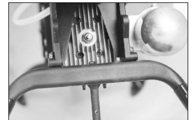
14. Secure the helicopter onto the landing brace with two 3x25mm Socket Screws, two 3 x23mm Socket Screws and four M3 Locknuts. Start from the rear brace then the front. Now you can CA the Silicon Landing Fairing in place.
