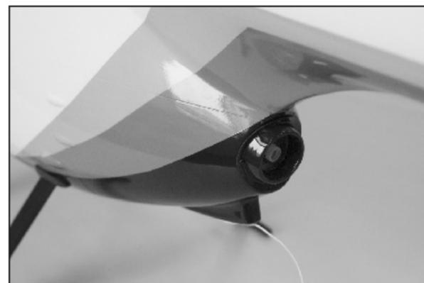
21. Secure the exhaust vent in the place with four 2x5mm wood screws as shown.
