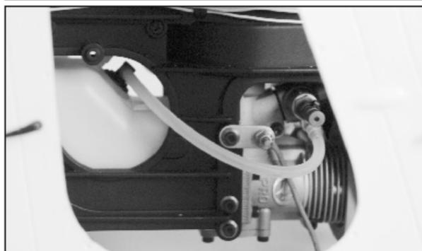
18. You will have to install the remote glow plug adaptor (TTR3803) for easy glow ignition. Also install a diverter and drill an exit hole at the bottom of the fuselage or you may extend the diverter to fuselage exhaust vent to obtain a more scale-like look.
