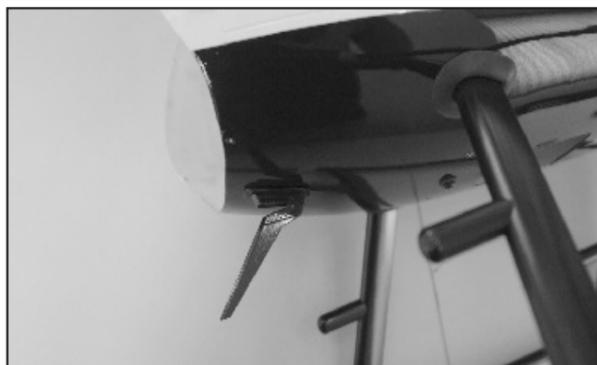
19. Install the wire strike on the front windshield. The big one is at the bottom and small one is on the top. Use 2x5mm wood screws to secure the strike in place.
