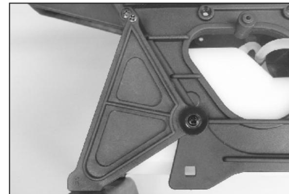
2. Put the scale fuselage aside for a moment and get your heli prepared. For Raptor owners, please remove the Landing Skid, Tail Fins, Boom Supports and Tail Rotor Assembly. Locate the Extended Rear Frames, which are specially designed for this MD fuselage. Secure the Extended Rear Frame in place with the screws and washers. (3x18mm self tapping screw for the top; 3x10mm washer self-tapping screw and big flat washer for the bottom).
