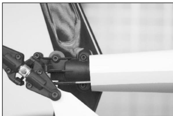
16. Secure the Vertical Fin in place with two 3x40mm Socket Screws, two M3 Washers and two M3 Locknuts.
