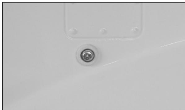
15. Secure the fuselage with 3x10mm washer self-tapping screw as shown.
