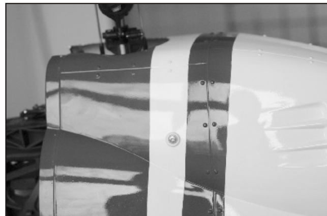
12. Drill the hole on the molded dot. Next enlarge the hole at about 8mm in diameter. Insert the silicon grommet in the hole.
