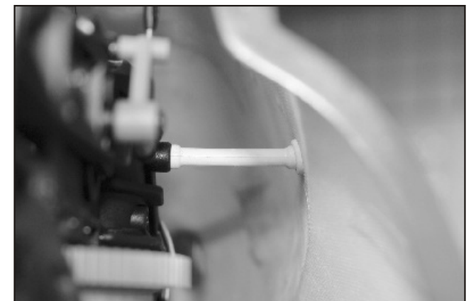
18. Secure the fuselage with 3x10mm washer self-tapping screw.
