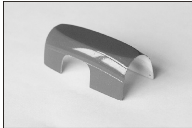
23. Trim the FRP case cover as shown to avoid any contact with the transmission case.
