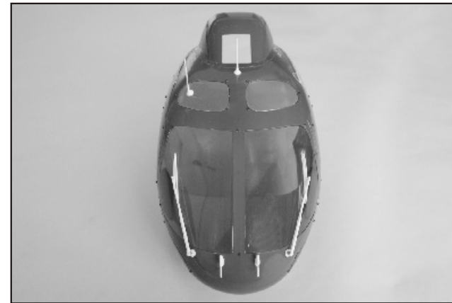
27. Install the fittings as shown includes wiper, pitot tube, antenna. Drill 2mm hole and use the retaining collar to hold the fitting in place. After adjusting the fitting properly, apply tiny CA on the collar to prevent it loosed. For wiper, secure the strut on the wiper mount with 2x6mm screw and M2 nut. Apply Loctite on the screw to prevent it from loose.
