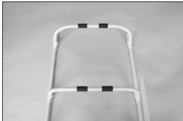
9. Apply foam tape at the mounting area of the landing skid.
