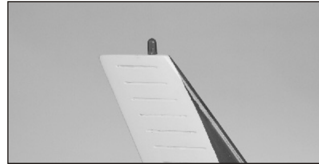
25. Cut the LED legs and glue the LED on the Fin for scale look.
