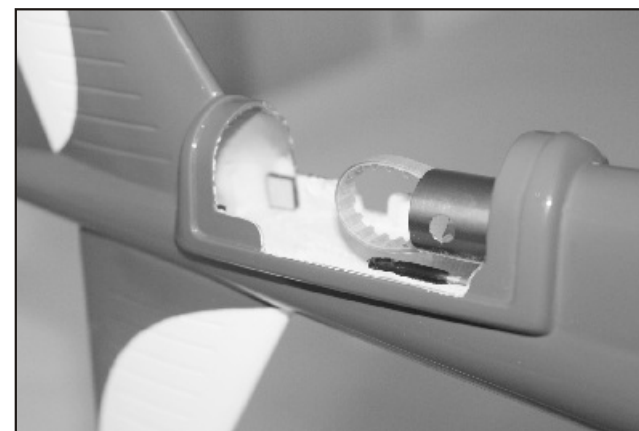
15. Place the Raptor into the fuselage, the post should be located near a molded dot on fuselage. Insert the tail boom into the fuselage and the skid adaptors sit in place, make sure the sponge is tightly fit in the tail and secure the tail boom firmly. Check the pushrod movement is freely without binding and adjust it if necessary. It is not necessary to glue sponge in the fuselage in case you had to remove the heli from fuselage.
