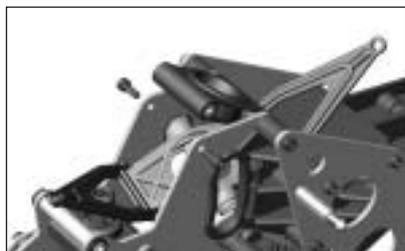
When installing the elevator control arm subassembly, temporarily remove the two screws that hold the rear of the upper BRG subassembly in place and move it up out of the way.
