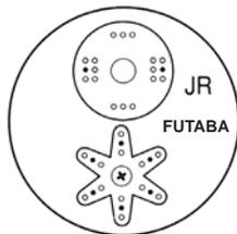
Mount the Steel Linkage Balls at 10.5mm(approx 7/16") from the center of the servo horn.
