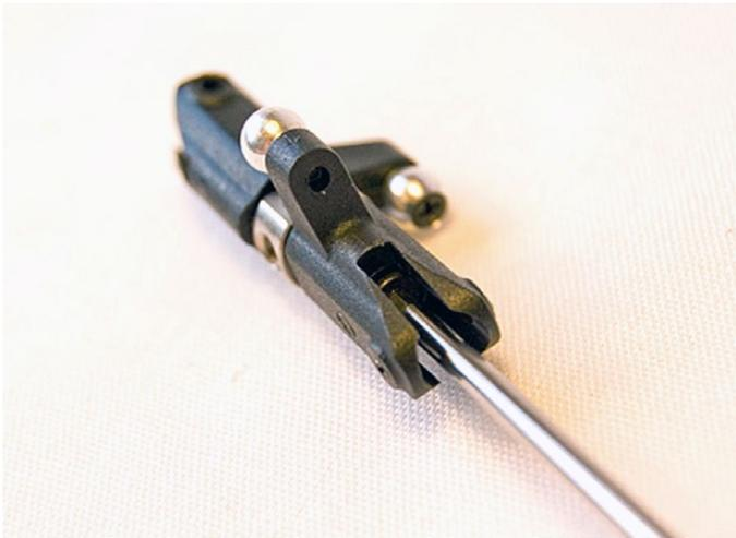
Fix both Tail Blade Holders (INT-073) onto the Tail Housing (INT-074) with a Cap Screw (INT-072).
