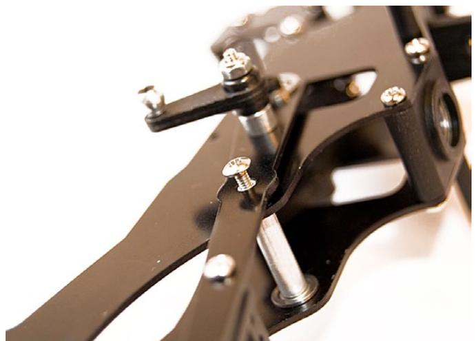
Place the Collective Pitch Lever and fix through the central hole with a Pan head Screw (INT-012) be careful with the threadlock.
