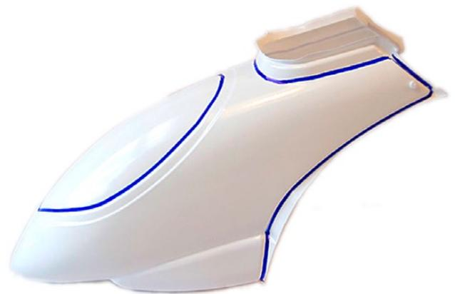
The Canopy (INT-094) needs the window area cut out and the flashing trimmed. The lines to follow are marked above.
