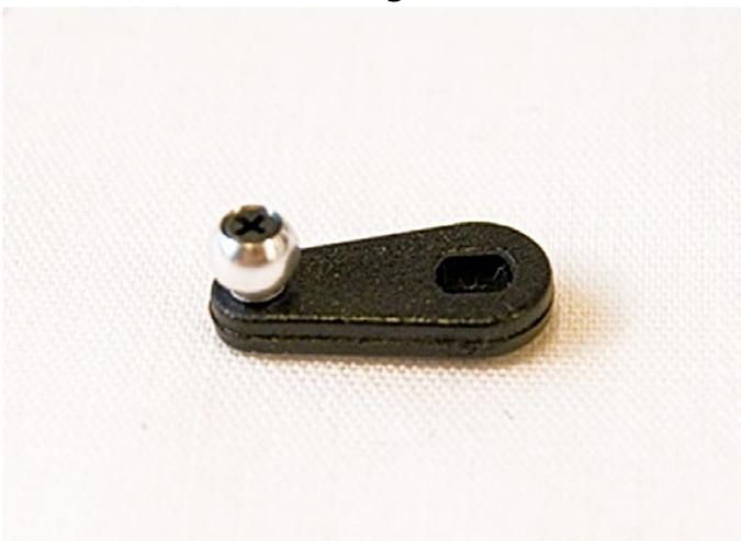
Elevator Torque Lever (INT-054) also needs the ball links (INT-001 + INT-002) installed.
