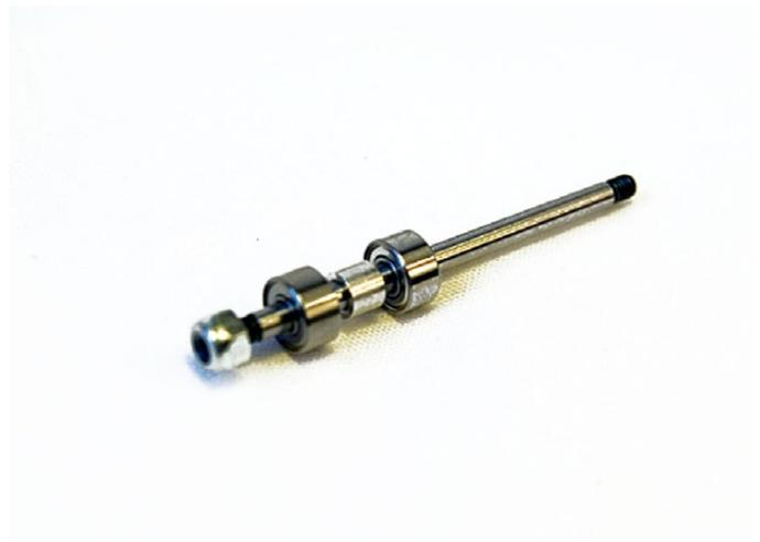
The M3 Nylon Nut (INT-007) followed by the Bearing (INT-005), Bearing Collar (INT-006) & the last Bearing. These are put on the Feathering Spindle (INT-010).
