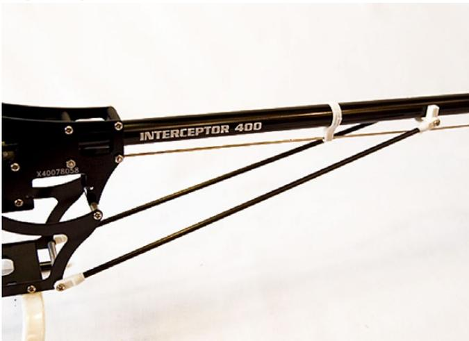
Affix ends of Tail Boom Brace Sets (apply a CA Glue) and screw into stabilizer holder with smaller screws before it sets.
