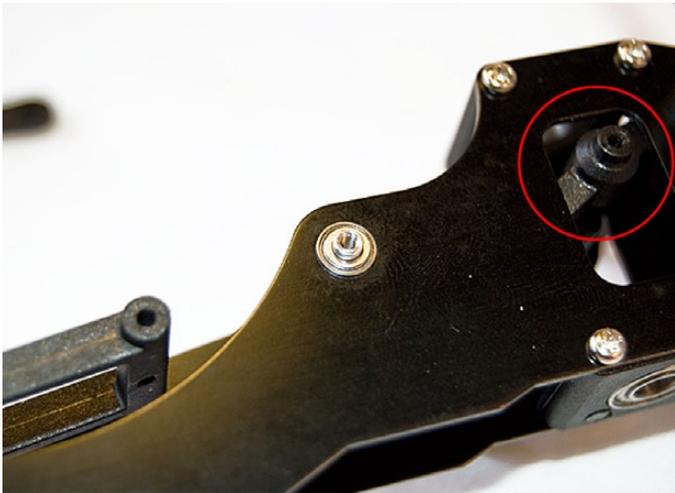
This is to be inserted into the frame and fixed through the Collective Pitch Lever (INT-057).
