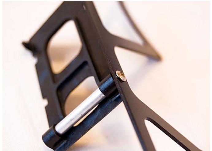
Affix the Lower Frame Set (INT-065) to the the Cross Member on both sides using a Pan Head Screw (INT-012) thread lock is advised.
