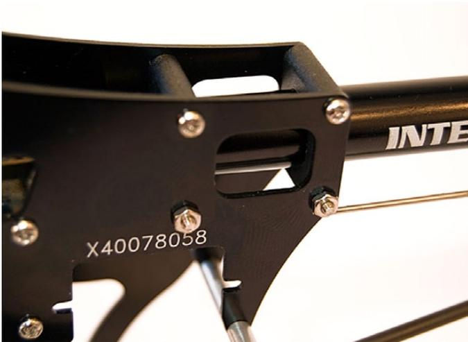
Once the belt is correctly looped over the pulley (see diagram) pull the boom and holder back into place and refix - tightening fully. This will ensure correct tension.
