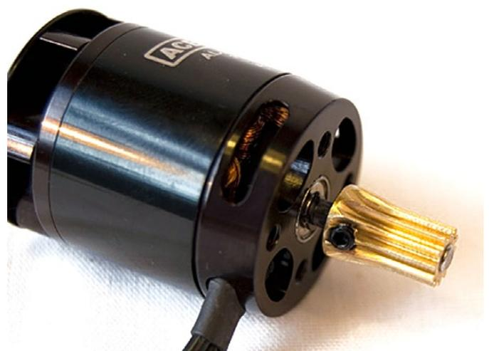
Install the pinion - we recommend a 12T for an all round performance. Use threadlock on the grub screw.
