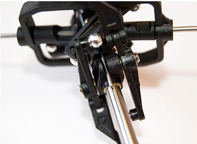
Slide Washout Control Set onto the Main Mast and align with pins - please note the direction the washout is inserted.
