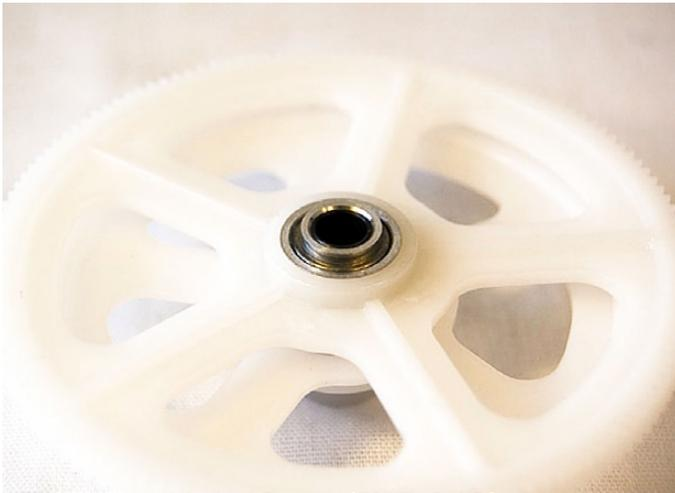
Take the Main Gear (INT-040) you have assembled and check that the collar is on top.
