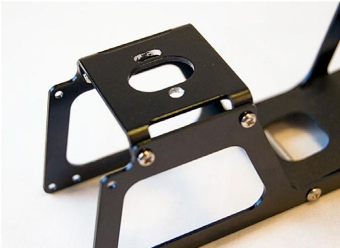
Fit the Motor Mount (INT-061) with Pan Head Screw (INT-067) and M2 Nut (INT-044) with thread lock.
