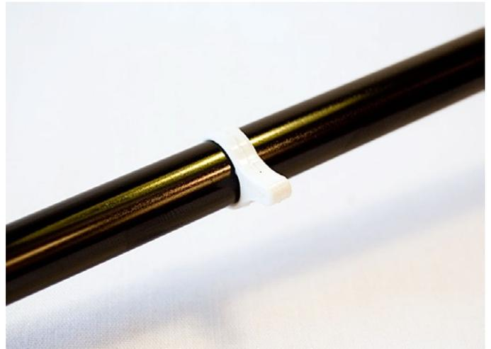
Slide the rudder push rod support onto the boom.
