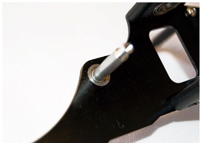
Place elevator shaft (INT-051) into holder on frame.
