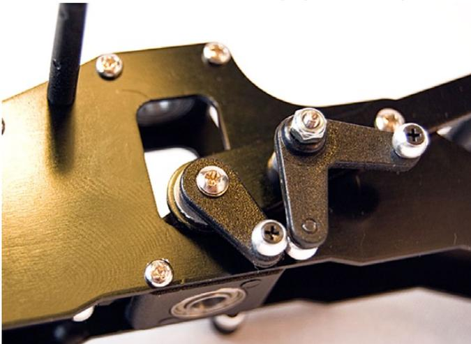
Fix the Elevator Torque Lever (INT-054) to the Elevator Arm (INT-048) with Washer (INT-032) and Pan Head Screw (INT-012). Place washer between lever and screw
