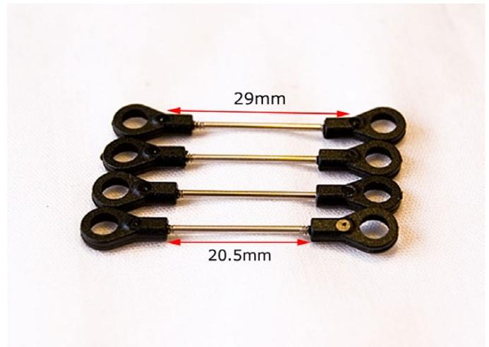
Put together four Elevator Swash Rods (INT-090) with a link to link measurement of 20.5mm. They all attach from the lower Swash Plate Set (INT-023) to...
