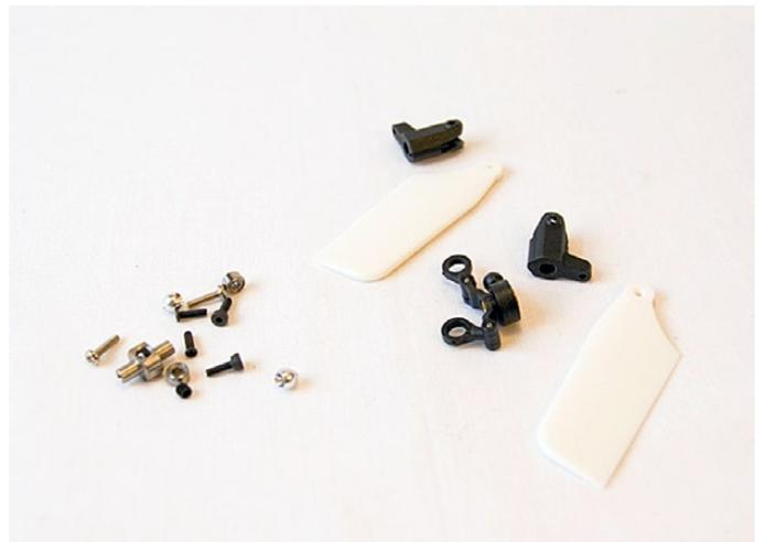
Start the tail by assembling the rotor holders.
