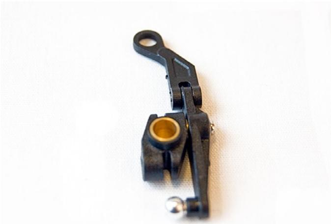
Screw Washout Control Arm (INT-029) into place on Slide Block (INT-031). Please ensure screw is aligned correctly. DO NOT OVERTIGHTEN.
