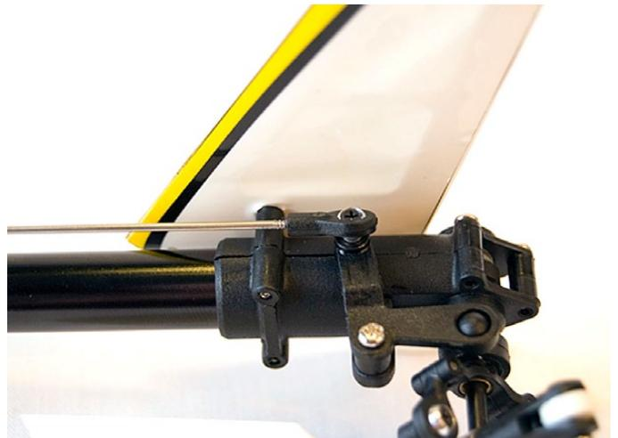
Screw ball link onto end of Rudder Push Rod (INT-085) and clip onto Tail Pitch Lever (INT-077).
