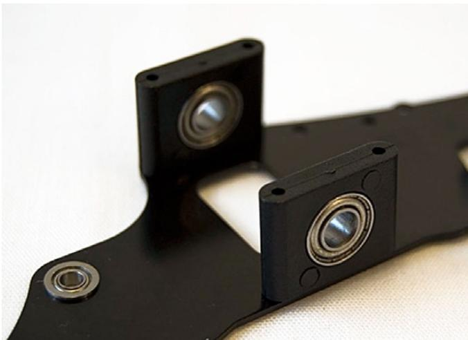
Affix both bearing holders in place with self tapping screws.
