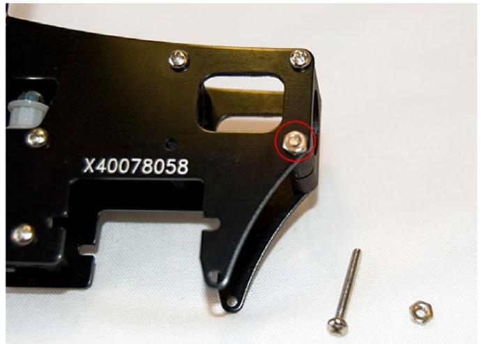
Fix the sides of the frame together - work from the back. Using the Pan Head Bolt (INT-053) and M2 Nut (INT-044) - don't tighten.
