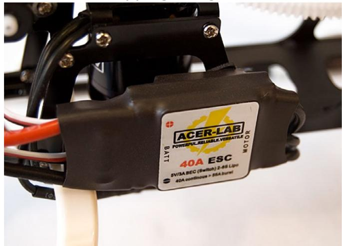
Mount the ESC as above - we advise not to use cable ties as this can cause overheating and malfunction. Using cable ties on many ESC's voids the warranty.
