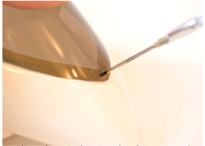
Align the window on the Canopy and pierce both. Fix with the four window screws.
