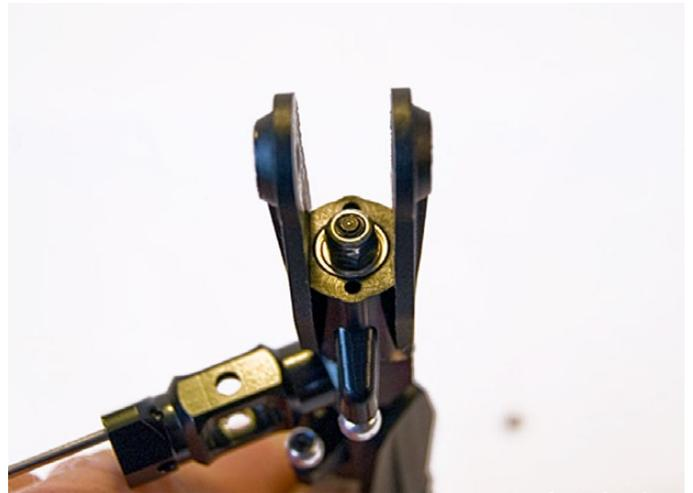
Screw two 3mm screws into each Blade Holder.
