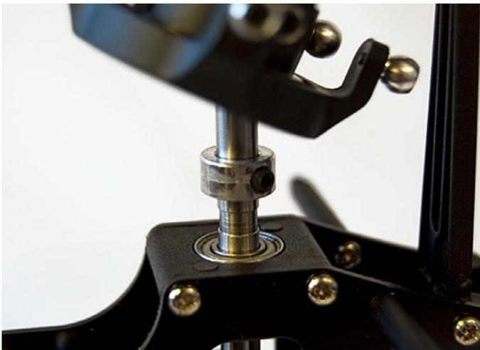
Loosen the Mast Lock (INT-027).
