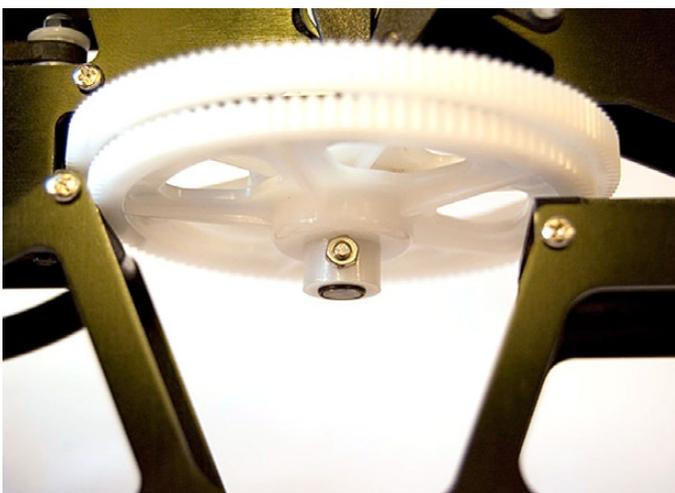
Insert Pan Head Screw (INT-025) and secure with M2 Nut (INT-044) - do not overtighten or you may damage the Main Gear.
