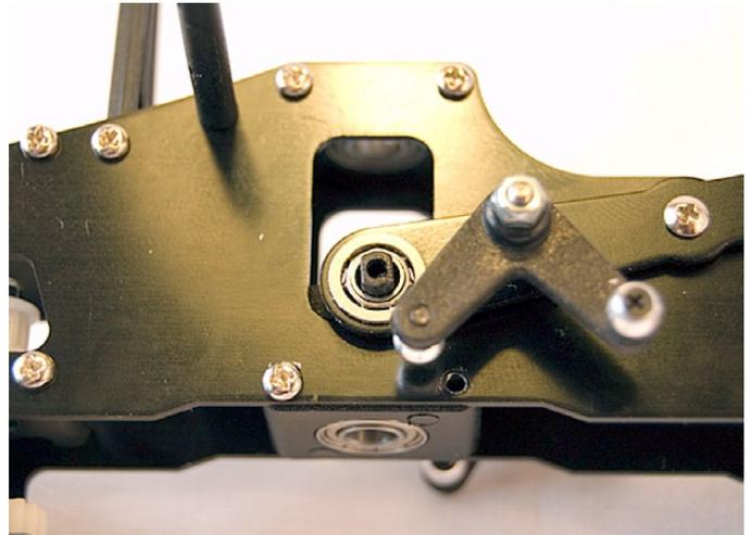
Push the Elevator Lever into the fixed Collective Pitch Lever. The longer part should extrude past the lever.
