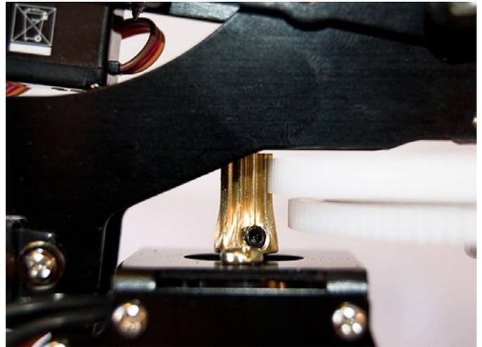
Adjust pinion and gear mesh - too tight will cause the ESC to burn out and overload your batteries. Too loose will risk stripping the gear.
