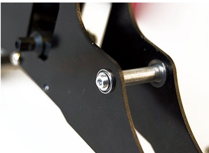
Place the washers over the end of the Elevator Shaft (INT-051).
