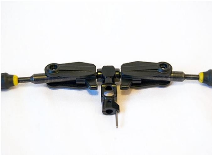
Tighten with two 5.5mm socket wrenches.
