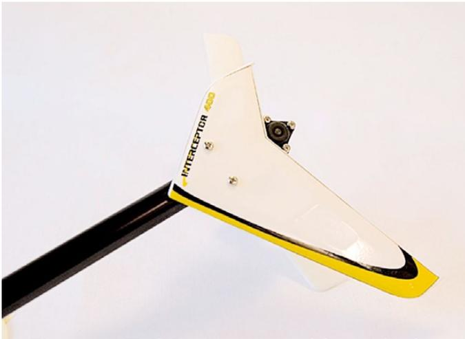
Fix onto Tail Rotor assembly with the screws.
