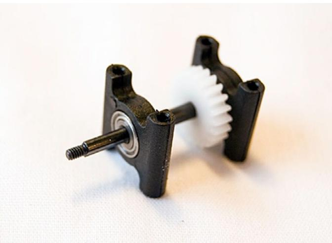
Push the second Counter Gear Case (INT-035) onto Counter Shaft (INT-036).
