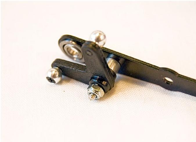
Install the assembled Aileron Levers and secure with an M2 Nylon Nut (INT-024). Do not overtighten.
