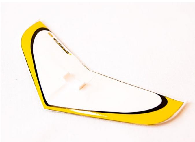
Cut out decal and fit to horizontal stabilizer - take time on lower one as it can be a tricky fit around the boom rest.
