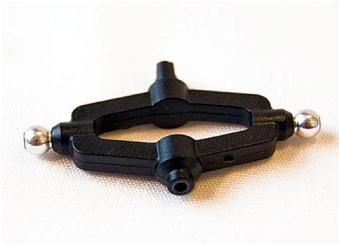
Screw ball links (INT-001 + INT-002) into the elevator arm (INT-048)
