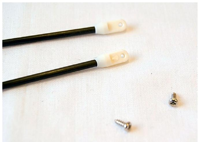
Put one end on to each of the Tail Boom Brace rods. Use a little CA Glue.
