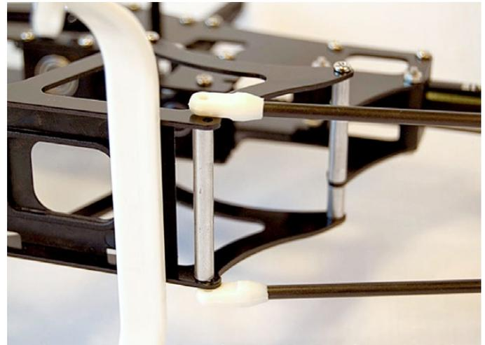
Place Cross Member M2x34 (INT-063) and screw into place the Tail Boom Braces (INT-084). Use thread lock to hold the screw securely.
