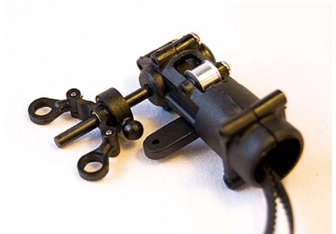
Slide Tail Pitch Set (INT-076) onto Tail Shaft (INT-079) - note direction of fitting.
