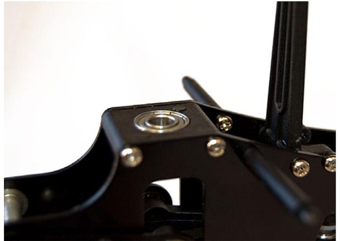
Place bearing holders so that the bearing faces upward and the recess is downward (applies for both upper and lower).
