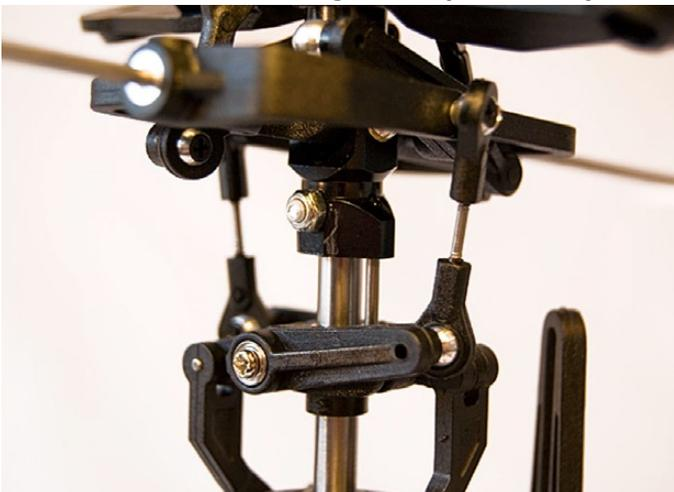
The Stabilizer Control Rods (INT-088) go from the Stabilizer Control Set (INT-018) to the Wash-out Control Arm (INT-029).
