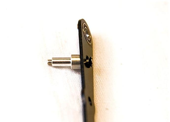
Take one Collective Pitch Lever (INT-057) and push one Flush Head Screw (INT-056) through and into an Elevator Mount (INT-055). Like above.
