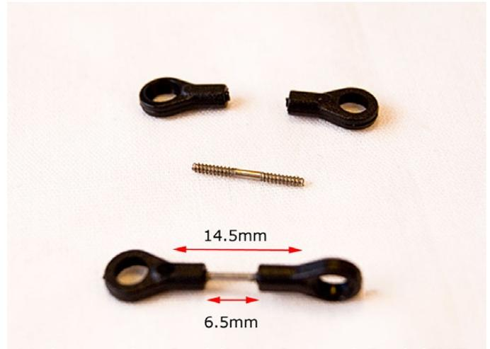
Make up the Stabilizer Control Rod (INT-088) it should be 6.5mm from link to link.
