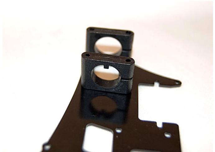
Position forward boom holder - note position of notch on the left side of the frame.
