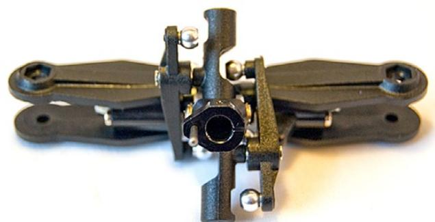
Screw both Mixing Arms (INT-017) onto the Seesaw (INT-016) through a Bearing Spacer (INT-013) and two Bearings (INT-014) with a Pan Head Screw (INT-015).
