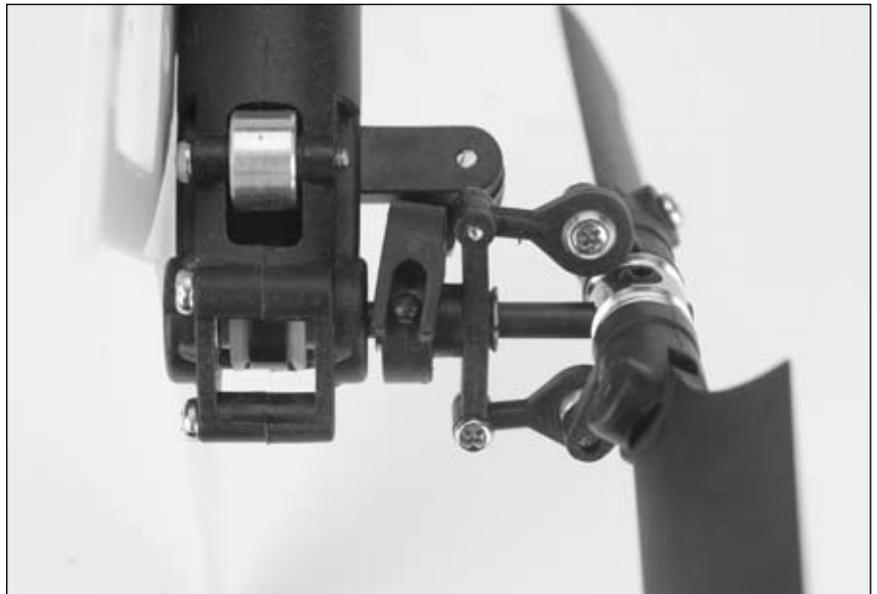
If you find that the tail servo is responding opposite to rudder control inputs, simply reverse the rudder channel in your transmitter.
