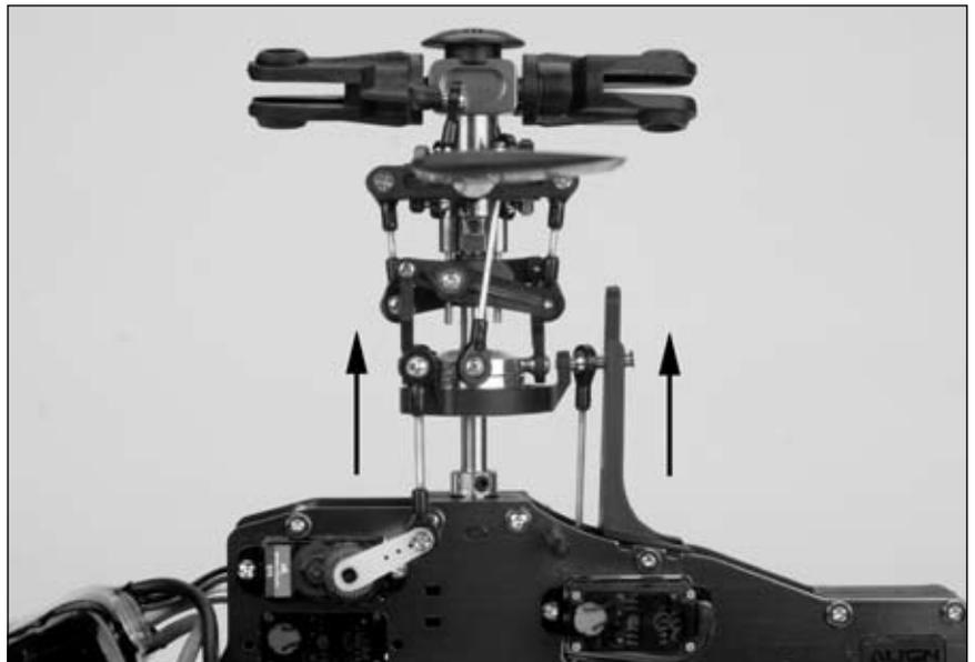
With the stick pulled back down, the swashplate should lower, decreasing the pitch of the main blades.
