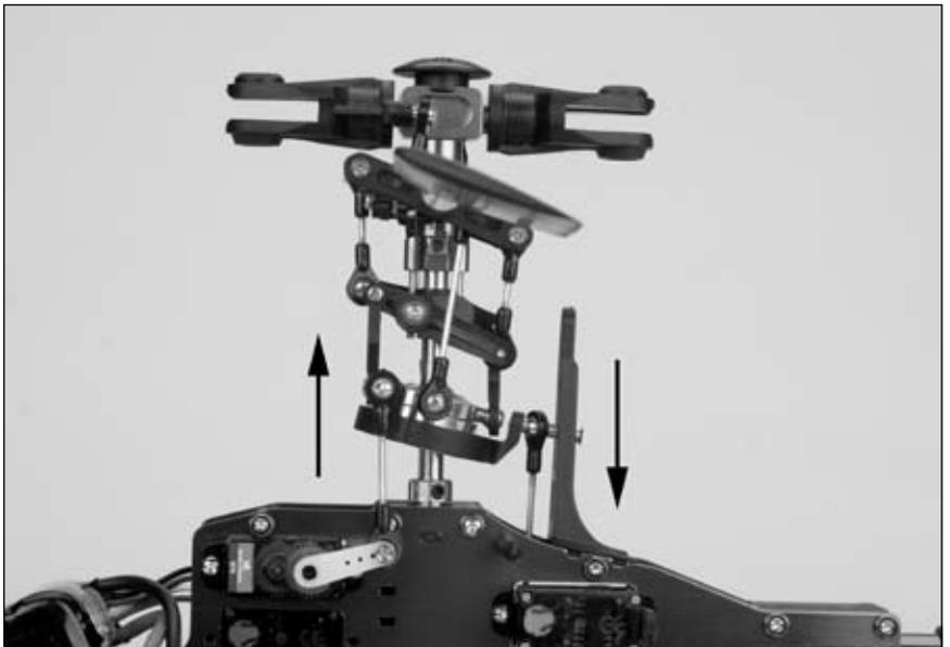
Viewing the helicopter from the rear (tail boom toward you), move the right-hand stick left and right to check aileron roll control. When the stick is pushed to the left, the swashplate should also tilt left.
