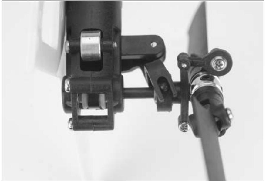
With the stick pushed to the right, the tail pitch slider should move to the left, toward the tail case.
