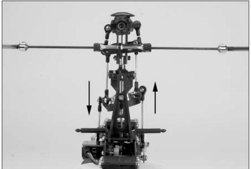
With the stick pushed right, the swashplate should tilt to the right.
