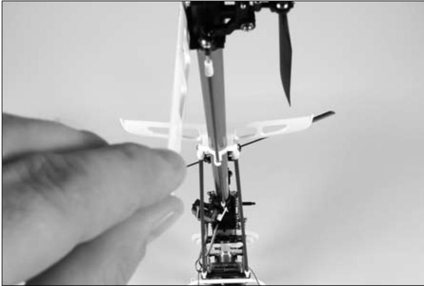
Then, adjust the servo and tail boom servo mounts (by sliding them fore or aft on the boom) until the tail pitch slider is centered on the tail rotor shaft. When the slider is centered, the ends of the brass bushing should be at equal distances from the tail rotor case and tail rotor hub.
