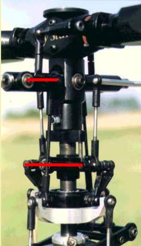
Fig. 5: MyStar 60 Rotor head basic setting: Blades on 0 degree, washout arms and seesaw mixing arms horizontal.
