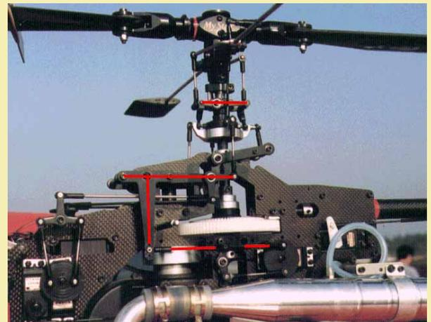
by the MS46 washout unit (413-6600 wash-out assembly) including the guide pin (513-5670) below the rotor head. This combination is only possible with the modified shorter pitch arm.
