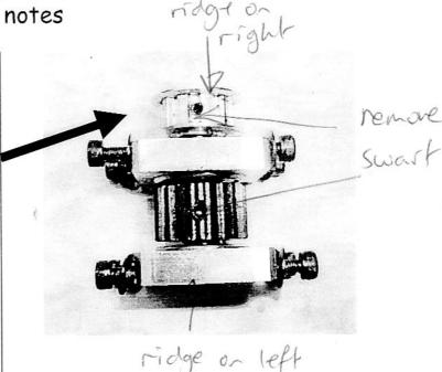
Fit the tail shaft pulley in the orientation shown. Look at the grub screw hole.
