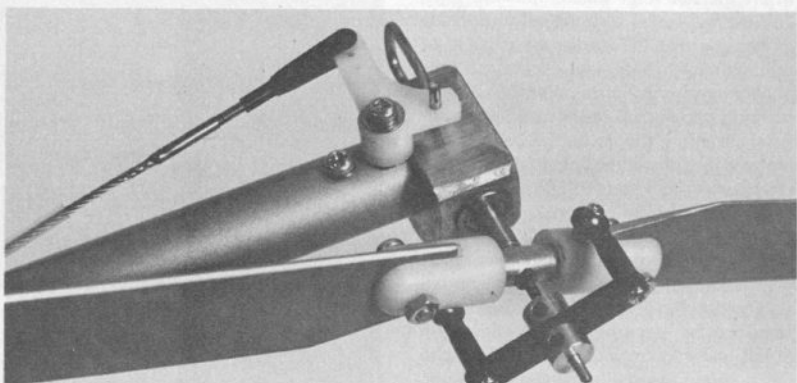
The tail rotor gear box, blade holders, collective pitch linkage, and blades are installed on the tail boom.
