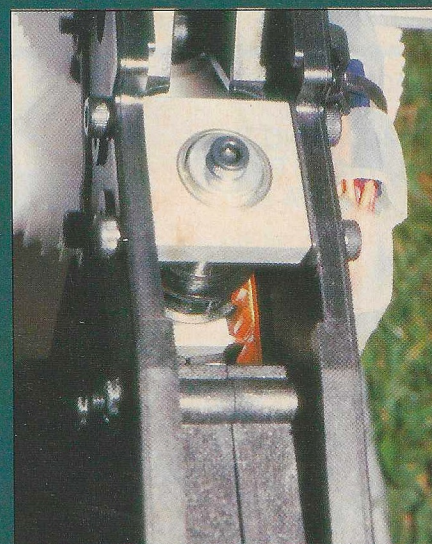
Tail drive, note the aluminium bearing blocks.
