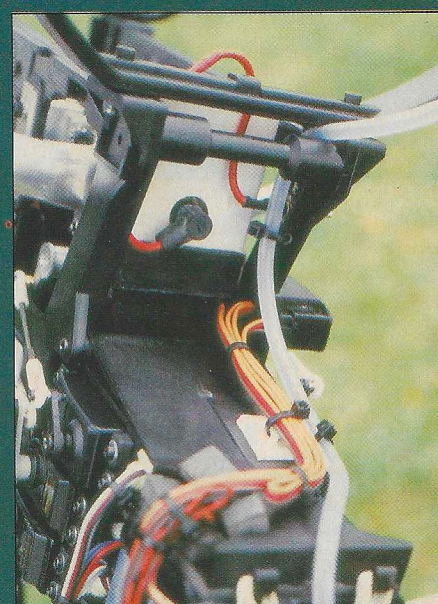
Cooling duct has been extended using plasticard - helps to keep things clean and cooler.
