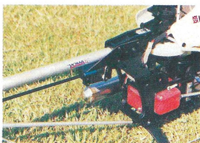
Dubro 2 oz header tank strapped to the radio tray provides totally consistent running.
