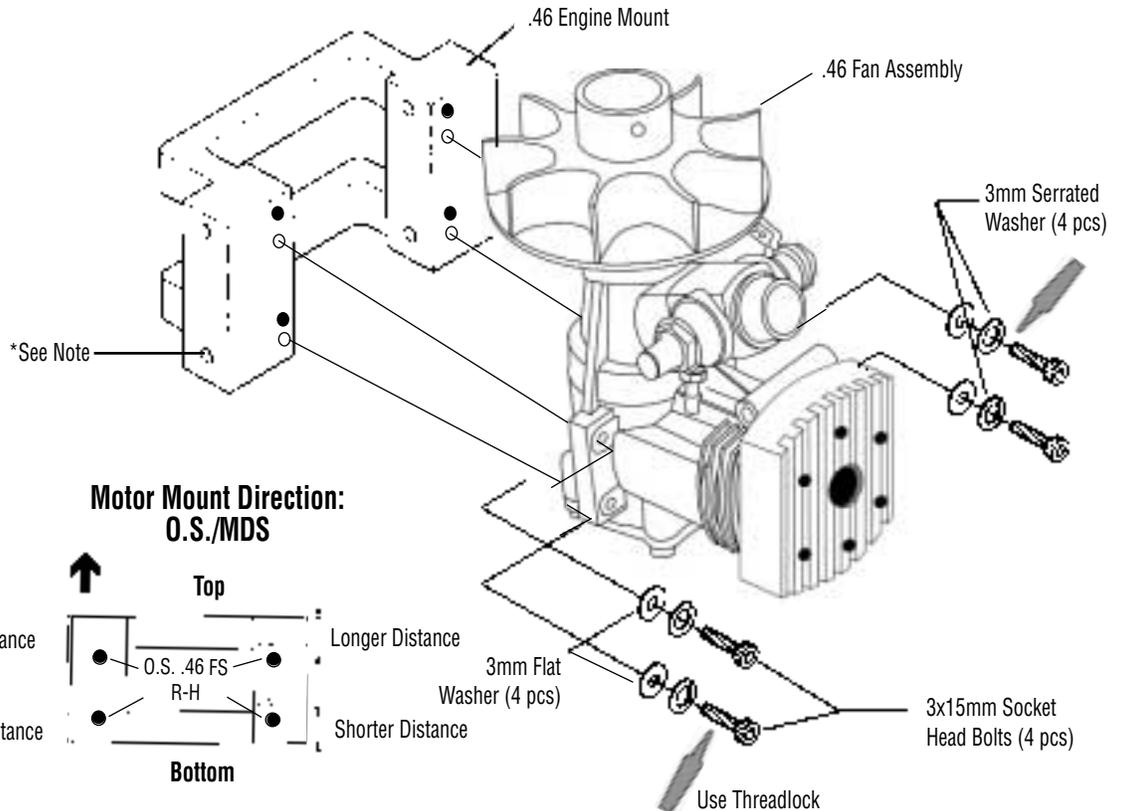
It is important to note the proper direction that the Motor Mount is installed to achieve the correct alignment of the engine.
