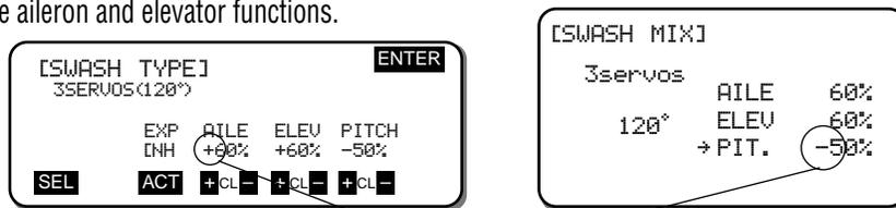
To reverse the direction of a CCPM control function it's necessary to change the value from + to -, or - to + as needed.
