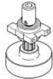
**Note:** Be sure to allow a slight amount of clearance between the Start Hex Adaptor and the Bearing Block to prevent binding.
