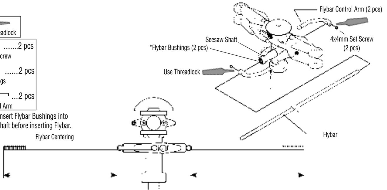
**Note:** Center the Flybar in the Seesaw Shaft before securing the two Flybar Control Arms.
