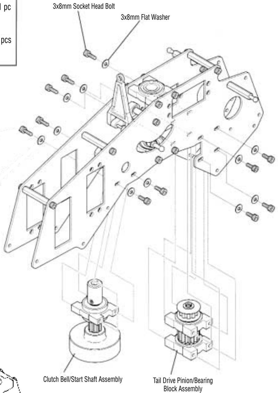
**Note:** Both the Clutch Bell/Start Shaft Assembly (Step 1-1) and the Tail Drive Pinion/Bearing Block Assembly (Step 1-2) are temporarily installed at this time. These assemblies will be adjusted and secured in Step 3-2.
