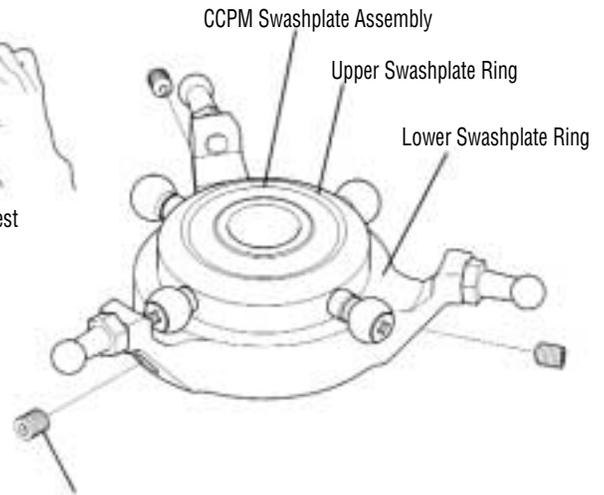
4x4mm Swashplate Adjusting Screws
