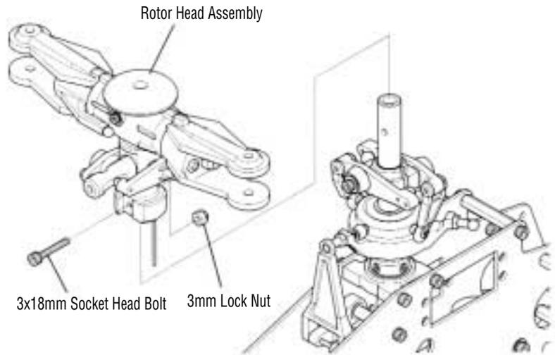
**Note:** Be sure to engage the rotor hub pin into the washout base groove before securing the rotor head in place
