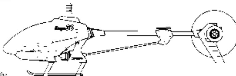
**Caution:** Be sure to maintain a safe distance from the helicopter (15 to 20 feet) when tracking main rotor blades.
