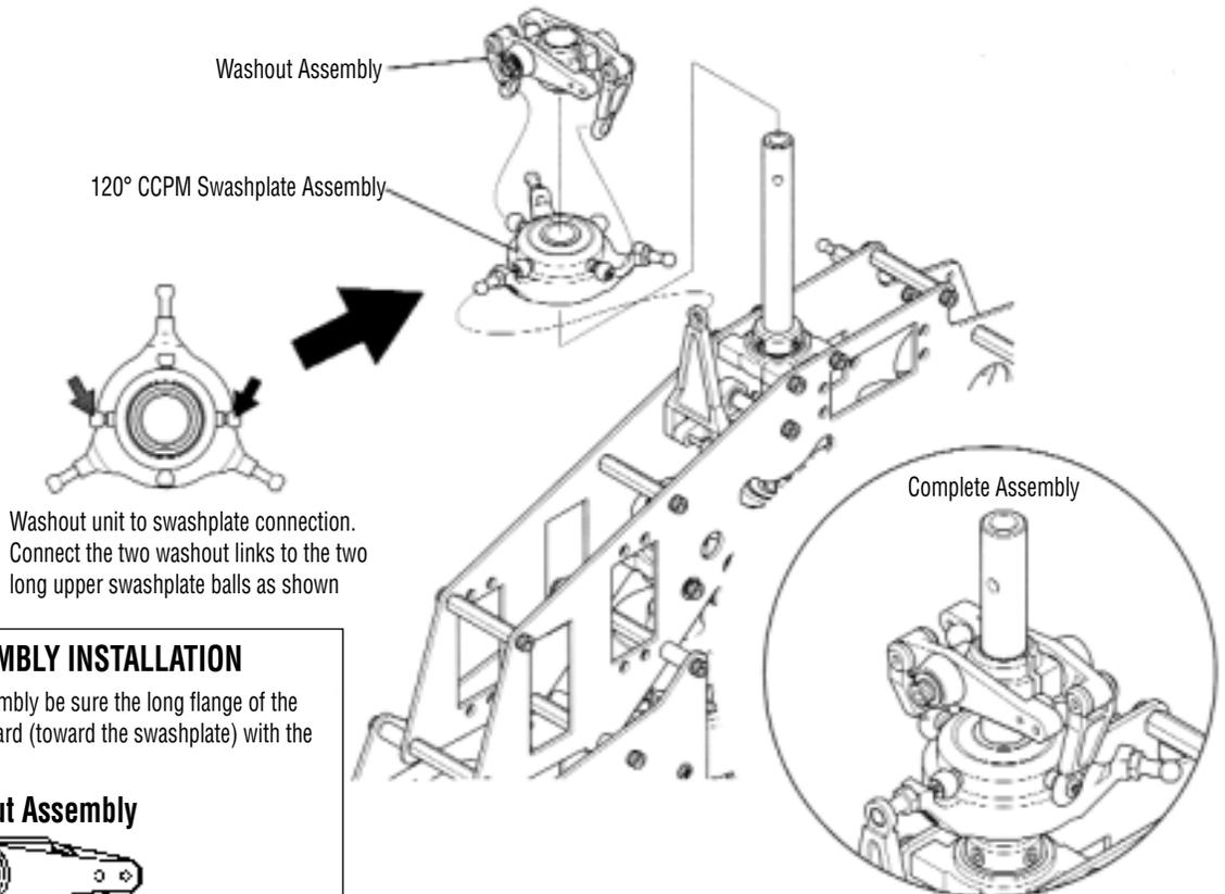
Washout unit to swashplate connection. Connect the two washout links to the two long upper swashplate balls as shown
