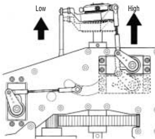
View is shown from the left side of the model. Notice how in this example the swashplate has tilted forward as the collective has moved from the center to the full high pitch position.
