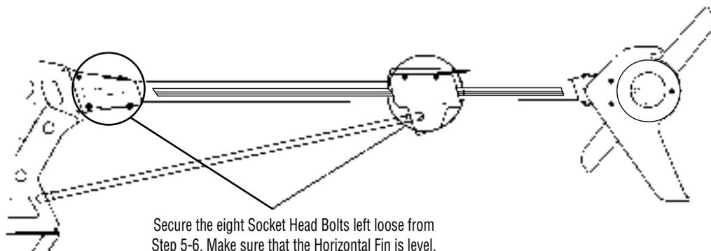
Secure the eight Socket Head Bolts left loose from Step 5-6. Make sure that the Horizontal Fin is level.
