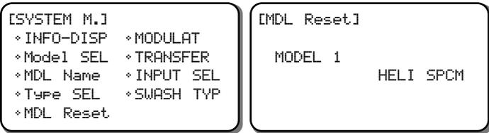
B) Press the UP or DOWN keys to move the cursor to the SWASH TYPE Function, then press the UP and DOWN keys simultaneously to access the Swashplate Type Function.
