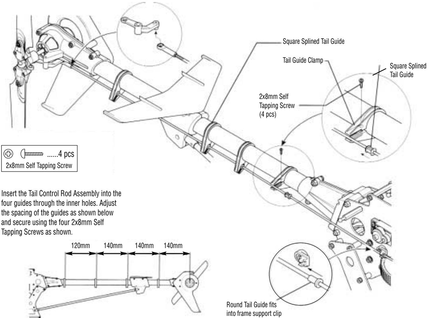
Insert the Tail Control Rod Assembly into the four guides through the inner holes. Adjust the spacing of the guides as shown below and secure using the four 2x8mm Self Tapping Screws as shown.
