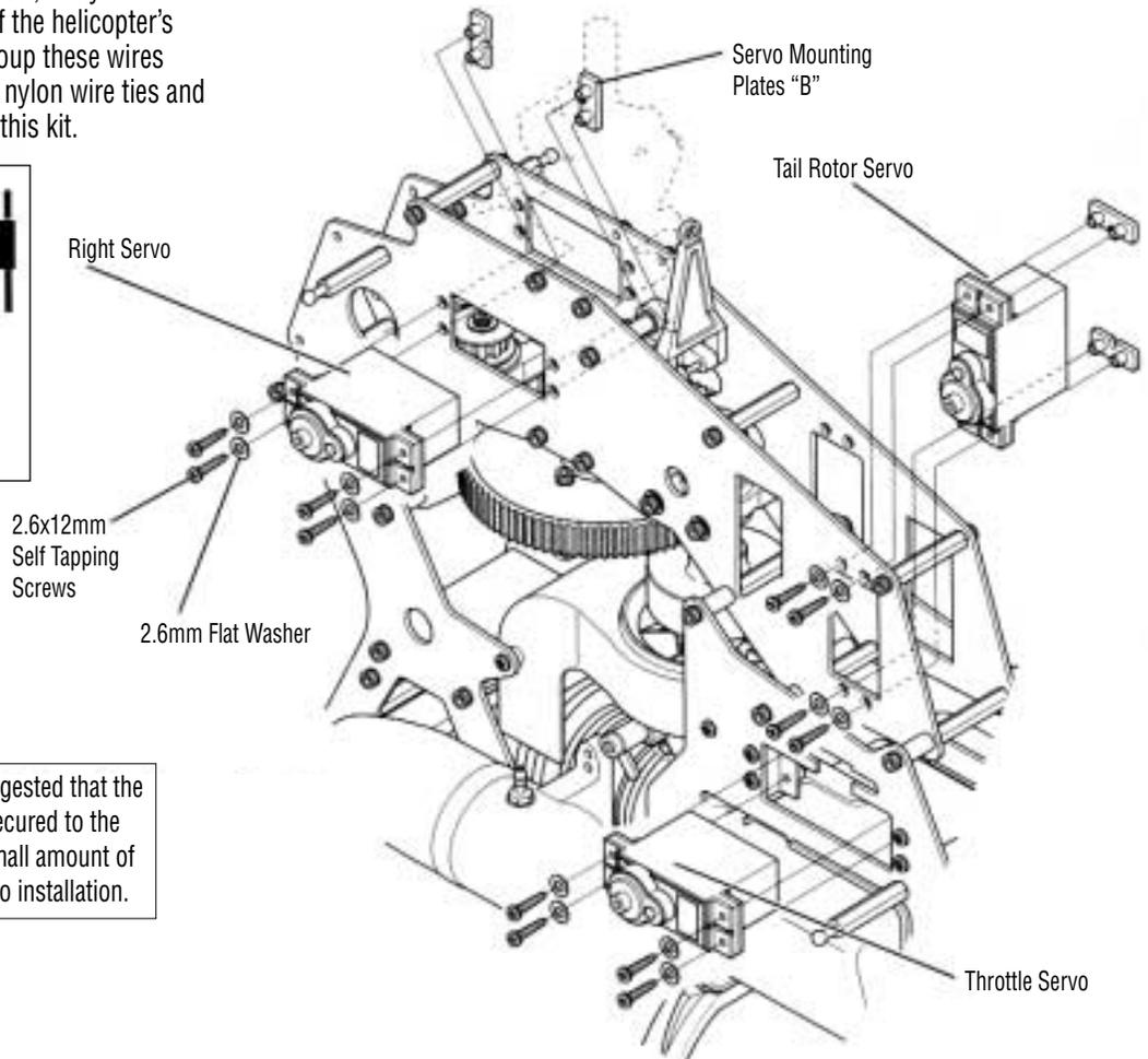
Note: Before installing servos, it's suggested that the servo mounting plates "B" be secured to the inside frame position using a small amount of CA adhesive. This will ease servo installation.
