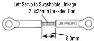
**Option:** For smooth operation, pre-size the ball links with the JR Ball Link Sizing Tool prior to attachment.
