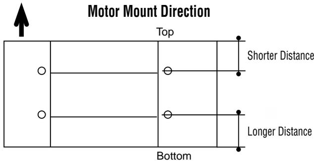
It is important to note the proper direction for the motor mount installation for achieving the correct alignment of the engine.
