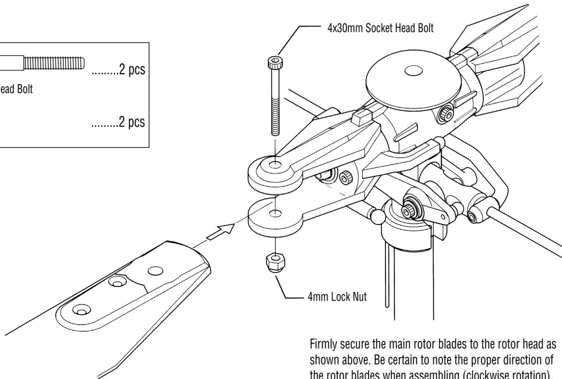
Firmly secure the main rotor blades to the rotor head as shown above. Be certain to note the proper direction of the rotor blades when assembling (clockwise rotation). Main blades should be tightened so they can pivot when moderate pressure is applied. Do not allow the main blades to swing freely within the main blade holders.
