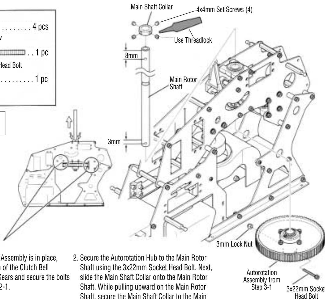
1. Once the Main Shaft Assembly is in place, adjust the gear mesh of the Clutch Bell and Tail Belt Pinion Gears and secure the bolts left loose from Step 2-1.
