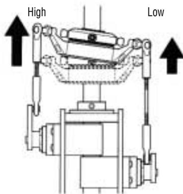
In this condition, we would suggest that the travel value for the Left servo be reduced slightly (5–10%). Repeat the procedure above. If the same condition occurs, but to a lesser degree, then the travel value of the Right servo should be increased slightly and retest. In most cases, it will require only the adjustment of the Left or Right servo to correct this situation.
