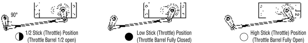
\*To avoid differential throttle travel, make certain both the throttle arm and the servo horn are positioned as shown in the above diagrams.
