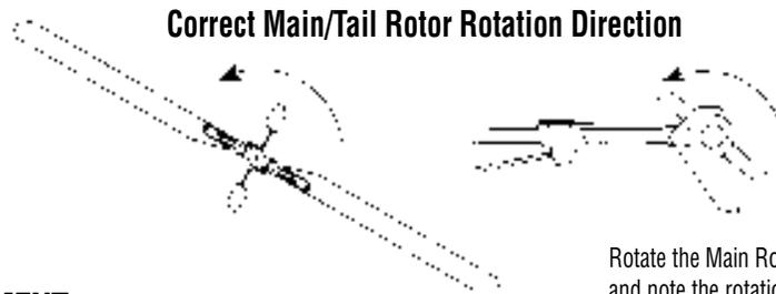
Rotate the Main Rotor counterclockwise (backward) and note the rotation of the Tail Rotor.
