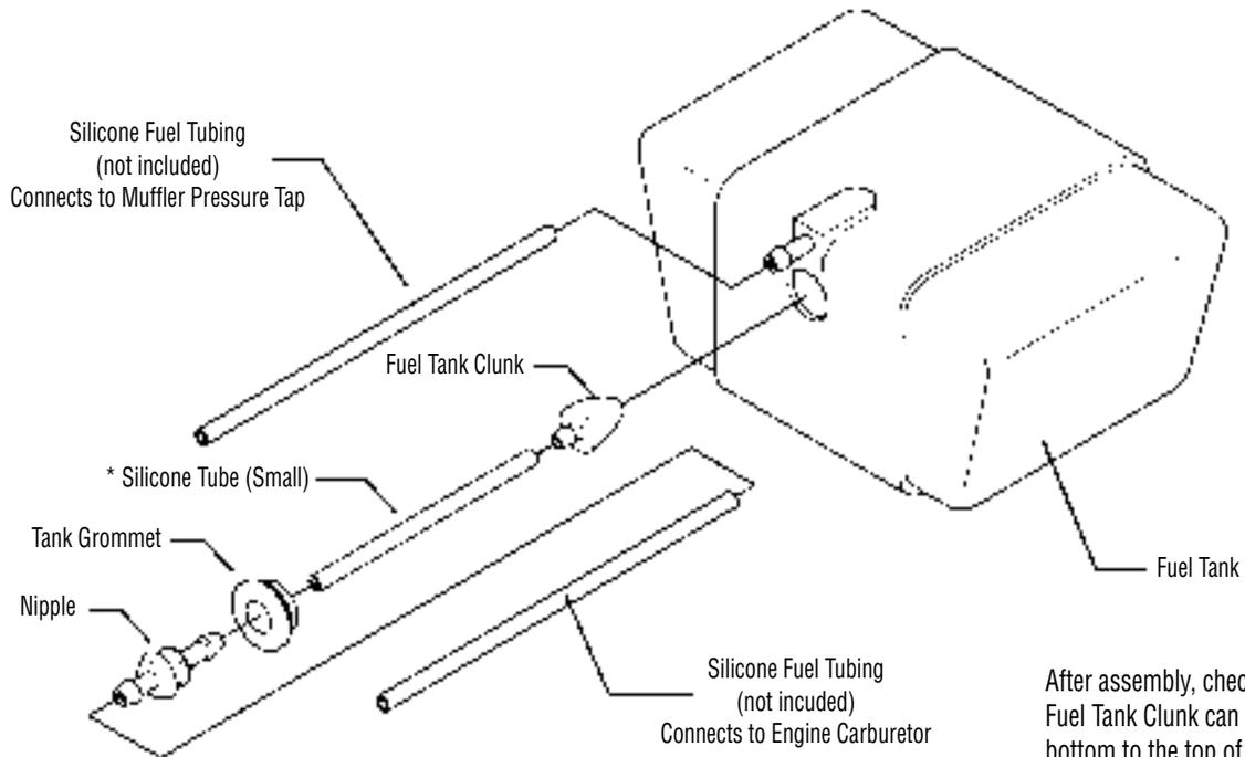
After assembly, check to be sure the Fuel Tank Clunk can move from the bottom to the top of the tank without touching the back wall of the Fuel Tank.
