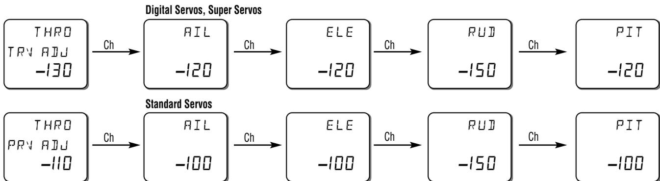
**Note:** The travel values shown for the rudder function are for use with Piezo gyros, like the JR NEJ-900, NEJ-400, NEJ-450, or NEJ-3000 type gyros. If a conventional mechanical type gyro is used (JR 120, 130, etc.), then the travel values of the rudder will need to be reduced to approximately 100%.
