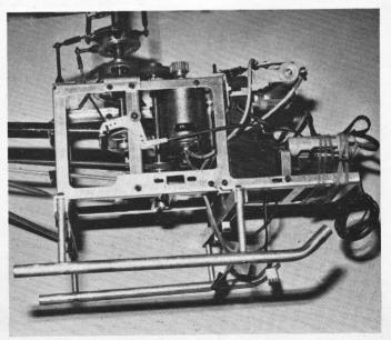
two motors at maximum power. Before continuing further, for the benefit of those readers who have not actually seen this model, a few measurements etc. may be of interest. Rotor diameter is 992mm, overall length 846mm, weight (fully loaded) 1.560g. Motors (2) RS 540S, Radio system 4-function lightweight. Note that the R/C system must be a reasonably up-to-date set using the smaller size servos. I fitted my Sanwa F.M. and the servos were only just small enough to suit the servo mounts.
