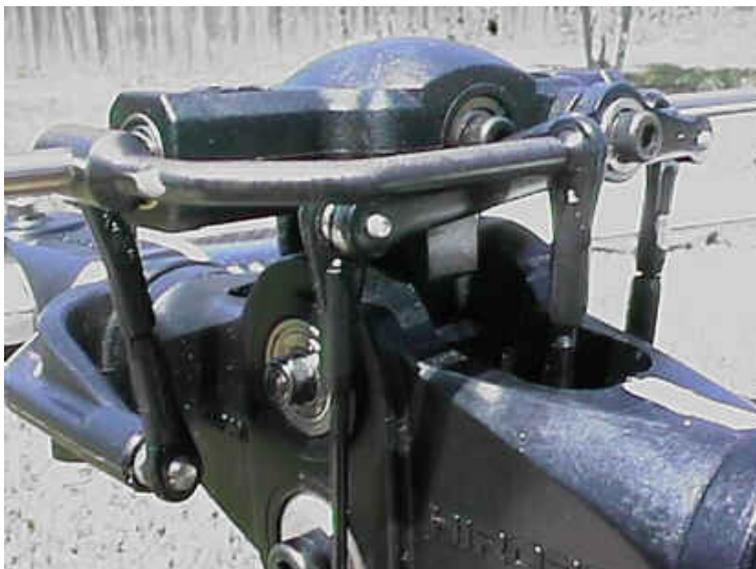
On an engineering note, the blade holders are attached to short stub axles that are molded into the yoke. They are virtually impossible to bend even after a really hard crash. Each of these axles provides  $0.5^\circ$  of positive coning angle. Funny, but the Tsurugi appears to be just as stable upside down as it is right side up. True!
