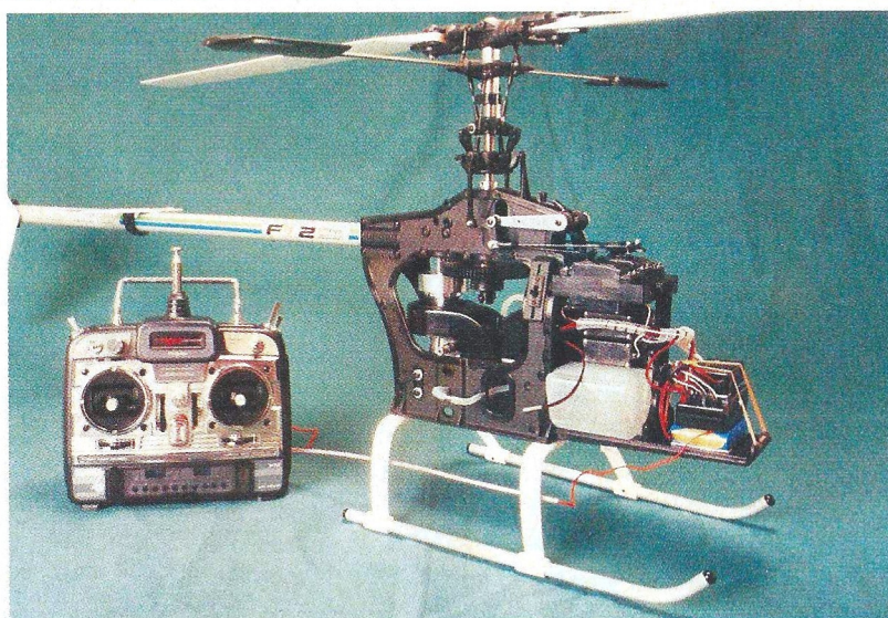
Radio installation is simple with excellent instructions in the manual. The transmitter pictured here is the Futaba Skysport 6H, a non-computer set providing the basics a beginner would need.
