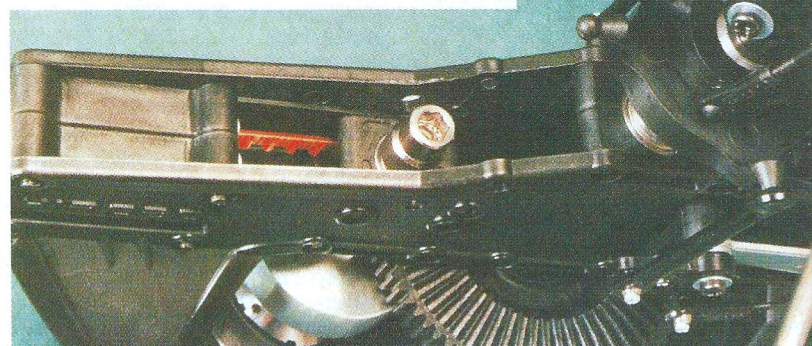
Final part of the top start system - the hex drive adapter which does away with the old belt start system making it easy to start and ideal for fuselage use.
