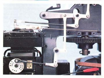
Above: Showing the new Shuttle from the port side, with the re-designed silencer. The changes in the collective pitch control mechanism, the lowered ball-joints on the roll servo output disc and the side-frame mounting points for the tail-boom braces may be noted. The individually mounted servos are also visible.
