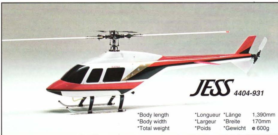
The design of this fuselage for sports helicopters has been based on the Jet Ranger model which is very popular among all modellers worldwide. This streamlined body in flexible epoxy material is ideal for aerobatic as well as static manoeuvres and can be fitted on every Hirobo .60 size mechanic. Easy access for maintenance due to the large removable top cover.
