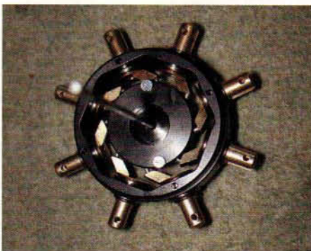
Fenestron hub is beautifully engineered and is factory assembled.
