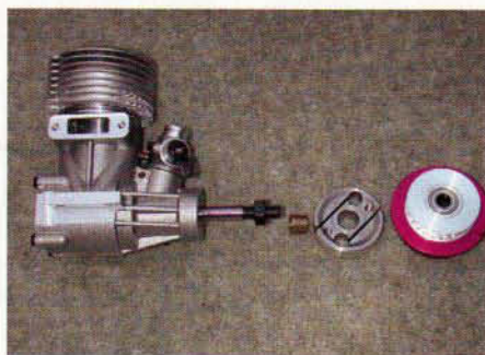
Motor and clutch - note the use of the 8 mm crankshaft on the Rossi 65.
