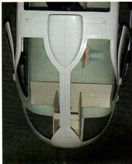
Front formers to reinforce the fuselage - note the hinged front doors.
