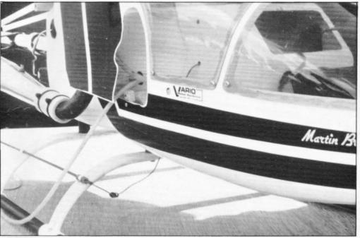
The removal of two small screws allow the canopy to split for removal without dismantling the exhaust system.
