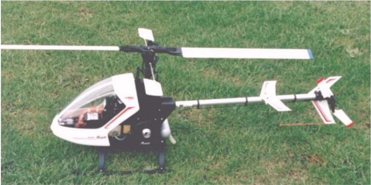
The original Robbe/Schluter 'Moskito' kit was supplied with both skids and a tricycle undercarriage, together with a plastic cabin/canopy unit with an integral dummy pilot. A notable feature was the possibility of building the machine for clockwise or anti-clockwise main rotor direction. This kit is still available as the 'Moskito Standard'.
