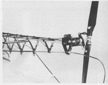
The tail boom and rear fuselage plate must be joined together over the plan in order to obtain the correct angle of 'up-sweep' of the boom. Too great an angle will result in. bent tail boom longerons when these are clamped to the rear plate and will also cause 'binding' of the tail rotor drive shaft
