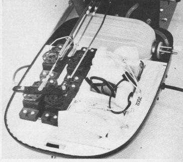
a necessary modification to avoid possible rearward movement of the rotor assembly in flight is to drill both sides of the clamp and insert self-tapping screws through into the plastic case of the assembly. The results of not carrying out this modification are detailed in the flight test.
